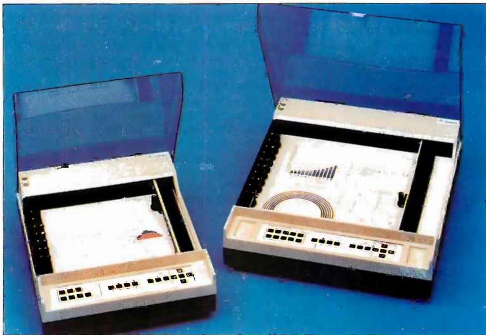
sets, including a scientific/Greek alphabet, are stored in ROM. Other features include variable line fonts; cross-hatching, bar, and pie chart capability; arc and circle generation; character rotation and slant; and
