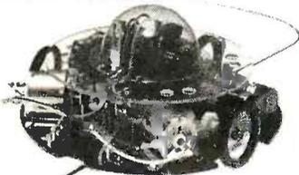
Uses an infra-red light sensor to automatically follow a black line (min. 10mm wide) drawn on white paperboard. (Minimum turn radius 15cm.) Uses 2 AA and 1 9V battery (not included).
