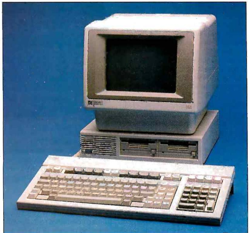
Photo 1: The HP 150 with a 9121 disk-drive unit.
