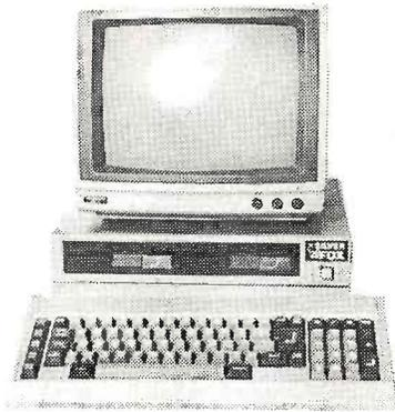
256K RAM/1.6 Megabytes on dual floppys Compatible with 160K, 320K, 360K formats Keyboard/12" monitor/Printer Port/8088 CPU One Year Warranty/Graphics/MS-DOS Wordstar/Mailmerge/Spellstar/RAM-Disk/Easy Writer/Dotstar/Reportstar/FILEBASE/Calcstar Color Graphics Basic plus 25 games, graphics, and more
