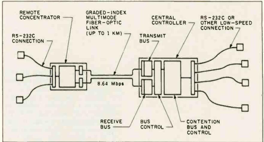
Figure 3: The fiber-optic connections in AT&T's 8.64-Mbps Information Systems Network serve as extensions of two metallic signal buses inside the central controller.
