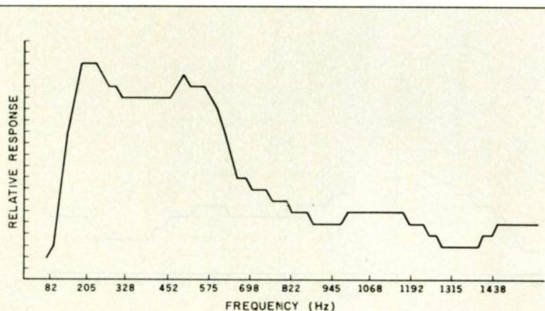
Figure 11: Frequency response with all controls even.
