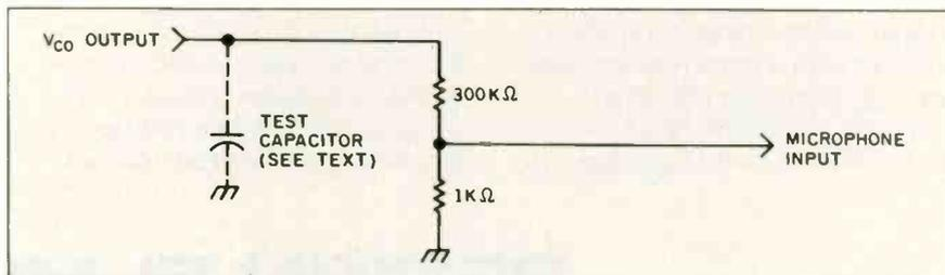
Figure 9: Input section calibrate and test setup.
