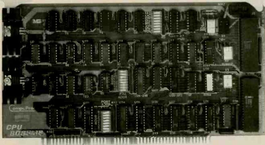
Gifford Computer Systems' MP/M 8-16 computer uses the CompuPro Dual Processor 8085/8088 board to run both CP/M-80 and CP/M-86.
