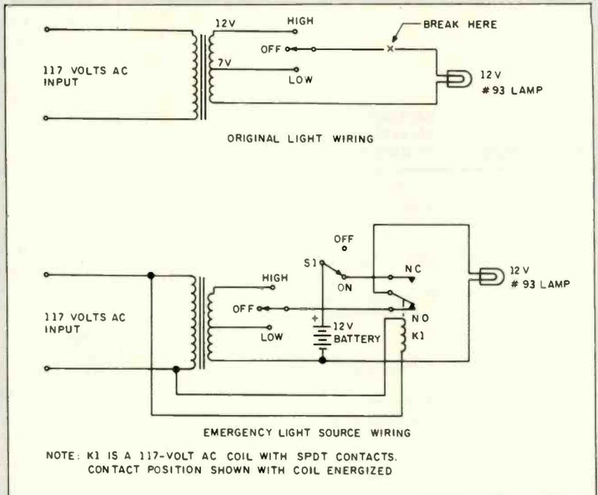
Figure A: This emergency lighting setup powered by a UPS can keep you from computing in the dark. (Original schematic by Barbara Campo.)
