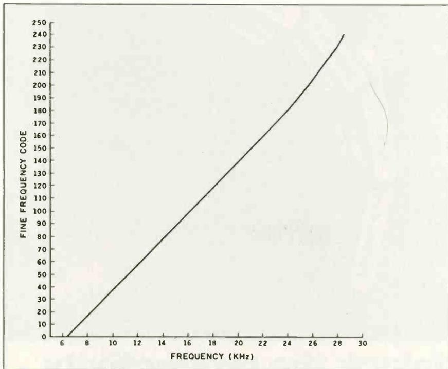
Figure 8: Graph of fine frequency versus output frequency.
