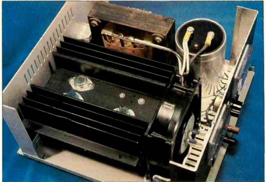
Photo 3: The completed power supply has little extra internal space. You'll notice that the filter capacitor has two sets of connecting wires to conform to the layout guidelines I've described. While the heatsink is sized properly for ambient air installations, I have added a fan to compensate for the insulating effect of the enclosure. To limit noise, the fan is controlled by a 130°F thermostat attached to the heatsink. The thermostat turns on the fan only when necessary.
