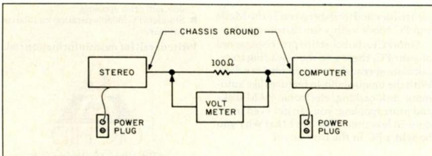
Figure 6: Potential ground problem test configuration.
