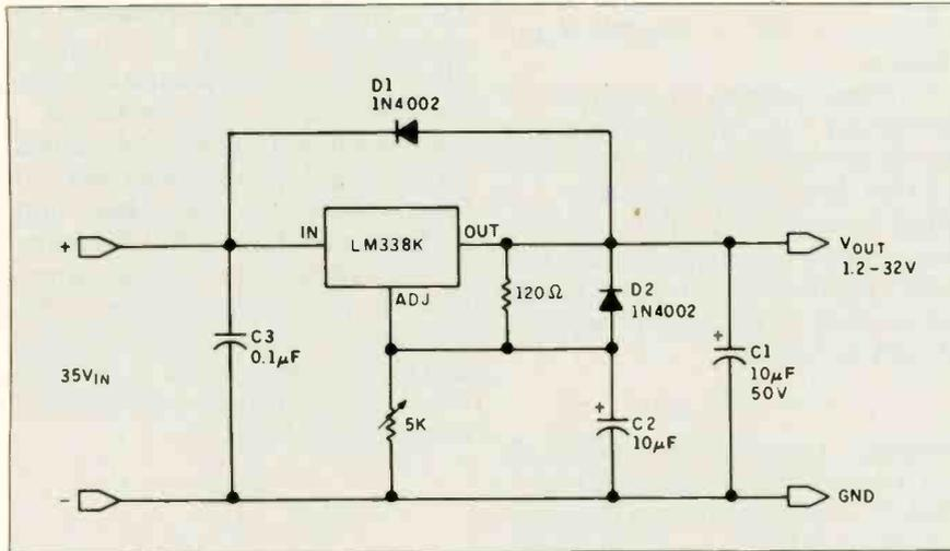
Figure 6: A typical variable-voltage three-terminal regulator.
