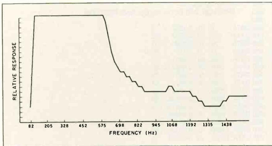
Figure 13: Frequency response with loudness filter on.
