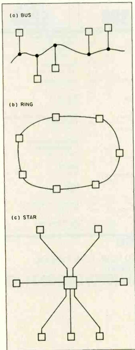
Figure 1: The bus, ring, and star topologies (or connection configurations) shown in their idealized forms.
