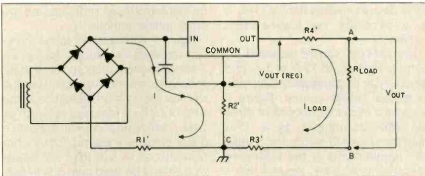
Figure 9: Sources of layout-induced errors in a typical three-terminal-regulator power supply.
