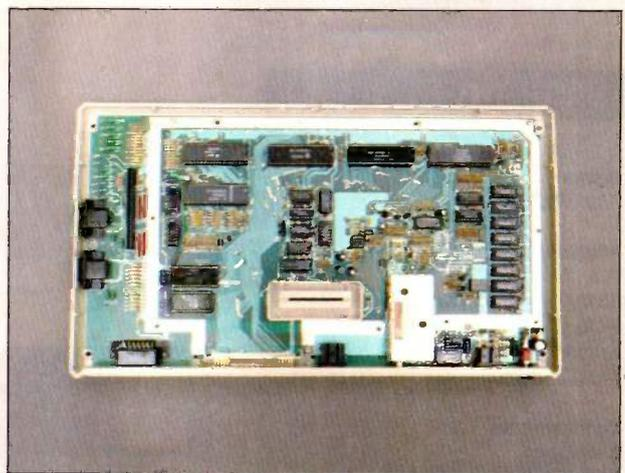
Inside the XL. From lower left, the single board contains the Antic chip, GTIA, 6502C, PIA, and then up toward POKEY (on the right side) the 16K-byte OS ROM, and the 8K-byte BASIC.
