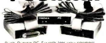
Push Button PC Switch lets you connect one computer to two printers, or modems, eliminate forms loading/unloading by keeping two dot matrix printers stocked, or pair one dot matrix printer with a slower Daisy Wheel printer for finished letters. Comes with 1 input panel connector, 2 output connectors on 6' ribbon cables.
