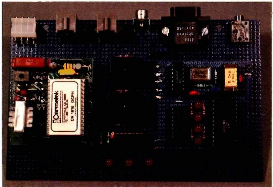
Photo 3: Prototype of the Touch-Tone Interactive Message System. The connectors from left to right are the power supply, answering-machine connector, telephone-line input, Microvox speech-synthesizer output, parallel I/O interface to computer, and the answering-machine earphone output.
