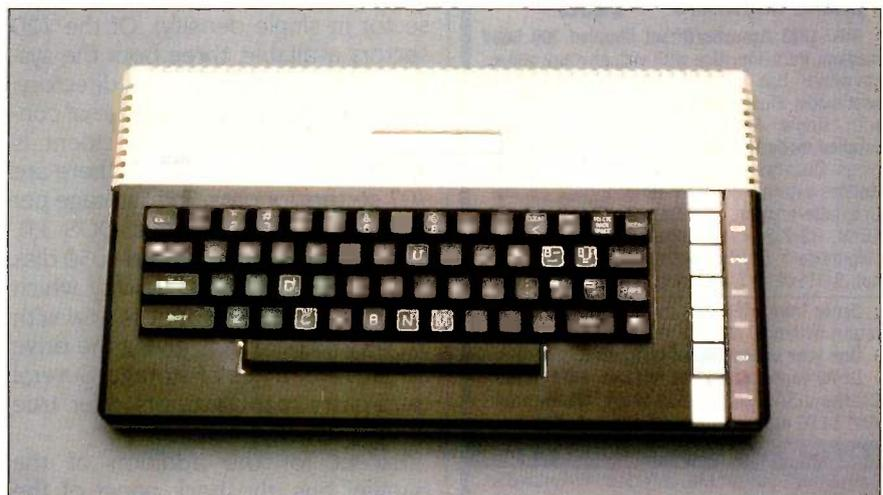
Photo 2: The keyboard of the 800XL. Note the better placement of the inverse-video key in the lower right corner.
