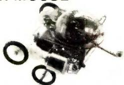
Controlled by sound sensor and 1-channel electronic circuit. Use the whistle in this kit and Piper-Mouse follows your commands, turning left or right, stopping and starting. Uses 2 AA and 1 9V battery (not included).
