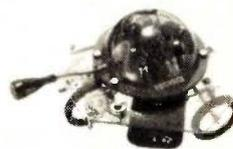
2-way sensor detects noise or solid objects in its path. When front sensor contacts an obstacle or hears a loud noise (hand-clap), Peppy automatically turns to the left.
