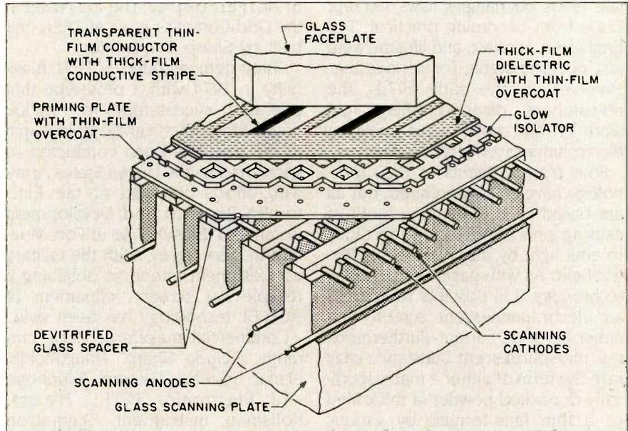
Figure 2: The hybrid AC/DC gas-plasma display developed by Burroughs Corporation to combine the virtues of the two types. An AC section serves as the display's memory, while the DC section is used for scanning the matrix.
