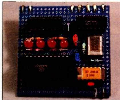
Photo 1: Prototype of the DTMF receiver board.
