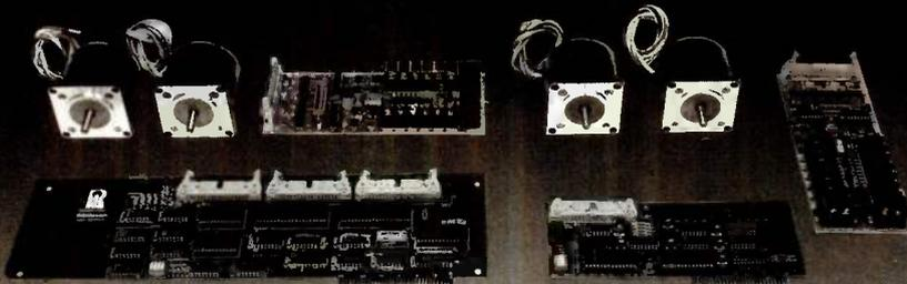
**Complete 2 axis systems using 2 size 23 stepper motors with R2D23 dual-axis driver; cable & powerful system software, expandable to 4 axis.**
