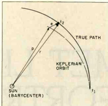
Figure 1: Illustration of Encke's model for calculating orbits around the sun;  $p$  is the radius vector of the Keplerian orbit,  $r$  is the radius vector of the true orbit, and  $e$  is the perturbation (the difference between  $p$  and  $r$ ).
