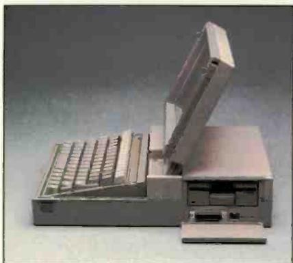
Photo 3: Behind the door on the Pro-Lite's right side is the 3½-inch disk drive, parallel printer interface, and power connector for a TI Portable Printer.
