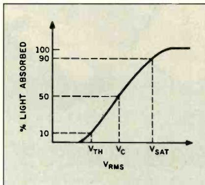
Figure 4: The threshold voltage is the rms voltage at which 10 percent absorption of incident light occurs.  $V_c$  is the voltage at which "on" pixels reach acceptable contrast (usually 2:1) to "off" pixels (those at  $V_{th}$ ) occurs.  $V_{sat}$  (saturation voltage) is the potential at which 90 percent of the light is absorbed.
