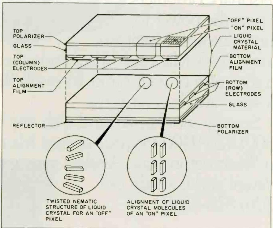
Figure 2: A cross section of a reflective liquid-crystal panel is shown. In the "off" state the LC molecules form a helix. In the "on" state (potential applied) the molecules align in the direction of the electric field.
