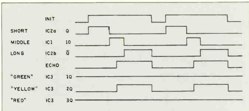
Figure 14b: High/low-limit ranging-sensor timing diagram.
