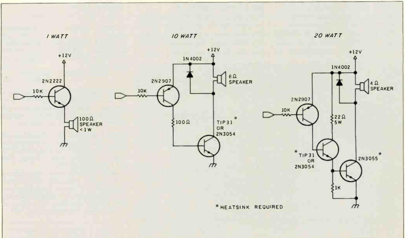
Figure 26: Power output stages for the design in figure 25.
