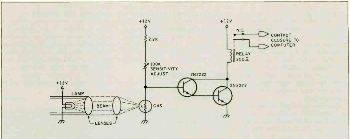
Figure 8: A simple light-beam alarm for doorways.
