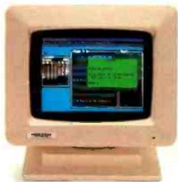
**HX-9/9E.** Nine inch, high resolution RGB monitor non-interlaced - .28mm dot pitch tube -9E compatible with IBM Enhanced Graphics Adapter -Nonglare screen -Green/amber switch -Apple/IBM colors - Etched dark glass screen -\$650/\$750 (9E)
