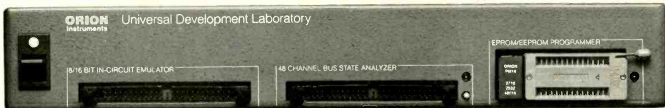
**32K bytes of EMULATION ROM (128K max)** allows you to make program patches instantly. Since the target ROM socket connects data and address lines to both the analyzer and the emulator, no expensive adaptors or personality modules are needed.
