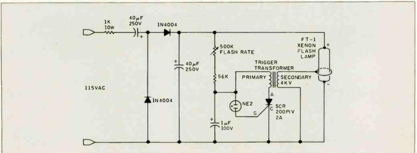
Figure 22: A 115-V AC xenon strobe light.
