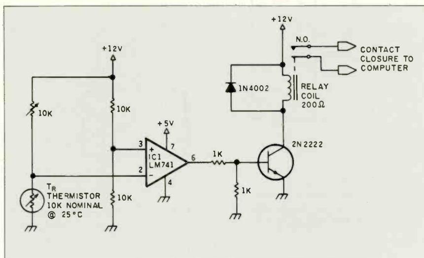
Figure 15: An over-temperature detector.
