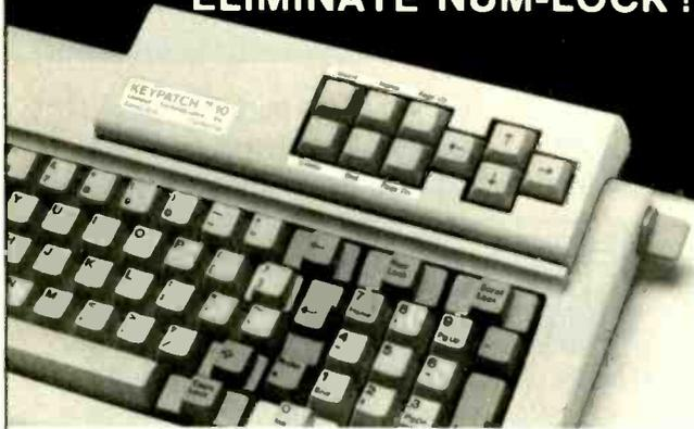
**KEYPATCH™ -10** - A full travel mini-keyboard. Plugs between keyboard connector and CPU. Automatically activates NUM-LOCK placing your IBM™ keyboard into the number pad mode while **KEYPATCH™ -10** provides separate cursor and screen control functions without the use of the NUM-LOCK key. Saves time — eliminates errors. **KEYPATCH™ -10** requires no software. A must for spread sheets; word processing; graphics; etc.
