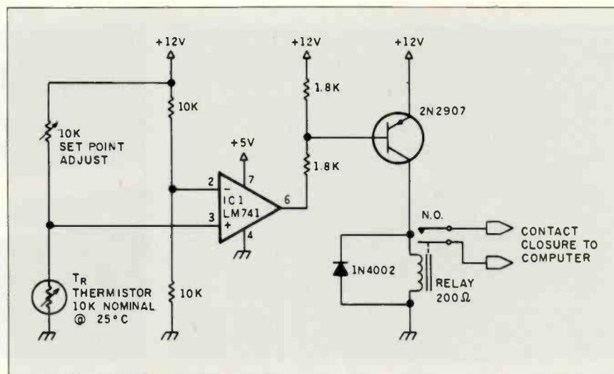
Figure 16: An under-temperature alarm.
