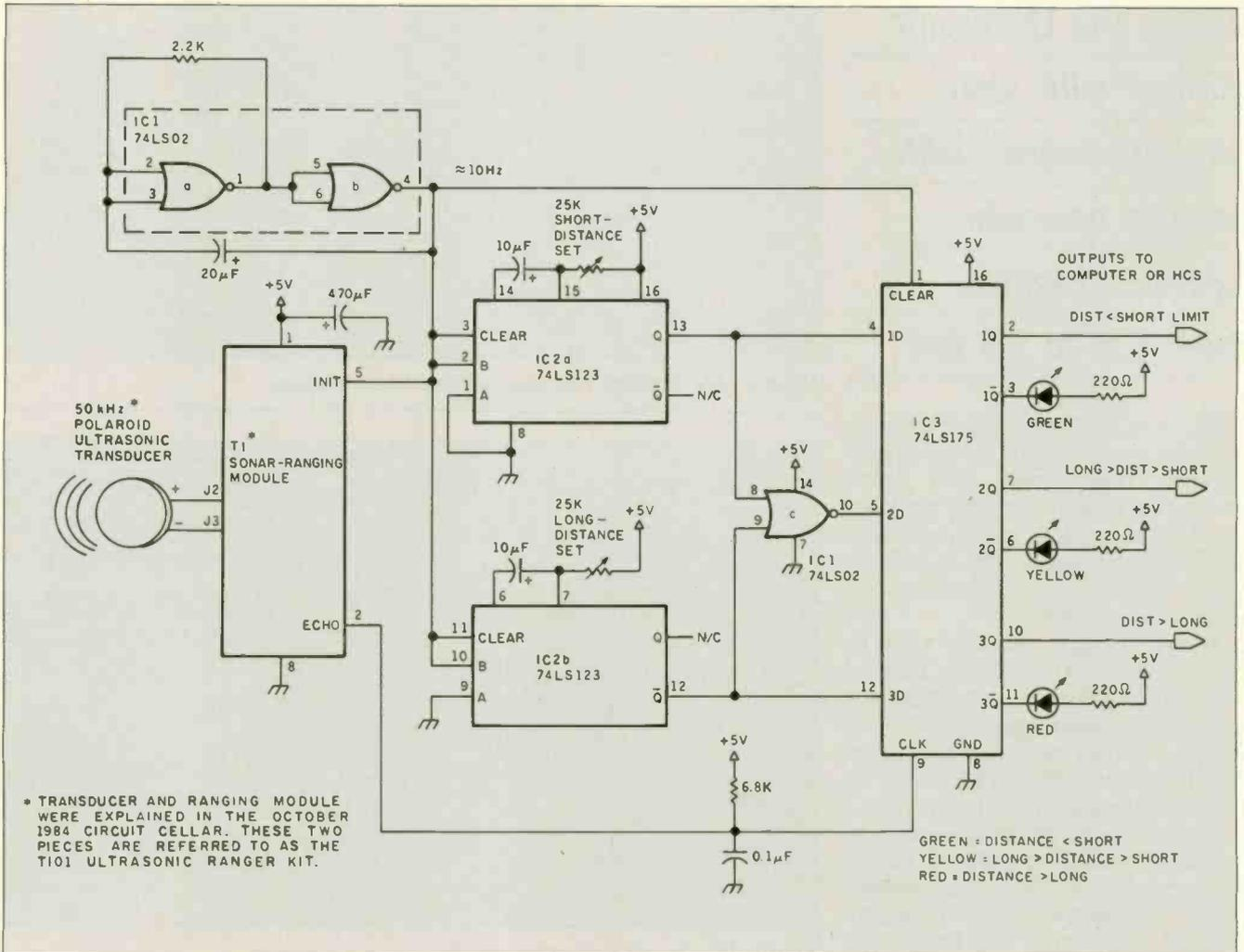
Figure 14a: The TI01 Ultrasonic Ranger.
