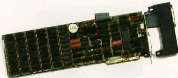
Simply, the best deal on a PC multifunction board--bar none. Basic Time's six function board, the **BT6Plus**, includes memory sockets for adding 64K to 384K, parallel printer port, asynchronous (RS-232C) serial communications port, battery-powered clock/calendar and electronic disk emulation & print spooling software. Optional game port. Comes complete with an easy-to-understand installation instructions/user's manual.
