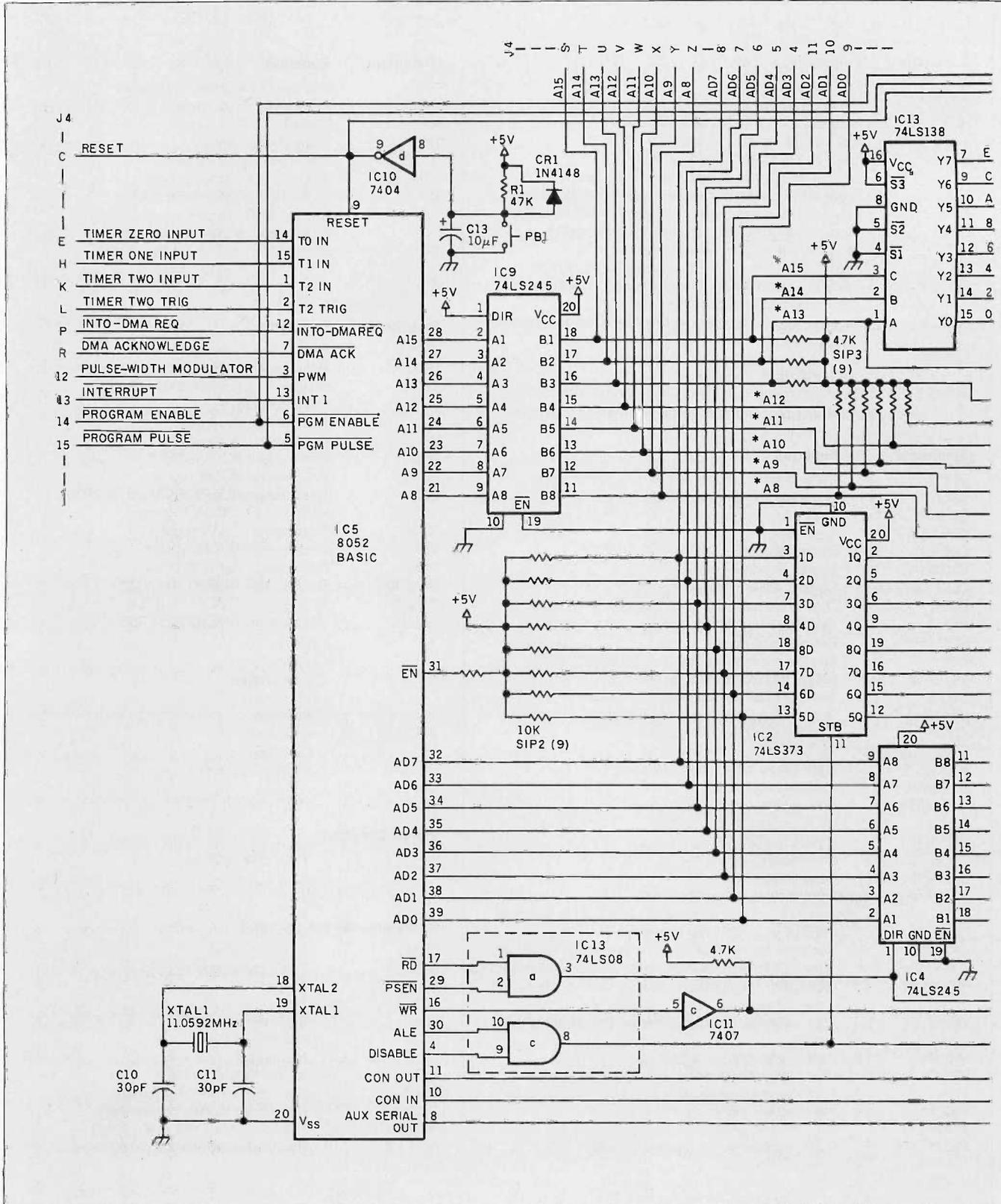
Figure 3: Schematic diagram of the BCC-52 board.
