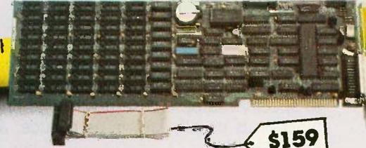
It gives you more than just added memory. It gives you reliable memory expansion (up to 384K), a serial port, a parallel port, a game port, and a battery back-up clock calendar. Includes RAM disk, print spooler, and clock utilities. (The 64K RAM set is only \$15.) With 2 serial ports \$175.
