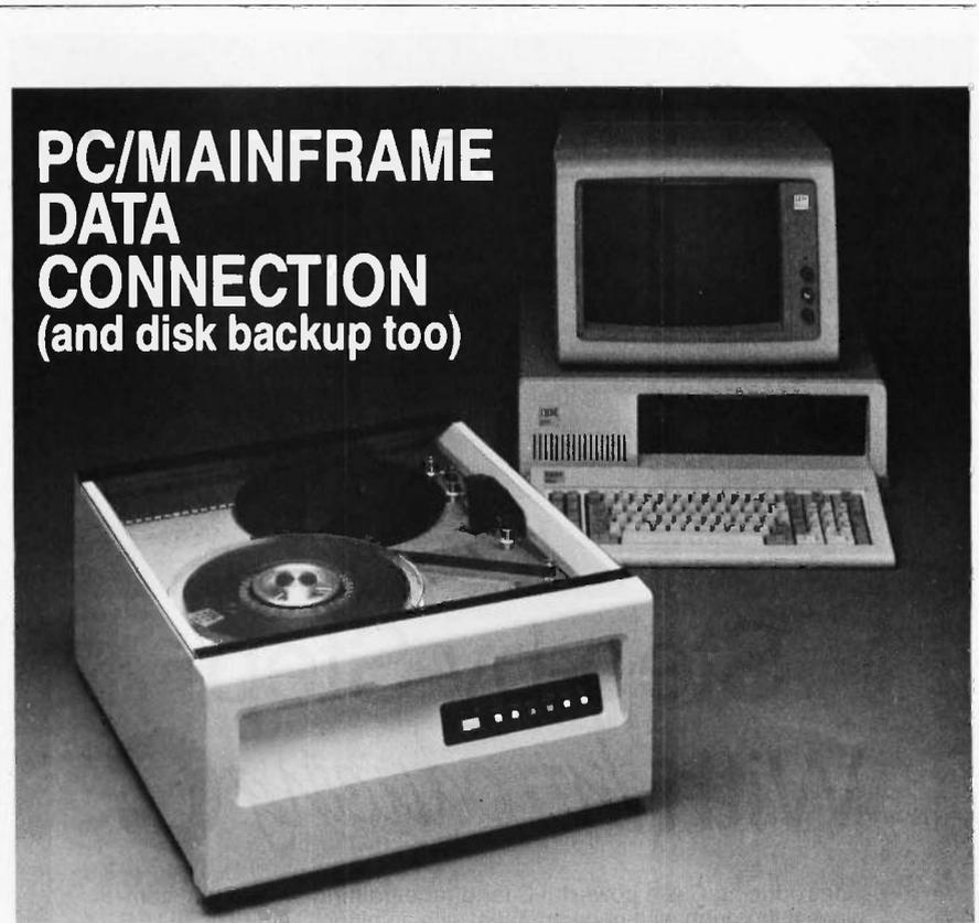
With the Digi-Data 2000 PC 1/2" tape system you can move data between your IBM PC, XT, or AT and a mainframe or minicomputer. IBM/ANSI compatible 9-track 1600 bpi 1/2" tape is the only truly standardized and interchangeable medium between the PC and mainframes or minis.
