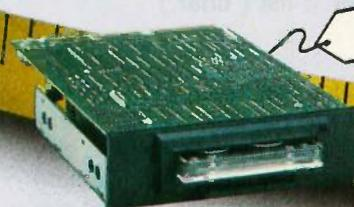
20 MB cassette and 60 MB cartridge back-up systems come with controller, cables and drive. Back-up 20 MB in 6 minutes. You can even do fast Image back-up and then file-by-file retrieval. Works on IBM PC, XT or AT. Internal 10 MB \$499, 20 MB \$699, 60 MB \$899. External 10 MB \$675, 20 MB \$875, 60 MB \$995.
