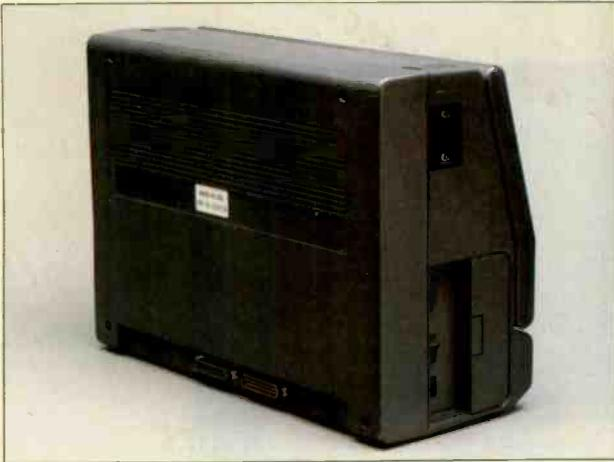
The rear of the Osborne 3 holds the parallel and serial ports.
