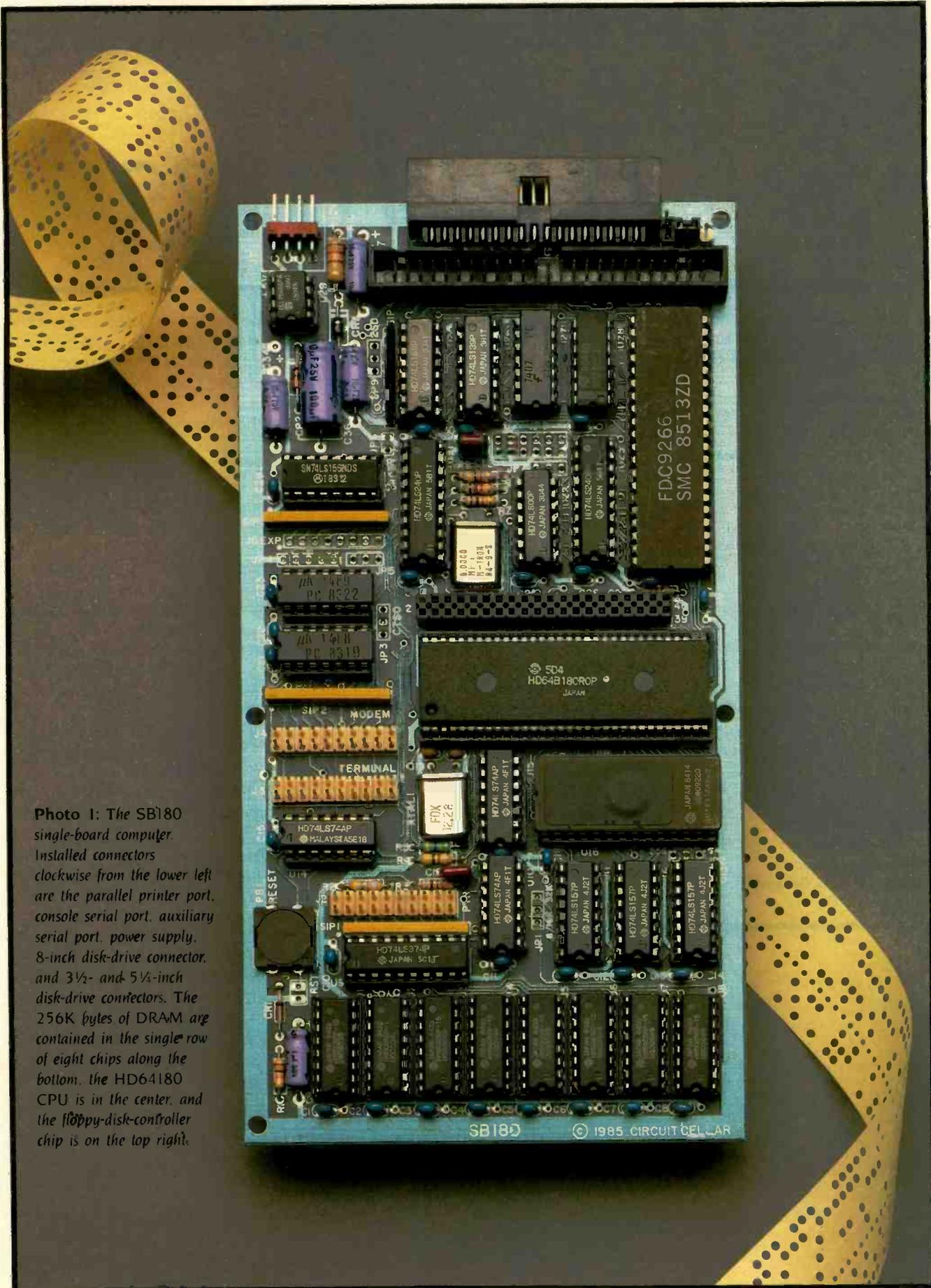
**Photo 1:** The SB180 single-board computer. Installed connectors clockwise from the lower left are the parallel printer port, console serial port, auxiliary serial port, power supply, 8-inch disk-drive connector, and 3½- and 5¼-inch disk-drive connectors. The 256K bytes of DRAM are contained in the single row of eight chips along the bottom, the HD64180 CPU is in the center, and the floppy-disk-controller chip is on the top right.
