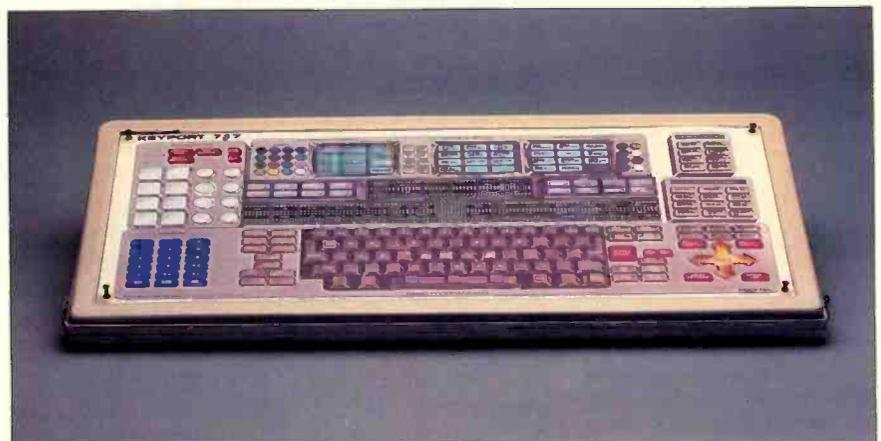
Photo 1: The Keyport 717 with the BASIC programmer's overlay.
