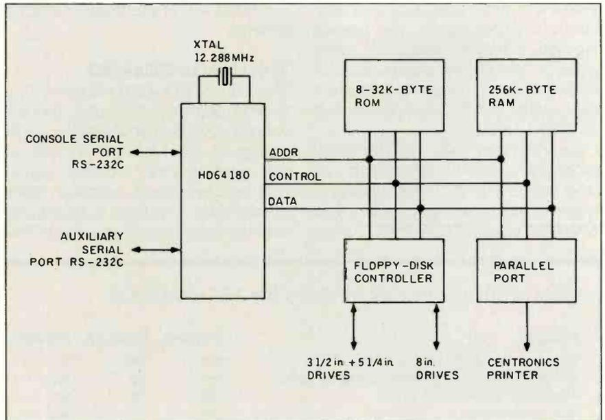
Figure 1: Block diagram of the SB180 single-board computer.
