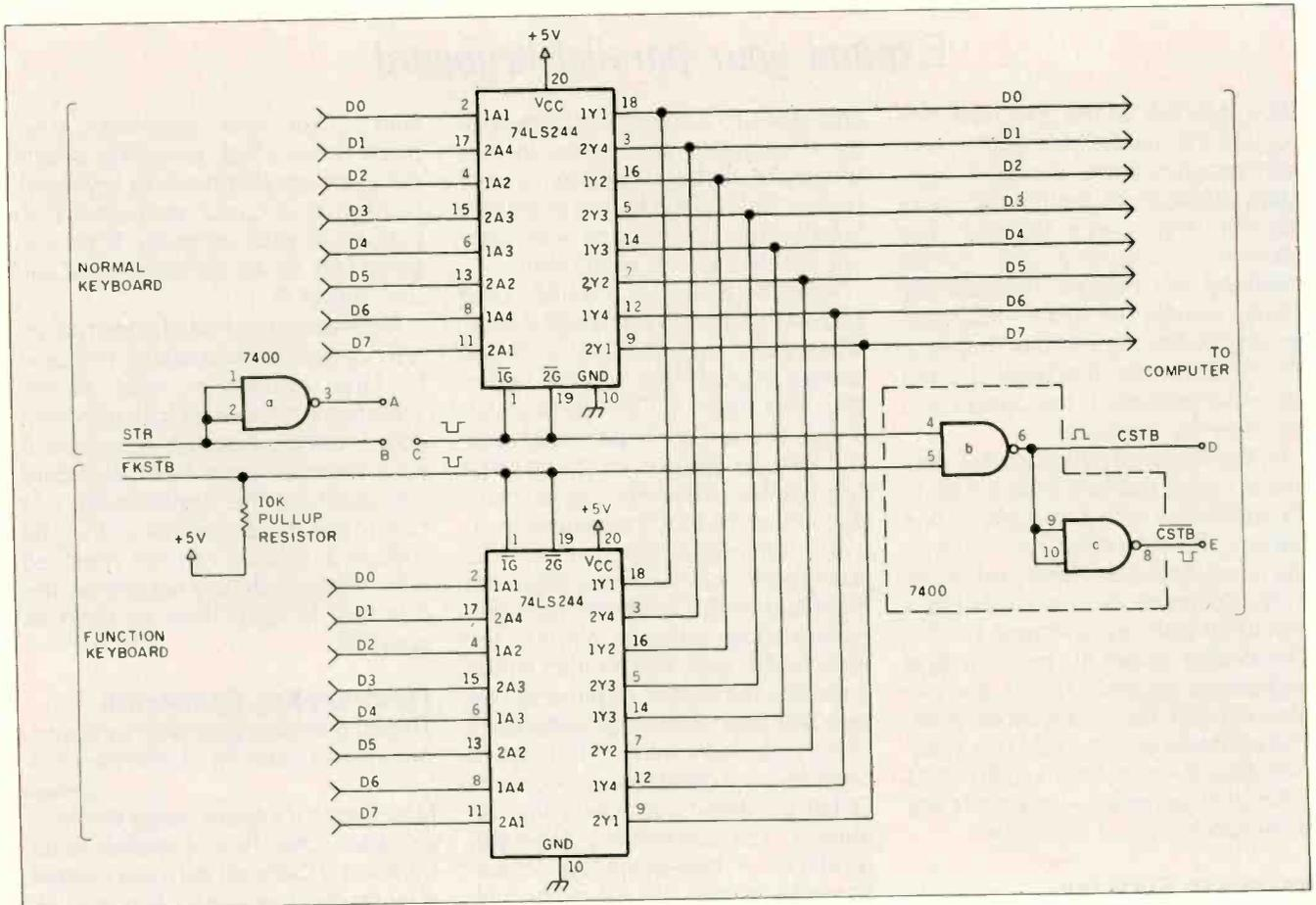
Figure 1: A schematic for the keyboard-splitter circuit.
