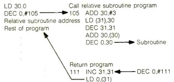
counter with the value 8, which is actually an unconditional jump to memory location 9 (since the program counter is automatically incremented at the end of every instruction). I can use any register as an index register. The simplicity gained by my instruction set resulted in a few strange-looking instructions. I have not yet found a use for some of the data instructions.
