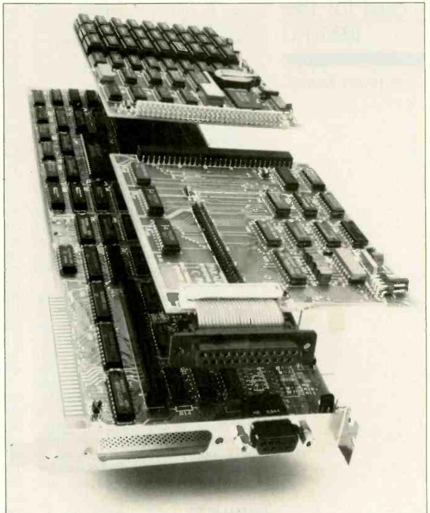
Photo 1: Modular Graphics Card from Paradise Systems fits into any full-size slot in an IBM PC or compatible. The connector at the bottom right of the photo mates with a cable from a monochrome TTL monitor. Also shown are two of Paradise's optional add-on modules; at the top is a combination RAM/clock card, and below that, a serial adapter card.
