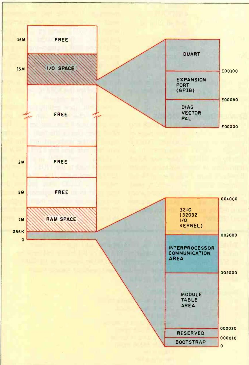
Figure 1: The DSI-32's memory map. 3210 is the I/O kernel that resides between locations 3000 and 4000. All addresses are in hexadecimal.
