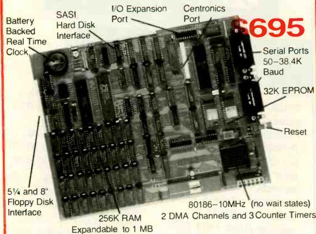
25% faster and double the RAM capacity of other 80186 boards make the Turbo-Mega-board the best value in single board computers at \$695. Fully assembled and tested, the Turbo-Mega-Board runs Turbo-DOS, CP/M-86 and MS-DOS. The advanced hardware and firmware features allow easy integration of a complete and powerful single or multi-user system. For more details call:
