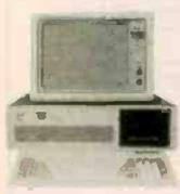
The **XAT** is our most versatile and powerful system. Using Intel's 80286 processor, the system runs at 6 and 8 MHz with a true 16-bit data bus. Comes standard with a 3 meg Add-On board, 2 parallel & one serial port, monitor, keyboard, DOS 3.1, two 1/2 height DS/DD 1.2 meg floppies.
