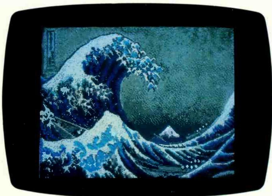
Photo 3: Low-resolution graphics offer 16 colors in a 320- by 200-pixel array.
