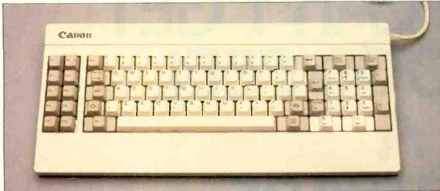
Photo 1: Keyboard of the Canon A-200 computer. It is identical to the IBM PC keyboard.
