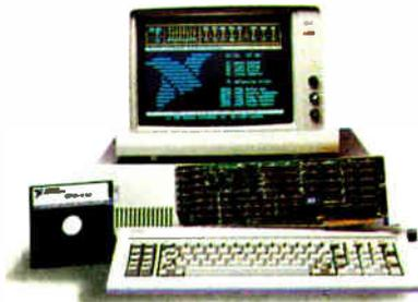
You can also use our Analyzer to run user-defined files of commands and data in order to prototype and debug GPIB systems. It comes as a single plug-in circuit card, and allows the PC to maintain its standard functioning.
