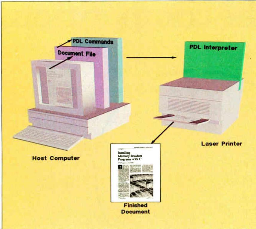
**Figure 6:** The document is created on the host computer and converted into a document file, in this case a Printerleaf file. A filter translates that file into the appropriate PDL. The PDL commands are passed to the PDL interpreter on the RIP. The RIP translates the commands in the pulses of the laser, which produces the finished document.
