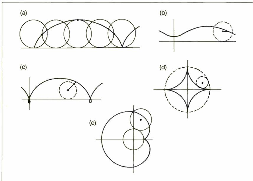
**Figure 1:** A variety of curves produced by rolling a circle along another curve: (a) simple cycloid; (b) curtate cycloid; (c) prolate cycloid; (d) hypocycloid of four cusps, or astroid; (e) epicycloid of one cusp, or cardioid.
