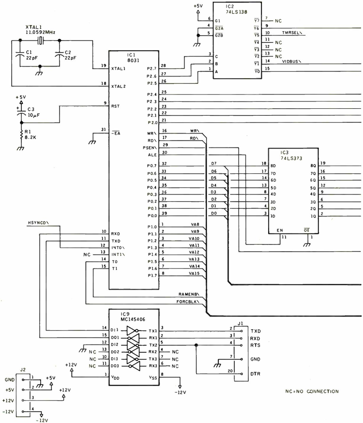
**Figure 5:** Schematic diagram of the ImageWise display/receiver hardware.
