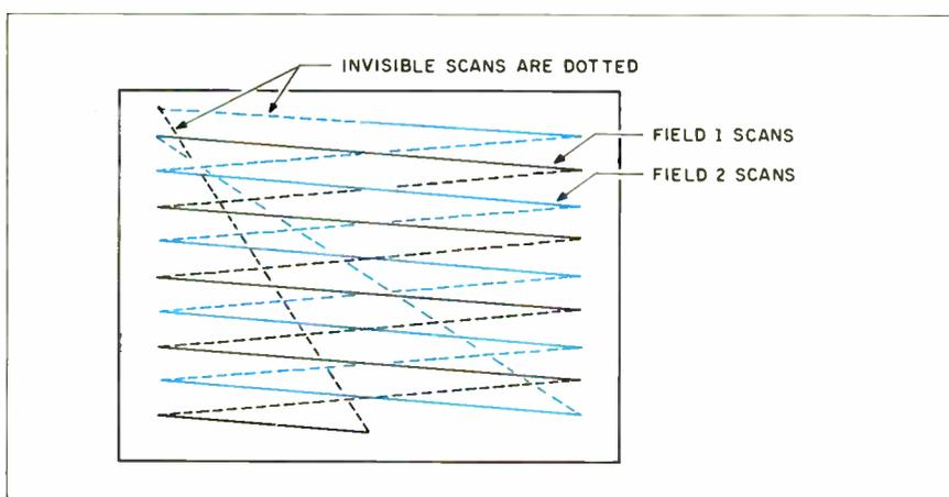
Figure 2: The path of the electron beam for an interlaced video scan.
