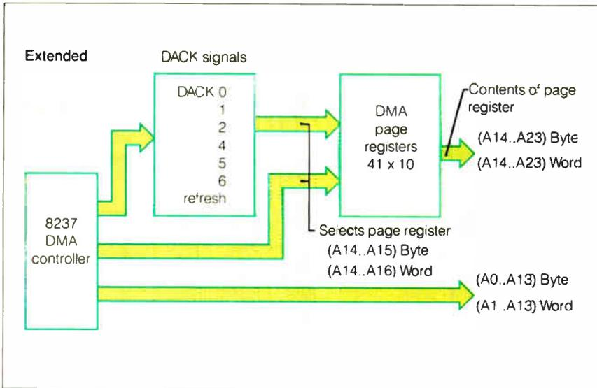
Figure 3: The extended-mode addressing scheme used by the memory mapper.
