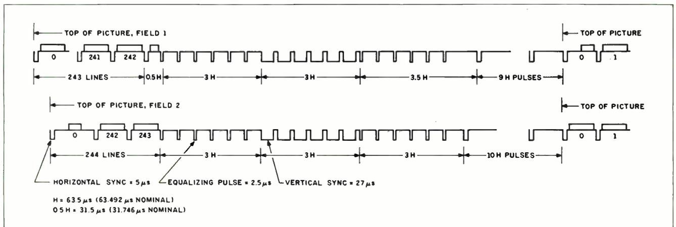
Figure 4: Signal voltage timing diagram for a complete field.
