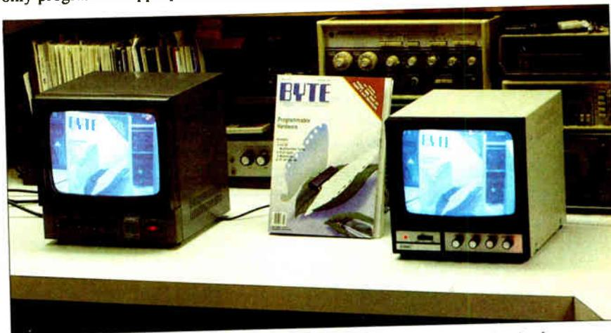
**Photo 6:** An in/out comparison. The camera is pointed at the magazine in the middle. The monitor on the left displays the image seen by the camera and the digitizer/transmitter. The monitor on the right shows the digitized image received by the display/receiver board.
