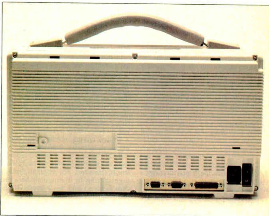
Photo 2: The rear view of the Portable III Model 20. Note the various ports, the sliding cover over the 96-pin port, and the machine's built-in padded handle.
