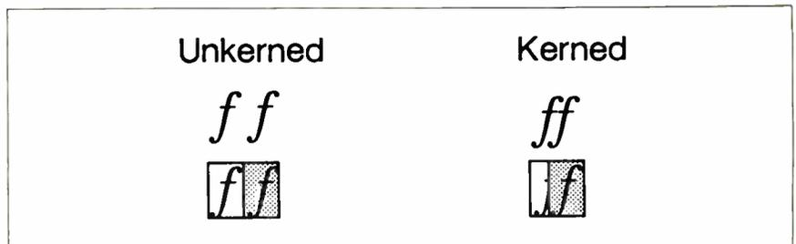
**Figure 2:** Unkerneled italicized *f*'s, shown on the left, each occupy an inviolate rectangle. Kerned letters, on the right, overhang each other, complicating the bit-mapping algorithms.
