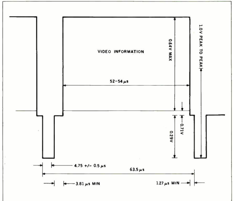
Figure 3: A profile of the signal voltage sent to the display during a single scan line. Note the bracketing 63.5-microsecond horizontal sync pulses.
