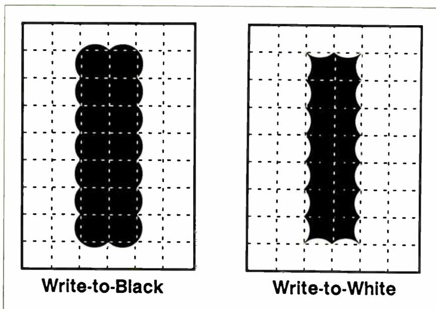
**Figure 1:** With write-to-black printers, black pixels are written to a white background. With write-to-white printers, white pixels are written to a black background. The resulting fonts can appear substantially different, as in the case of the sans serif's shown here. Hand-tuning fonts for specific printers can enhance legibility and style.
