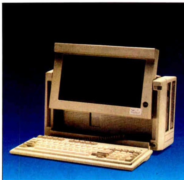
AT-compatible 8- or 16-bit add-on cards, an internal 300/1200-bps Hayes-compatible modem, and up to 6.6 megabytes of RAM.
