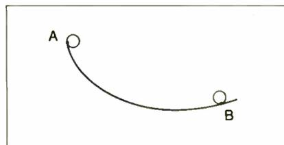
**Figure 2:** An inverted cycloid defines the path of quickest descent and the path of equal descent.
