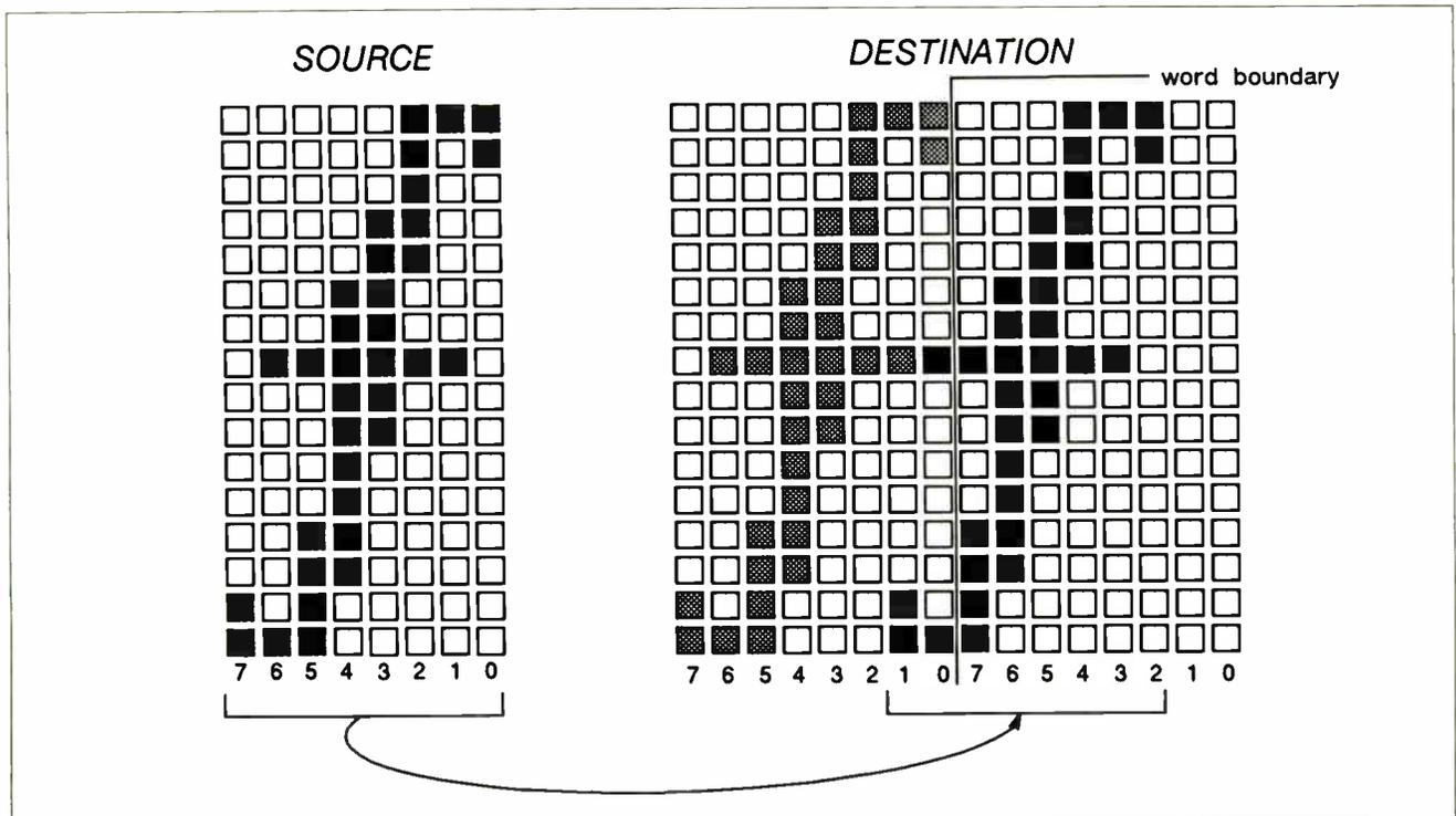
**Figure 3:** To move the source bit map row by row into the destination bit map (which can straddle word boundaries), each row must be shifted by the offset from the word boundary. In this case, the offset is six. In this example, kerned italicized *f*'s are shown, but the problem can occur with any letter. This figure uses 8-bit words to simplify the diagram.
