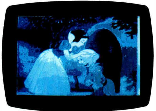
Photo 1b: The same image as displayed on an EGA 16-level gray scale.
