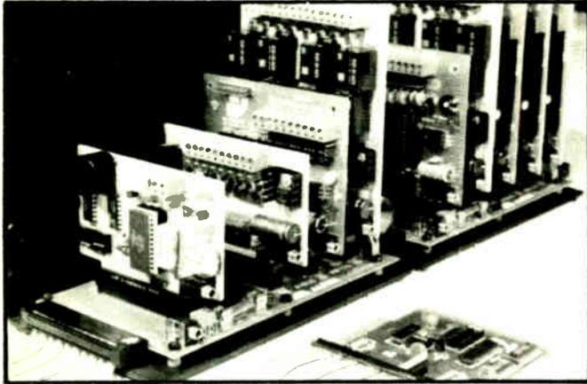
**An A-BUS system with two Motherboards**
