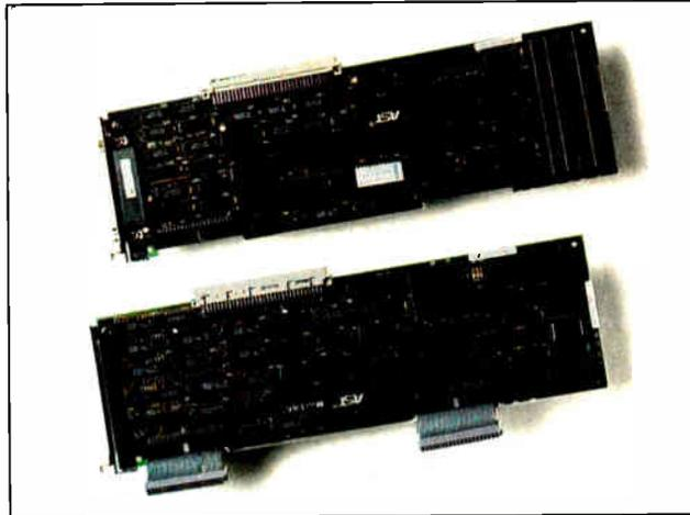
first board is a processor card with an 8-MHz Intel 80286 CPU and a socket for an 80287 math coprocessor. The second board contains the system's RAM. This RAM consists of four 256K-byte-density single in-line memory modules (SIMMs), providing 1 megabyte of parity-checked RAM. The first 640K bytes of RAM is MS-DOS user memory, and AST uses the remaining 360K bytes to house the PC ROM BIOS routines.
