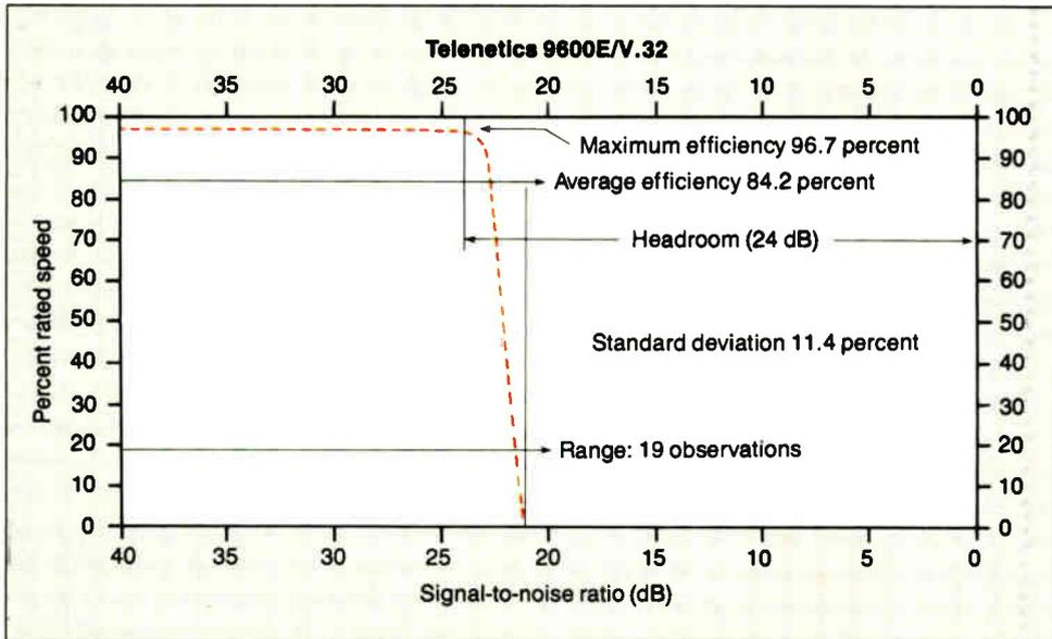
**Figure 1a:** The SNR Maps here and in figure 1b show that the Telenetics modem ran with greater efficiency than the Ven-Tel modem under typical line conditions. The Telenetics modem, though, showed a much narrower range of operation. Shown here are the raw test results for the Telenetics 9600E/V.32, a true V.32 modem. (In ideal performance, maximum and average efficiencies are high and close to one another, the standard deviation is a small value, and the range is a large value.)
