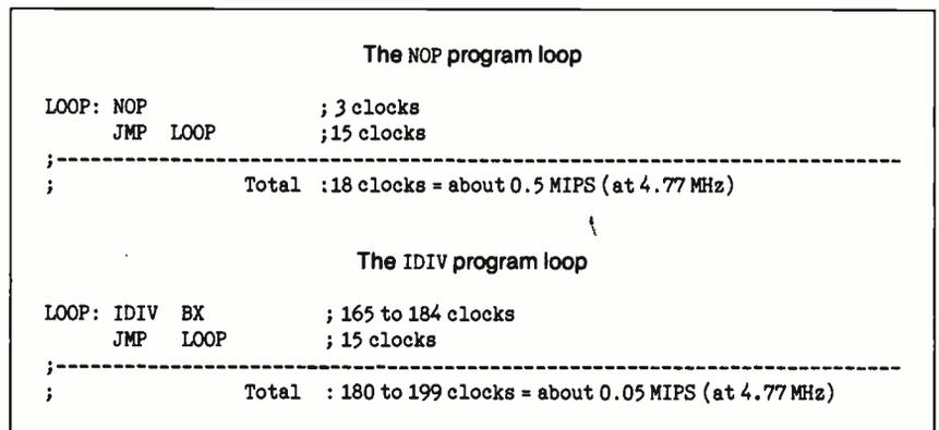
Figure 1: Why MIPS are meaningless. You could use either of these two code fragments to estimate MIPS on a machine, but their execution times differ significantly.
