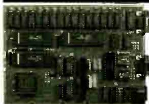
The GT180 has both TTL RGB (red, green, blue) intensity and analog RGB outputs, is totally compatible with virtually all standards and multicolor CRT monitors and has a connector for an IBM PC keyboard.
