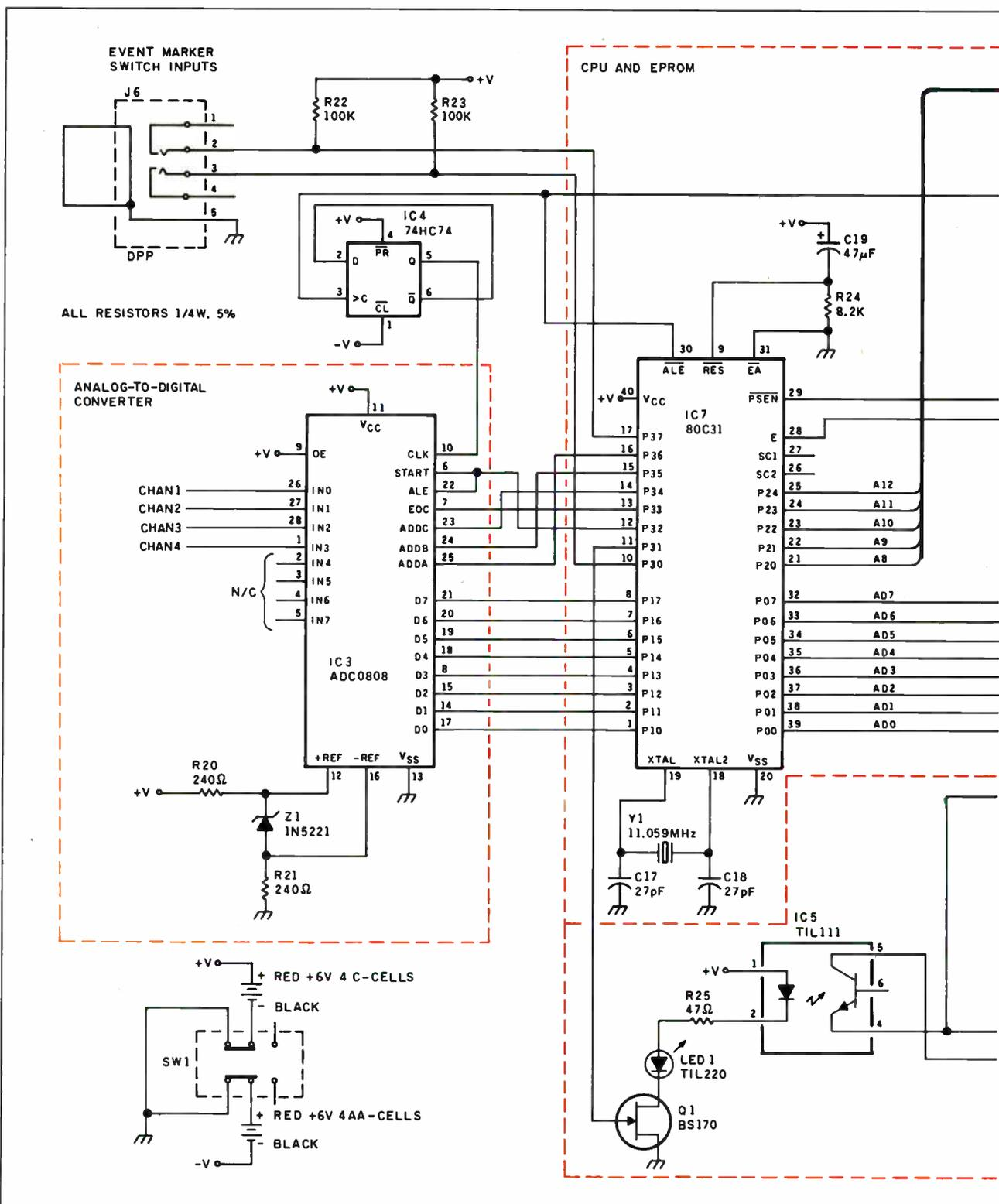
Figure 1c: HAL's A/D converter, on-board CPU, and RS-232C port.
