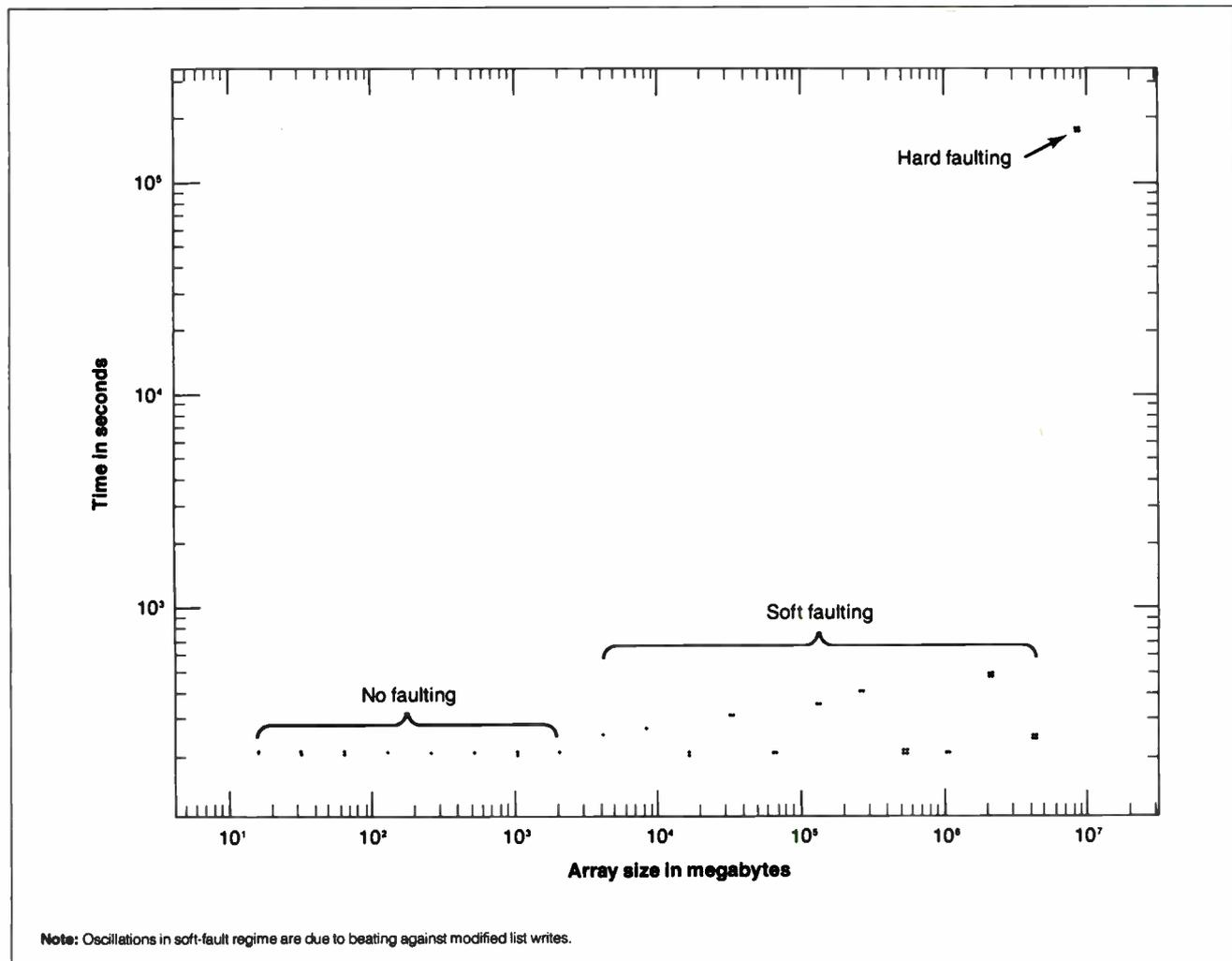
**Figure 2:** When a program tries to address memory outside the working set of directly addressable pages, execution time increases: slightly on a soft fault (memory found on the free list), and significantly on a hard fault (disk I/O required).
