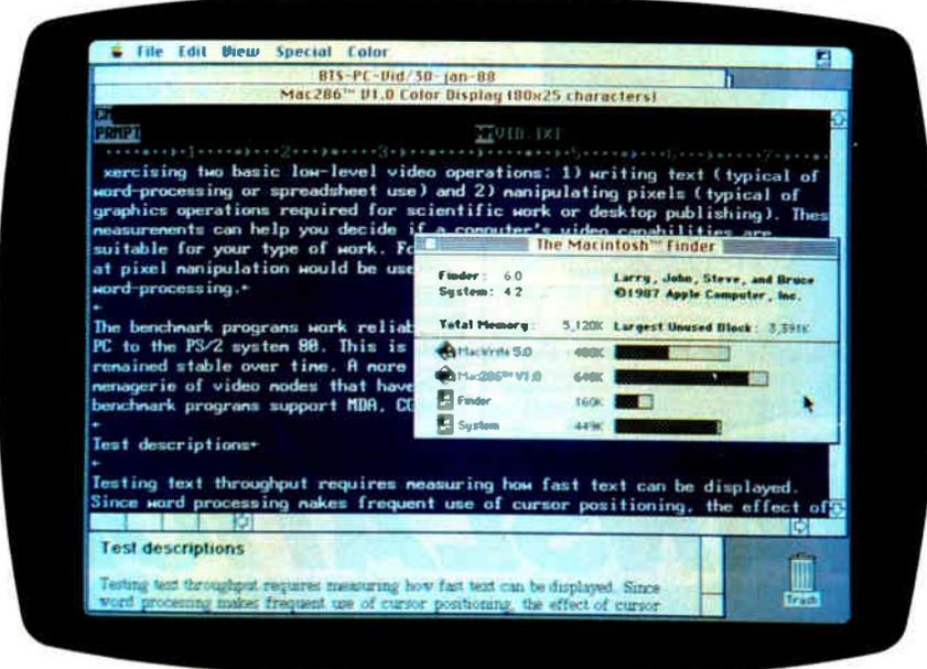
**Photo 1:** The Mac286 runs under MultiFinder on a Mac II with a 256-color display. The MacWrite document shown was just converted to a text-only file called VID.TXT and was copied to Mac286's drive C using the DOS command COPY D:VID.TXT C:. The document was then opened as it would be with XyWrite.
