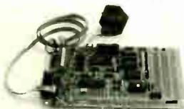
The SBC100 is a complete computer powered by a wall transformer. Available C compiler, assembler, linker and debugger run on a PC. Has battery-backed RAM, battery-backed clock, power fail interrupt, SBX bus connectors, serial and parallel I/O, prototype area for up to 20 IC's. Only \$295 including serial cable, power supply, 32k of battery backed RAM and schematics.
