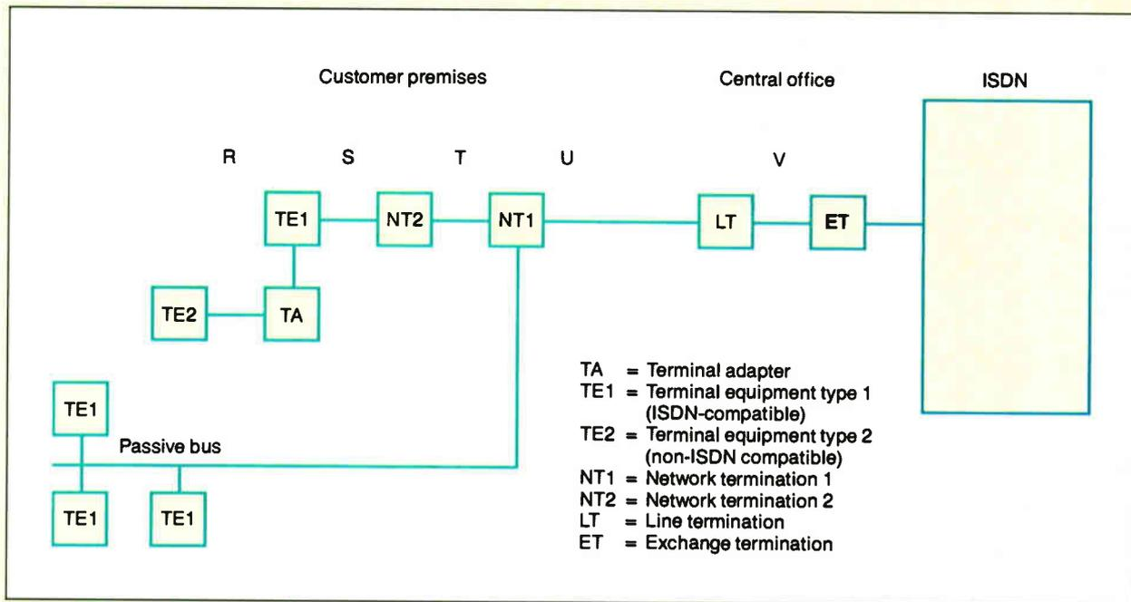
**Figure A:** The CCITT, a communications governing body of the United Nations, has designated five ISDN reference points: R, S, T, U, and V. These are places in the network where one or more interfaces for specific functions will occur.
