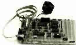
The SHC100 is a complete computer powered by a wall transformer. Available C compiler, assembler, linker and debugger run on a PC. Has battery-backed RAM, battery-backed clock, power fail interrupt, SHX bus connectors, serial and parallel I/O, prototype area for up to 20 IC's. Only \$295 including serial cable, power supply, 32k of battery backed RAM and schematics.
