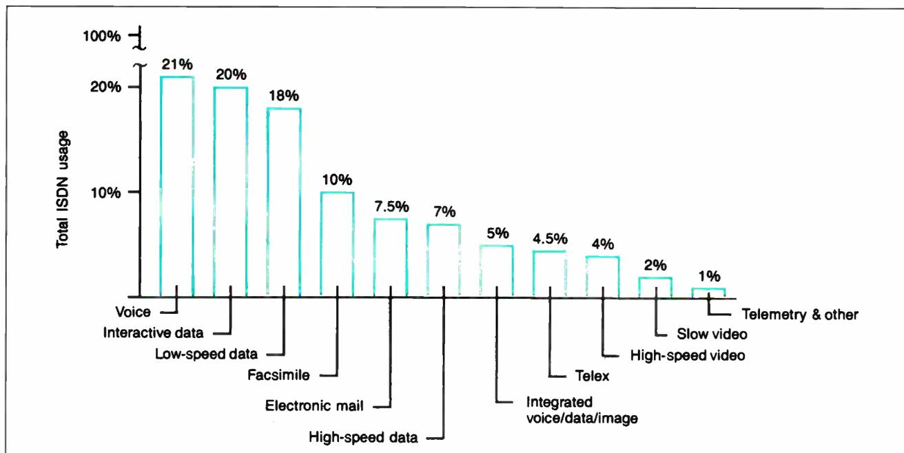
**Figure 3:** When ISDN is fully implemented, its largest usage will be for voice, interactive data, and low-speed data. As an emerging technology, however, ISDN may take off in directions unpredicted at this stage of the game.
