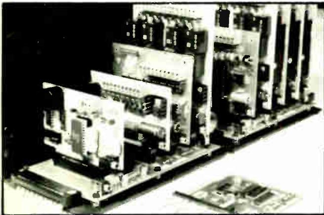
An A-BUS system with two Motherboards
