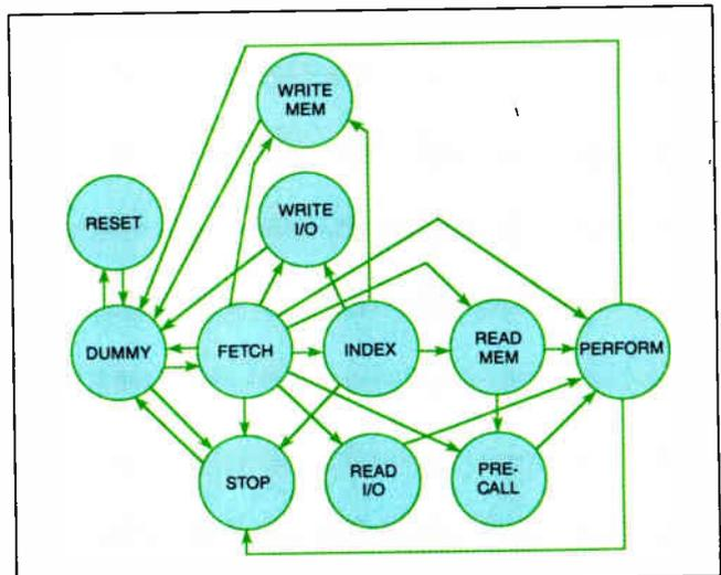
Figure 2: Eleven major states represent the mathematical model of the VIPER microprocessor.
