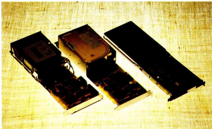
*The CompuAdd FlashCard 49, SPC Scorecard 44, and Plus Hardcard 40 trade top performance for compact size and ease of installation.*
