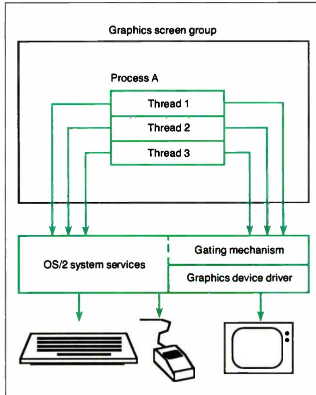
**Figure 2b:** An OS/2 graphics application needs three required threads, which use system services to access the keyboard and mouse but must use external graphics routines to access the graphics display.
