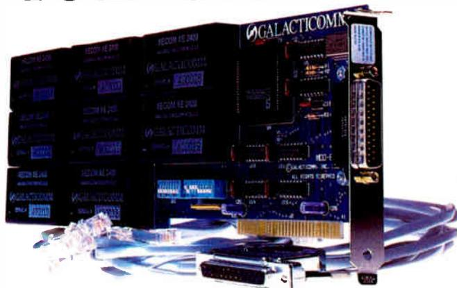
Our multi-modem PC cards are available in several configurations: 2 to 8 modems per card at 2400 baud, or 2 to 16 modems per card at 1200 baud. These are true single-slot cards with the modems built right in — no additional serial ports, power supplies, or external boxes of any kind are required.
