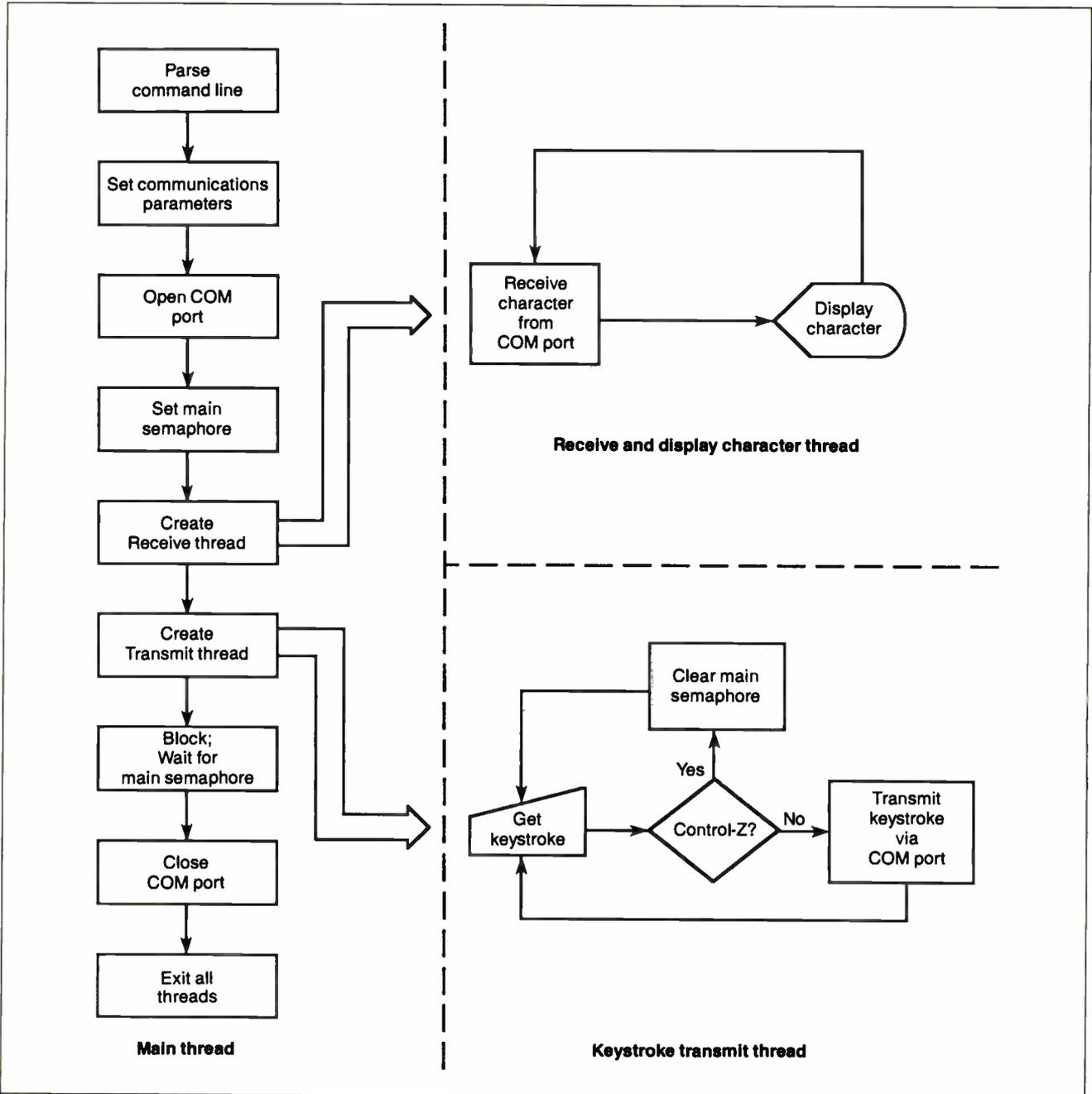
**Figure 1:** The main thread of OS2COMM creates two additional threads that do the actual communications processing: comtodsp receives characters from the COM port and displays them on the screen, and keytocom reads keystrokes from the keyboard and sends them to the COM port.
