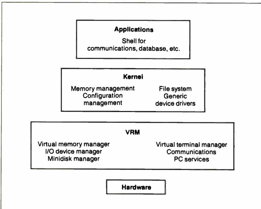
Figure 1: AIX's Virtual Resource Manager (VRM) hides the complexities of the hardware from the operating system software.
