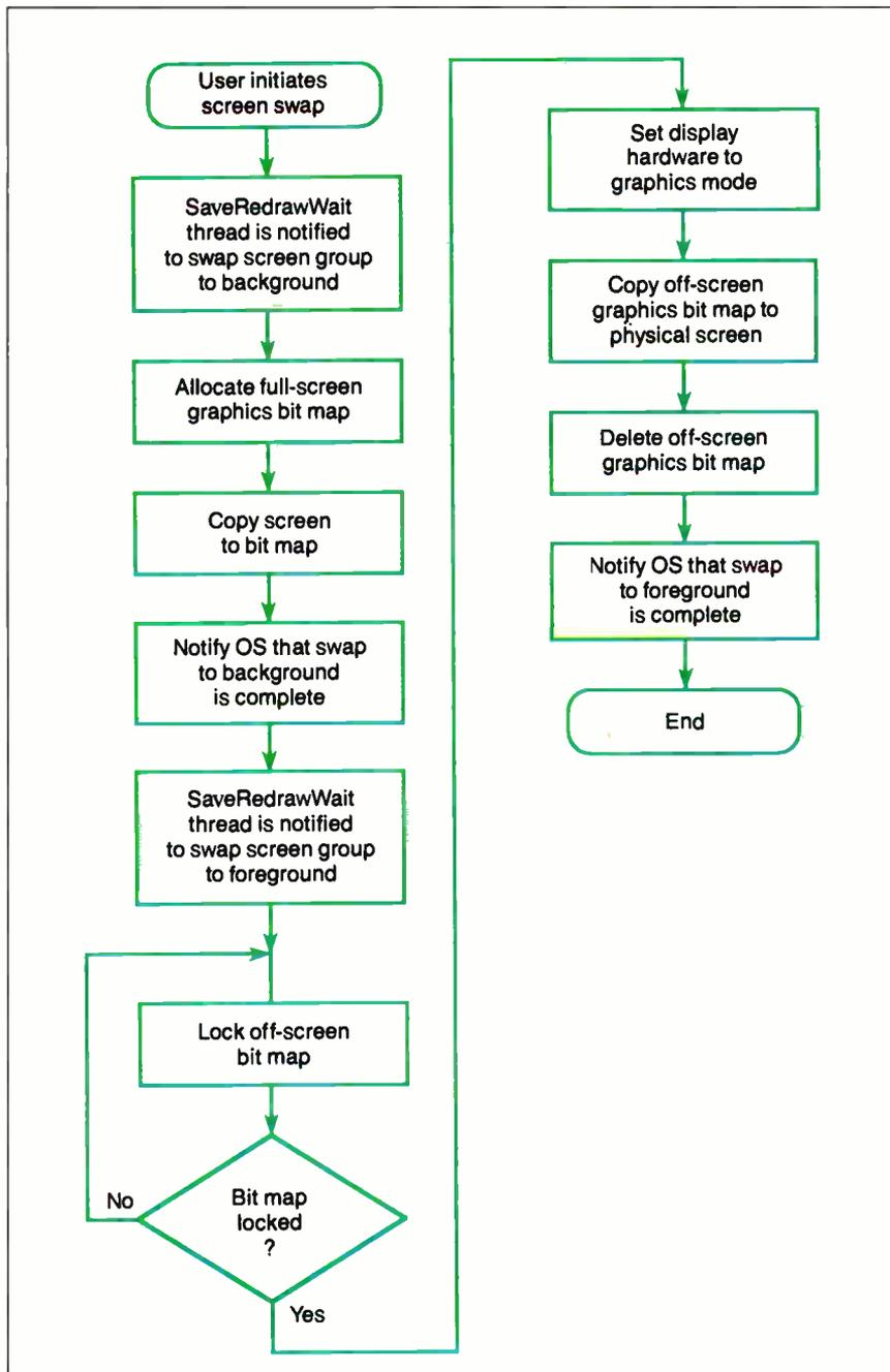
**Figure 3:** The left-hand portion of the flowchart illustrates the first part of a screen swap, where the foreground screen group is put into the background. The right-hand portion shows the second part of a screen swap, where the background screen group is put into the foreground.
