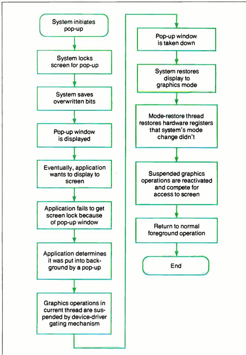
**Figure 4:** The left-hand portion of the flowchart illustrates the display of a pop-up window and what the foreground application does in response to the event. The right-hand portion shows what happens when the pop-up is taken down.
