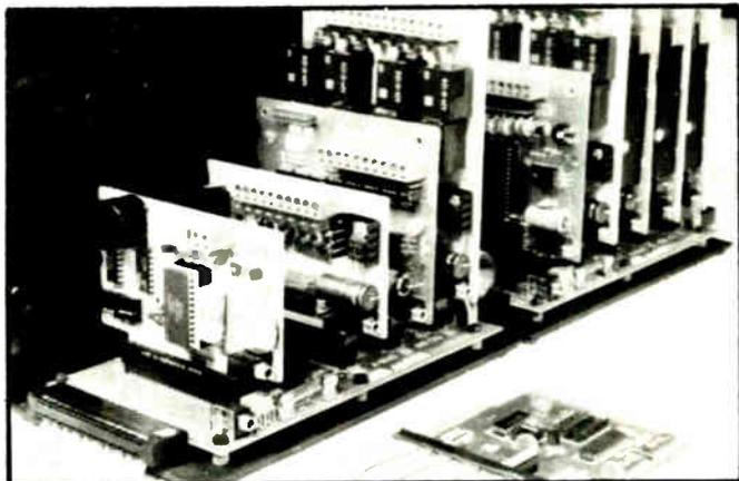
An A-BUS system with two Motherboards
