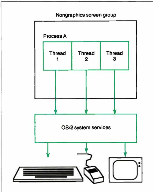
**Figure 2a:** In a nongraphics (alphanumeric) OS/2 application, a process's threads access input and display devices through system services.
