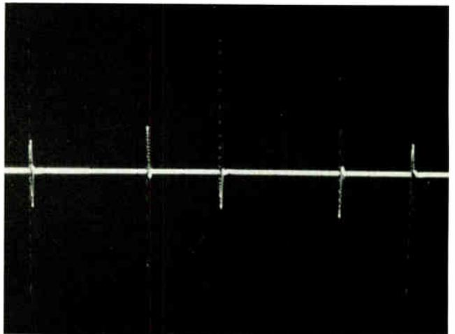
**Photo 2:** These innocuous-looking spikes are the output of the typical inexpensive SPS. They are actually 350 V in magnitude and can be the source of stress on your computer's power supply; they may even cause processing errors or damage to your computer's ICs.
