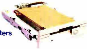
Includes 5.25" mounting frame for IBM PC/XT/AT and compatible computers. May require DOS 3.2 or higher for operation. The MF353B is compatible with the JE1043 and JE1049 Interface Cards (see page 259).
