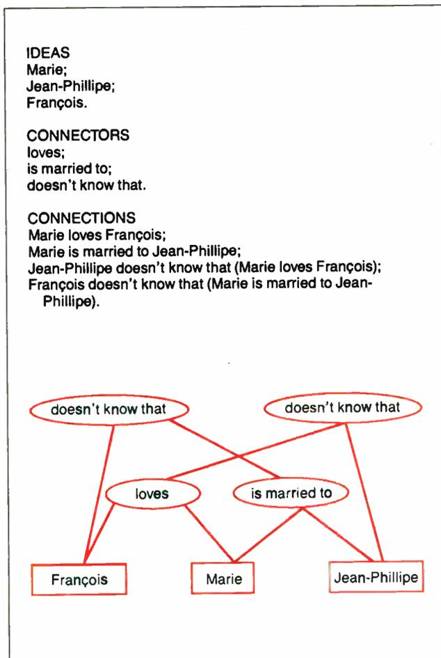
**Figure 4:** The outline generator performs its work by representing the ideas in each clause as nodes. As more and more links are created, a directed acyclic graph, such as this one outlining a movie plot, is constructed. Each connection is added to the graph by creating a new node with pointers to the two nodes it connects.
