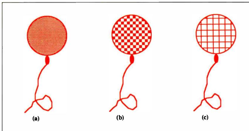
**Figure 5:** Treating the molecules in a gas as individual and unique leads to a fine-grained logically concurrent description (a), while grouping the gas into small but finite volumes leads to successively coarser descriptions (b) and (c).
