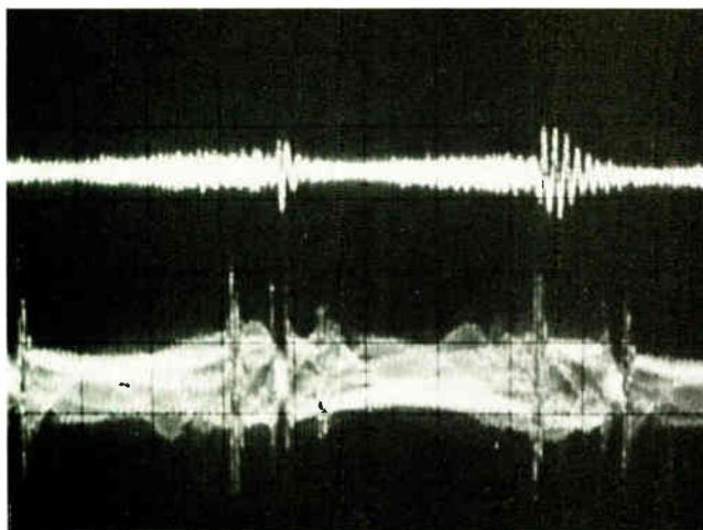
**Photo 4:** Normal-mode noise (top trace) and common-mode noise (bottom trace) after the insertion of an on-line UPS. The top trace contains a small amount of noise from the UPS's inverter. The bottom trace shows inverter noise superimposed over the common-mode noise present in photo 3. As you can see, the UPS has contributed to, rather than eliminated, common-mode noise.
