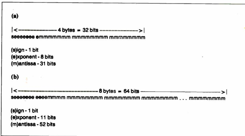
Figure 3: IEEE standard floating-point formats. (a) The format for 4-byte floating-point numbers (float). This representation has a range of  $\pm 3.4 \times 10^{-38}$  to  $\pm 3.4 \times 10^{38}$  and a precision of six to seven decimal digits. (b) The 8-byte double format, which has a range of  $\pm 1.7 \times 10^{-308}$  to  $\pm 1.7 \times 10^{308}$  and a precision of 15 to 16 decimal digits.
