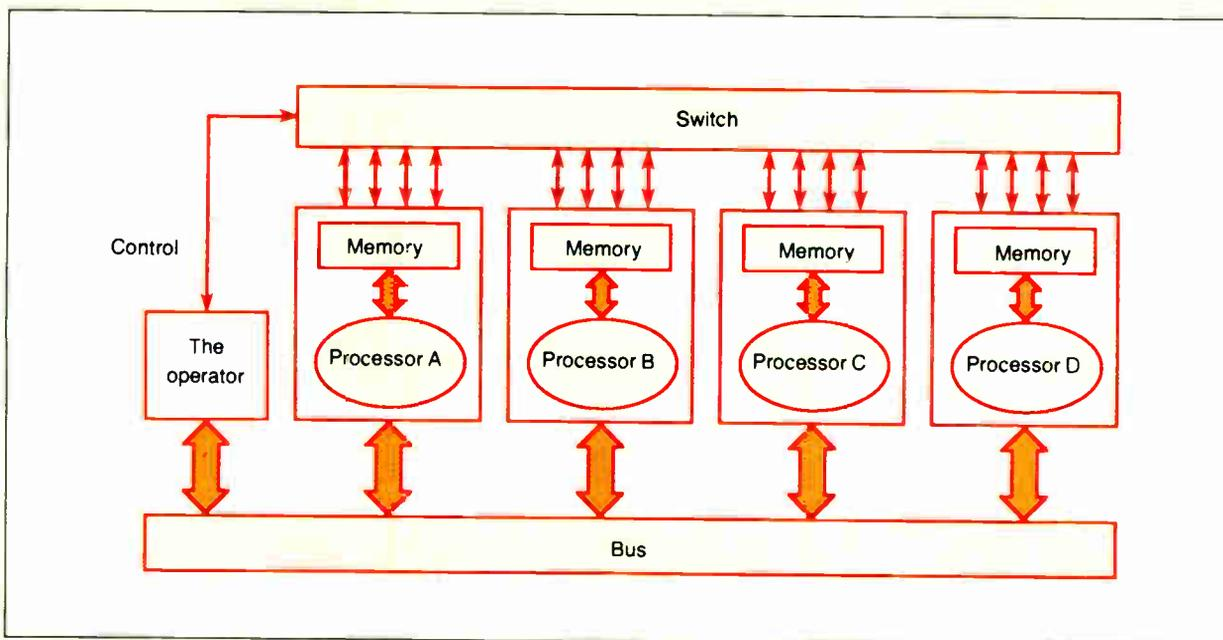
**Figure A:** The Cogent XTM's communications system. For A to exchange data with B, A notifies the switch controller via the communications bus. The controller then orders the intelligent switch to make a direct connection between A and B.
