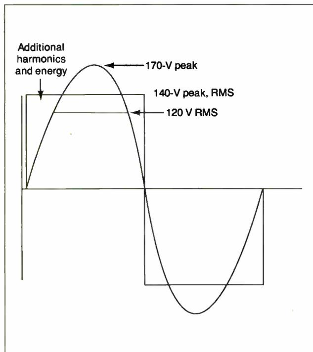
**Figure 2:** A comparison of the sine wave generated by utility power and the square wave produced by many SPSes. At any given point along the graph, a square wave contains more energy than a sine wave. Its peak voltage is equal to its RMS voltage.
