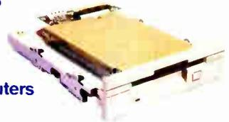
Includes 5.25" mounting frame for IBM PC/XT/AT and compatible computers. May require DOS 3.3 for operation. Also compatible with 720KB floppy disks. The MF355B is compatible with the JE1043 and JE1049 Interface Cards (see page 259).
