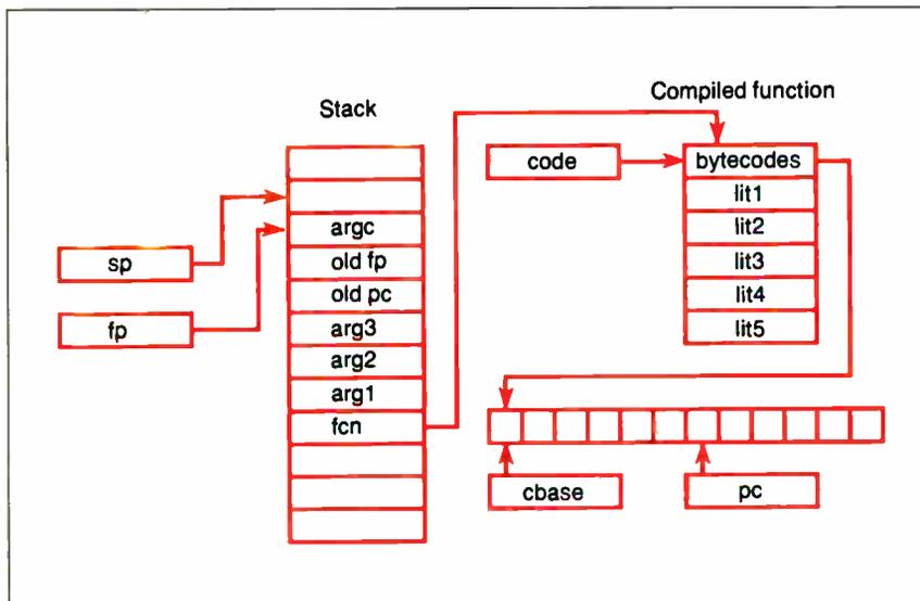
**Figure 1:** Inside the ExTalk virtual machine. The stack-pointer pseudoregister is `sp`, and the frame-pointer pseudoregister is `fp`. The pseudoregister `code` points to the current compiled function and is used for access to the literals. The `cbase` pseudoregister points to the base of the string of bytecodes associated with the current function, and `pc` points to the op code of the next bytecode instruction to execute.
