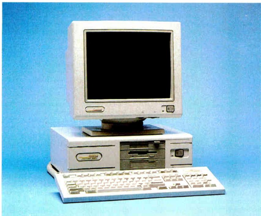
Compaq's 386s is the first of a new generation of microcomputers that implement Intel's low-cost 80386SX
