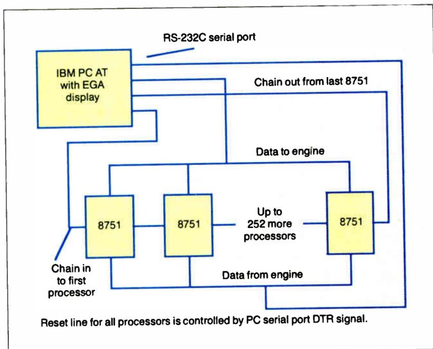
**Figure 1:** A block diagram of the Circuit Cellar Mandelbrot engine.
