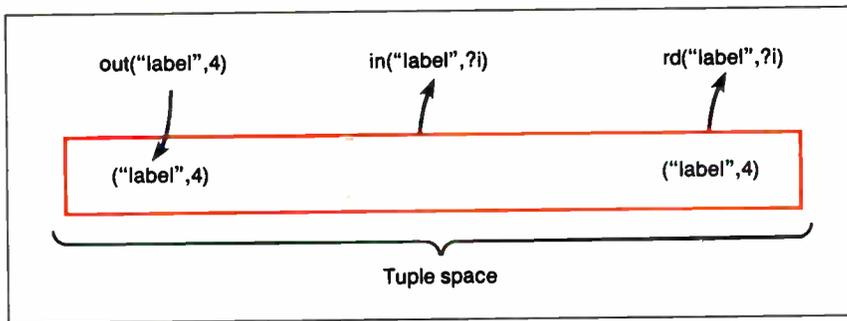
**Figure 1:** *The instruction out("label", 4) adds this tuple to tuple space while in("label", ?i) withdraws a matching tuple from tuple space; rd("label", ?i) simply reads a matching tuple without removing it.*
