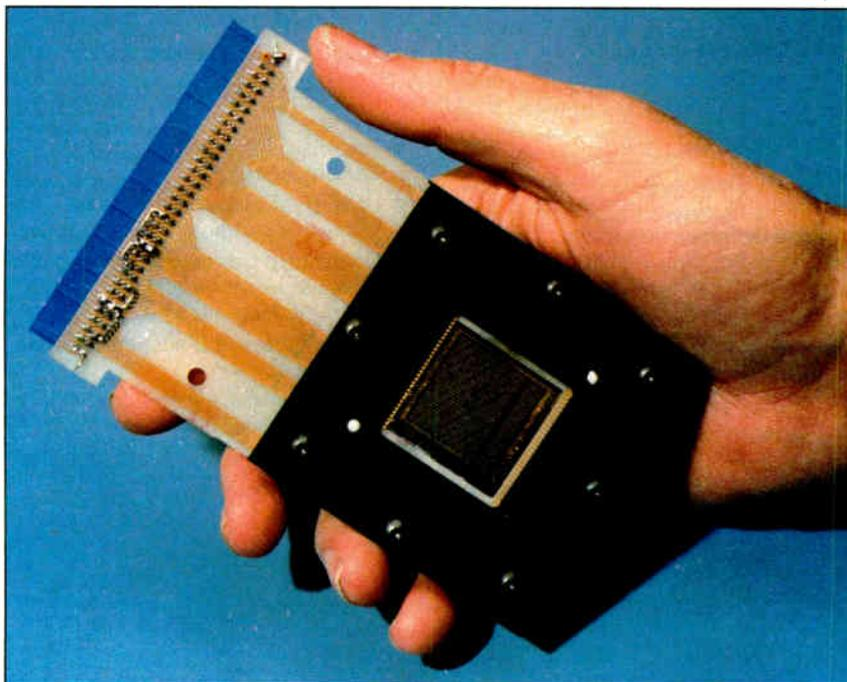
**Photo 1: A "hand-held" computer. The 1-inch square in the black section is the 32- by 32-element 3-D Computer.**
