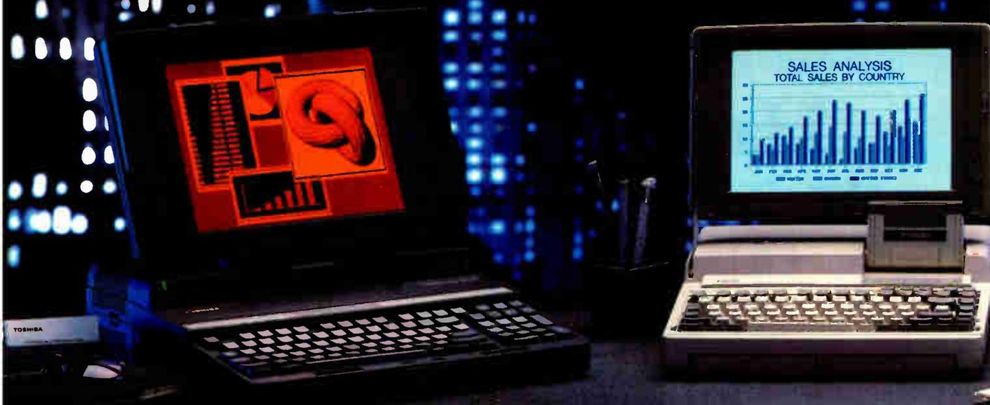
*T5200: 20MHz 386 processor, 2 internal IBM<sup>®</sup> compatible expansion slots, VGA gas plasma display with VGA monitor port, 40MB or 100MB hard disk, 2MB RAM standard expandable to 8MB, 1.44MB 3½" diskette drive.*
