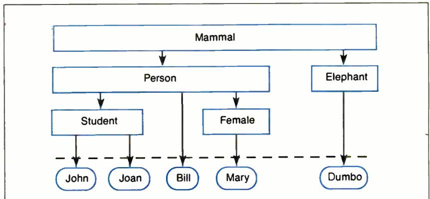
**Figure 3:** An inheritance hierarchy. Persons and elephants are defined as subclasses of mammals, and students and females as subclasses of persons. Instances (below the dotted line) are grouped into classes, while classes (above the dotted line) are categorized by their superclasses.
