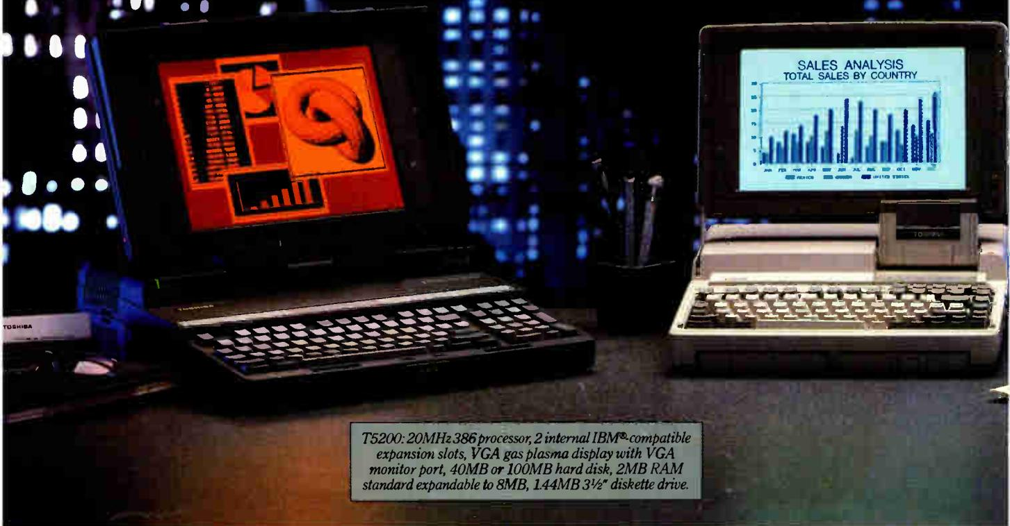
*T5200: 20MHz 386 processor, 2 internal IBM®-compatible expansion slots, VGA gas plasma display with VGA monitor port, 40MB or 100MB hard disk, 2MB RAM standard expandable to 8MB, 1.44MB 3½" diskette drive.*
