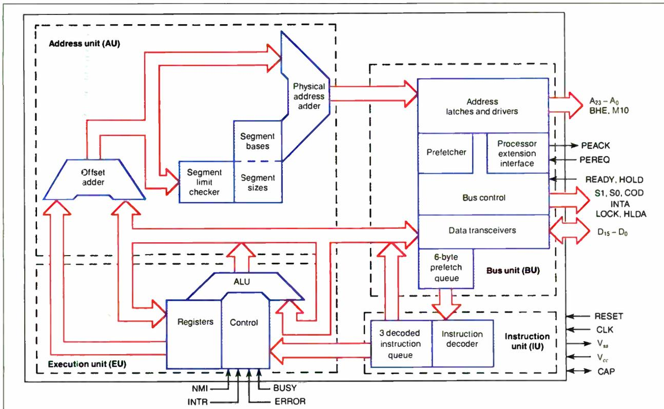
**Figure 1:** The 80286 CPU architecture. Though there are provisions for many sophisticated memory management and process-control features, the majority of applications only use the chip as a fast and efficient 8086.
