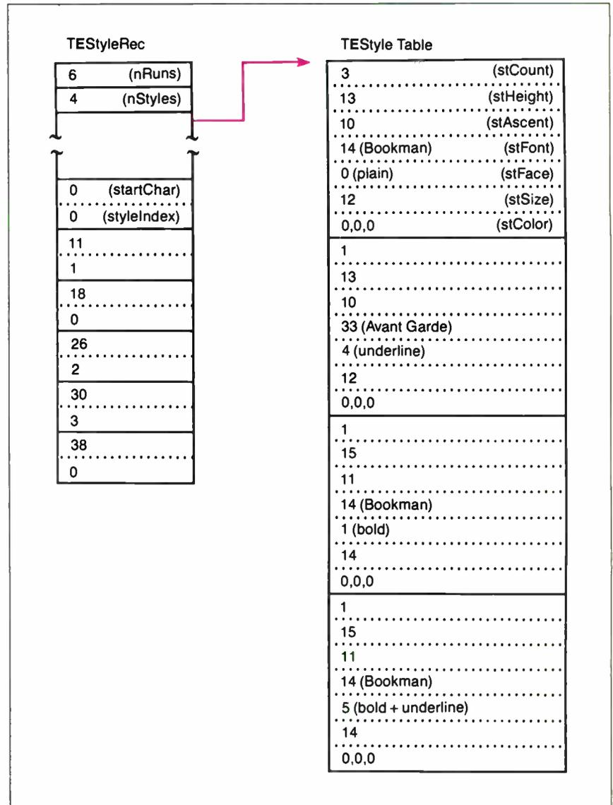
**Figure 2:** Style-run record giving the starting character offset from the beginning of the text, and an index into the style table.
