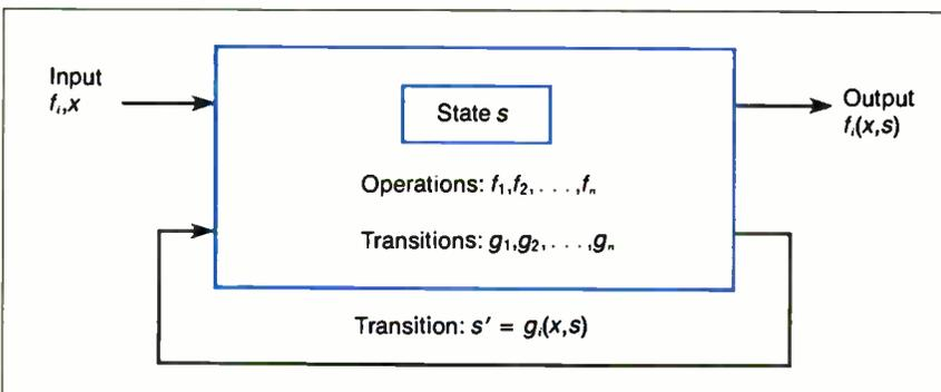
Figure 2: An object with operations  $f_1, f_2, \dots, f_n$ . Thus, operation symbols  $f_i$  are associated with symbols on the input tape, internal actions are associated with the state-transition function  $g_i(x, s)$ , and outputs are associated with operations  $f_i(x, s)$ .
