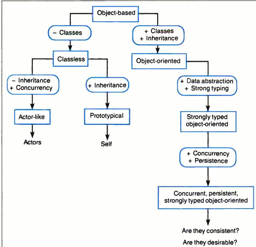
**Figure 6:** Classes of object-based languages. Note how the language features are used as design dimensions of a language design space. There is a potential language class corresponding to each of the 128 subsets of the seven language features, but some of the classes are more interesting than others.
