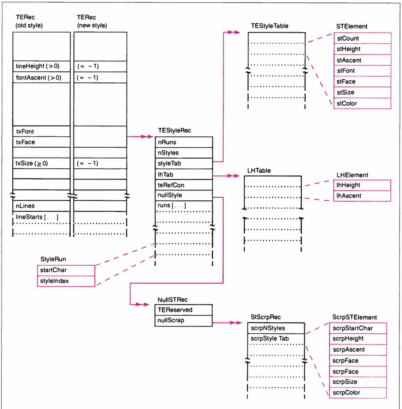
Figure 1: The new text-edit record and auxiliary structures. The double-headed lines indicate handles to data.
