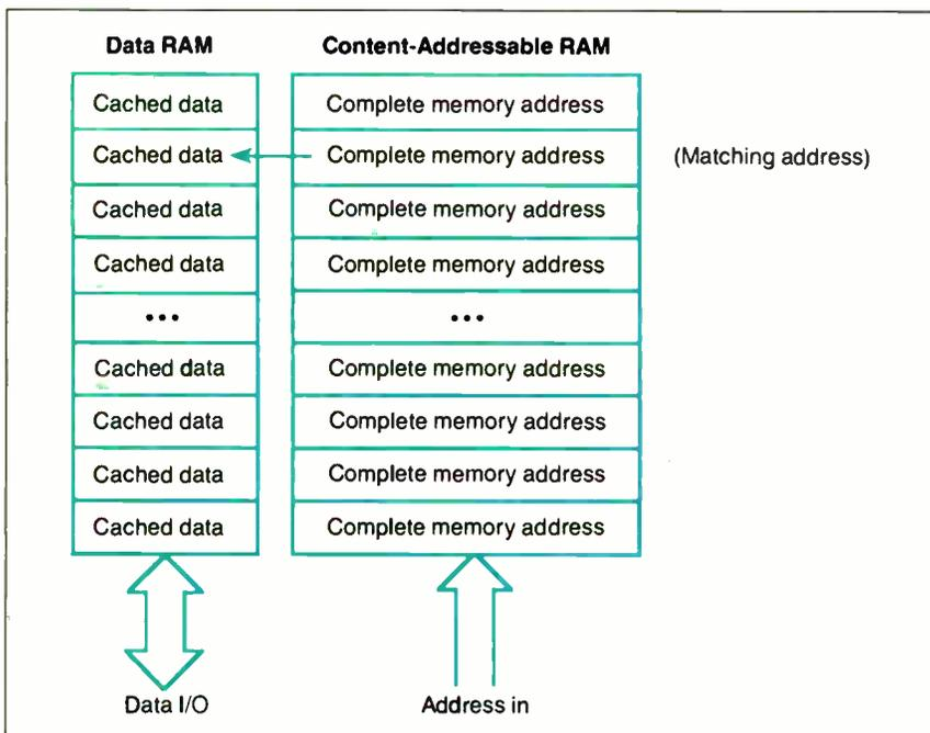
**Figure 1: A fully associative cache consists of a bank of data RAM and a content-addressable RAM containing the address where each data item came from. When each memory access occurs, the content-addressable memory is searched for the address of the required data. If it's found, the corresponding location in the data RAM can be used to complete the access. Since content-addressable memory is complex and expensive, fully associative caches are rare.**
