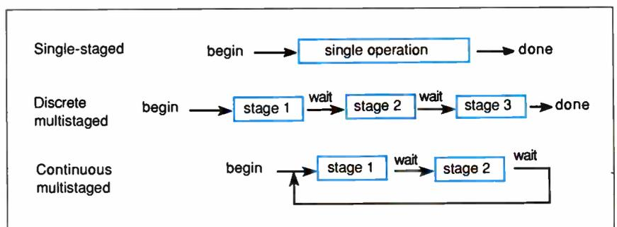
**Figure 4: ABIOS request types.** A single-staged ABIOS request completes immediately before returning to the caller. A discrete multistaged request is processed in stages with delays between the stages; control is returned to the caller until a hardware interrupt signals that a stage has completed. A continuous multistaged request starts a process—sometimes called a daemon—that loops forever between one or more stages.
