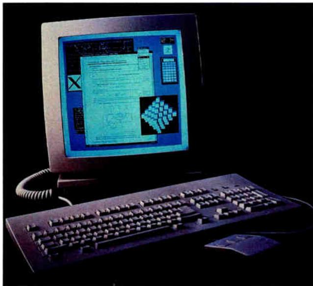
*The X Window-based NCD16 computer has an Ethernet link.*
