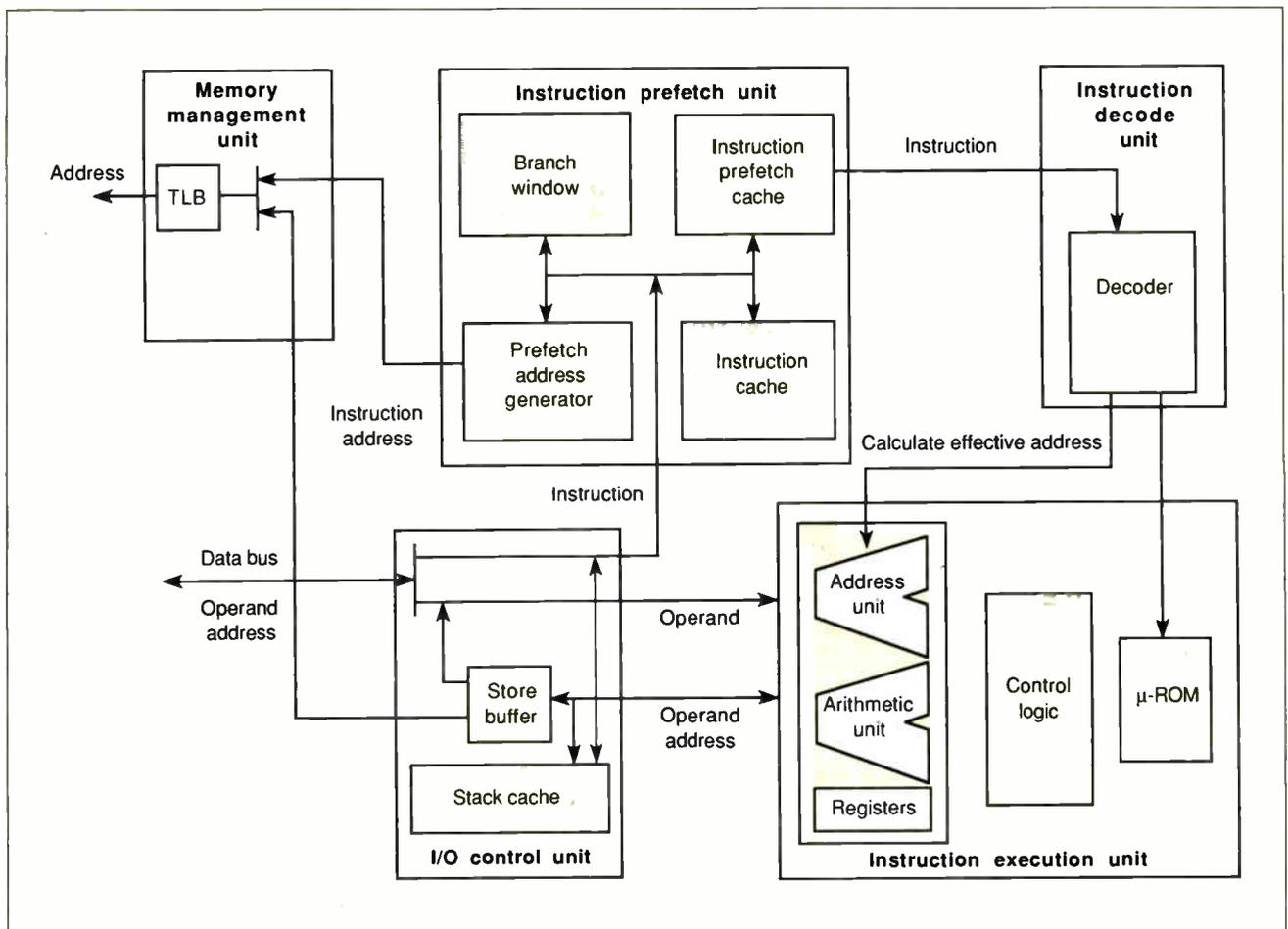
**Figure 5:** The Gmicro/200, the first generation of TRON CPUs, provides 32-bit addressing that is upwardly compatible with future 48-bit and 64-bit addressing modes. The internal structure of the Gmicro/200 provides for a very orthogonal instruction set. With the symmetry of operands, you can combine operands in any order.
