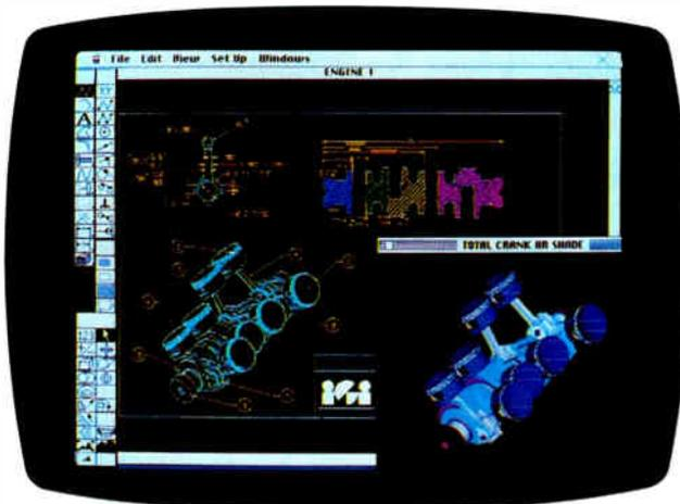
*In-CAD gives the Mac three-dimensional design, two-dimensional drafting, and solids modeling capabilities.*
