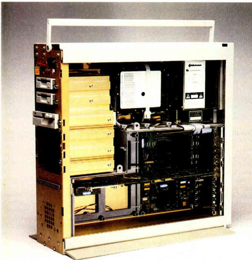
**Photo 1:** The inside of the CompuStar reveals the nature of the beast: plenty of expansion room and easy access to components.
