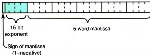
**Figure 1:** (a) A BCD floating-point number's internal storage (i.e., when the floating-point package is operating on the number), and (b) its external storage, as seen by the calling application. This format can handle numbers in the range  $\pm n \times 10^{\pm 16383}$ , where  $n$  is a decimal fraction with 20 digits of precision.
