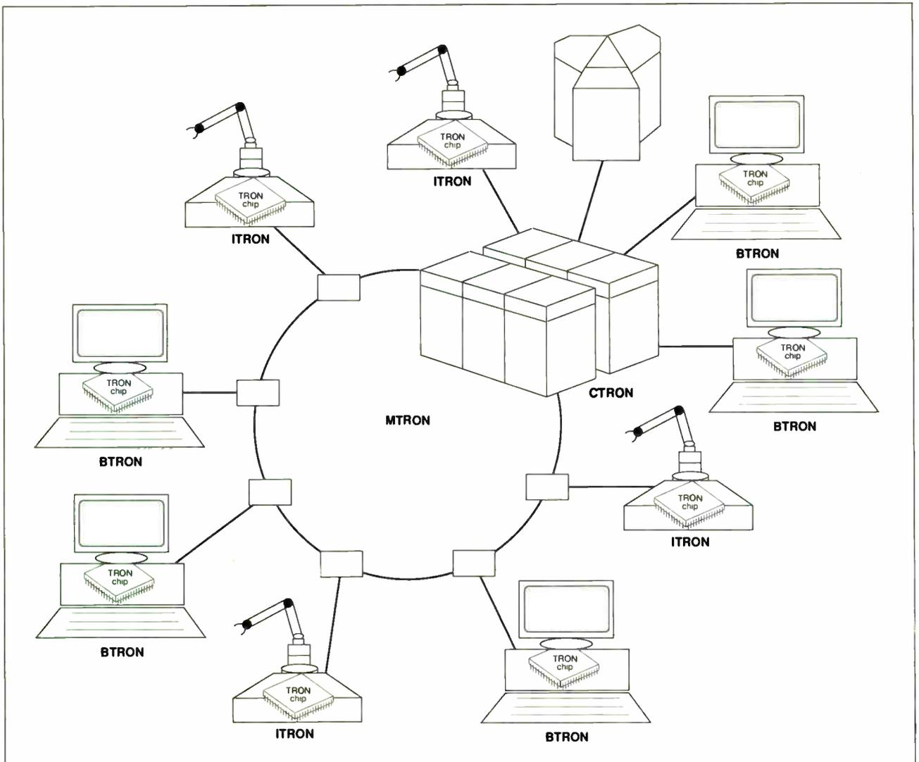
**Figure 1:** In the TRON world, BTRON workstations can communicate with ITRON industrial computers and share data with a mainframe through a CTRON file server. The network linking these and other "intelligent objects" together is MTRON.
