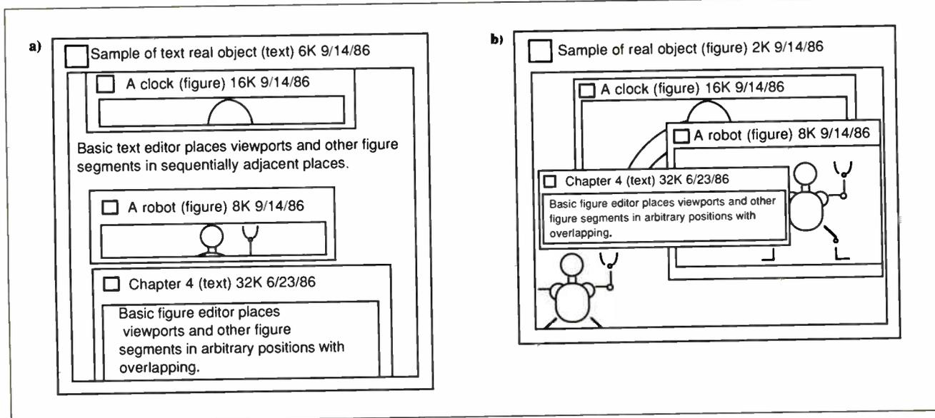
**Figure 3:** In BTRON, one-dimensional real objects (or text real objects) are stored sequentially (a), while two-dimensional real objects (or figure real objects) are arranged in a two-dimensional overlapped manner (b).
