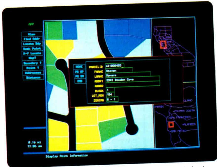
**Database Information Merged With Maps** MapInfo's desktop mapping package is the only software designed to directly tie dBASE files with maps. The parcels shown here were automatically shaded based on the data about each. A window is displayed that reveals the actual data behind a particular parcel.
