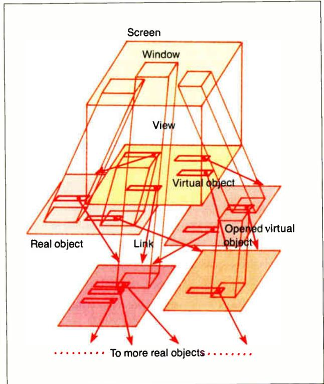
Figure 4: All BTRON data is stored in a real-object/virtual-object hierarchical structure. Real objects can be arbitrarily linked, and the virtual objects they contain can be nested to any depth.
