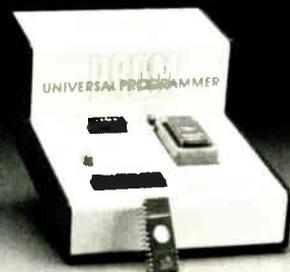
At \$495, Wintek's Universal EPROM Programmer is a low-cost and versatile tool for programming most industry-standard EPROMs (2716-27256). Since it can operate with an IBM PC, as well as stand-alone, the Programmer is ideal for use with PC-based microcomputer development software. Credit cards are welcome.
