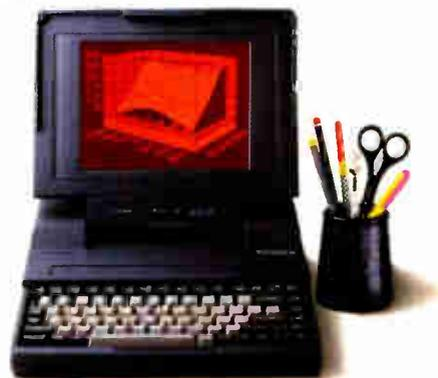
*T3100e: 12MHz 286 with 80287 coprocessor socket, internal half-length IBM slot, 20MB hard disk with 27msec access, 1MB RAM expandable to 5MB, gas plasma display, 1.44MB 3 1/2" diskette drive.*
