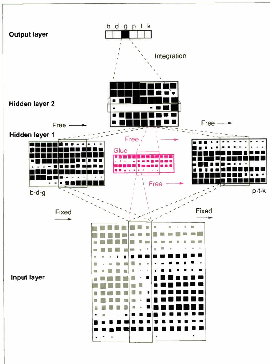
**Figure 2:** To form a modular network, you combine independently trained first hidden layers with a common second hidden layer. For greater accuracy, you can also provide free units (shown in red) for the combined first hidden layer.
