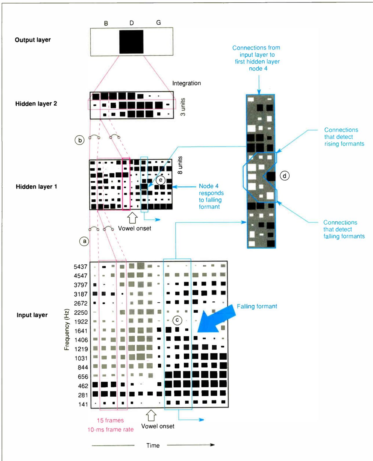
**Figure 1:** The left side (in red) shows the time-delay feature of the network. Three 10-millisecond input slices are combined to create activations in the first hidden layer (a). Activations in the second hidden layer (b) are created by combining five slices from the first hidden layer. The right side (in blue) shows the connections from the input layer to node 4 of the first hidden layer. When an input (c) matches the pattern of the connections (d), the node is activated strongly (e).
