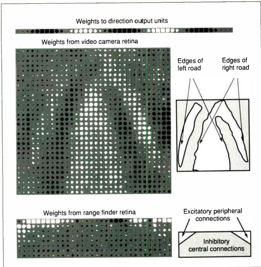
**Figure 6:** Pattern of weights projecting to and from a single ALVINN hidden unit after training on roads with a fixed width. This hidden unit acts as a filter for two types of road, one slightly to the left of center and one slightly to the right. The explanatory schematics on the right side of the figure highlight our interpretation of these weights.
