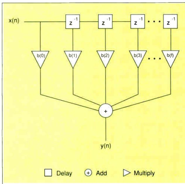
**Figure 3:** The digital filter structure shown here performs discrete convolution. The output  $y(n)$  is the sum of an input  $x(n)$  and  $k$  previous inputs, each multiplied by a coefficient ranging from  $b(0)$  to  $b(f)$ . Convolution can be used in a number of different applications, such as edge enhancement in image processing.
