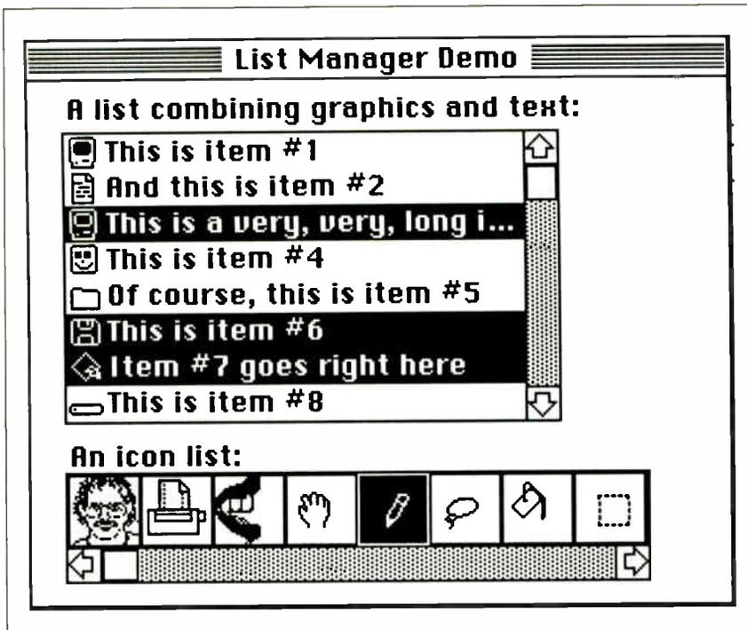
**Figure 1:** The sample application `ListMgrDemo` in action. The top window shows the output of `MyList.c`, which is a combination of scrollable text and graphics. Note that you can select more than one item in the list, as determined by the selection flags. The bottom window shows the output of `IconList`, which is a list of icons. This type of List Manager output makes it easy to implement a tool palette window for a painting or CAD application.
