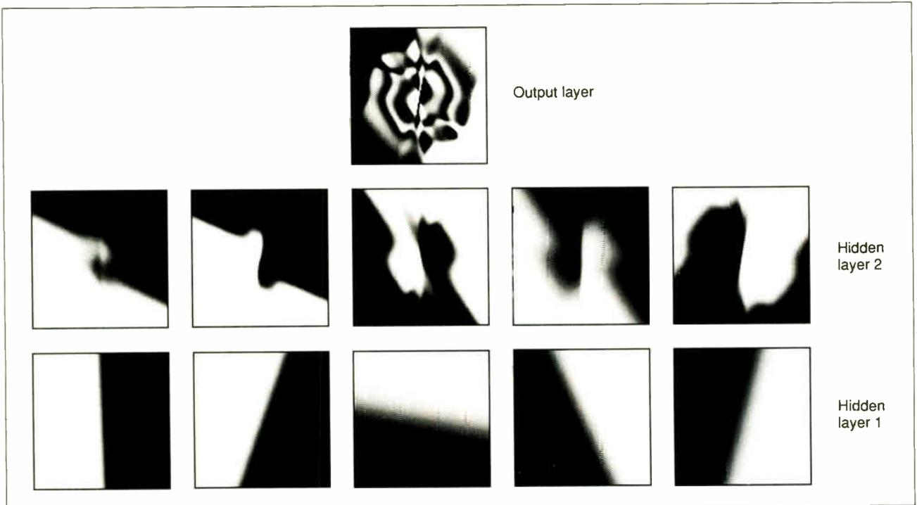
**Figure 4:** Response function plots for the units in the two-spirals network. Each plot shows the activation level of a single unit as the x,y input to the network ranges over the interior of the unit square. The topmost plot is for the output unit, and the plots below are for the five units in each of the two hidden layers. (Figure courtesy of Kevin Lang and Michael Witbrock)
