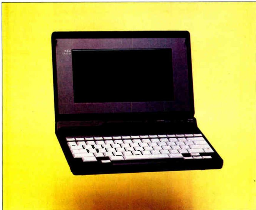
*The NEC UltraLite weighs in at only 4½ pounds but offers greater performance than an IBM PC XT.*
