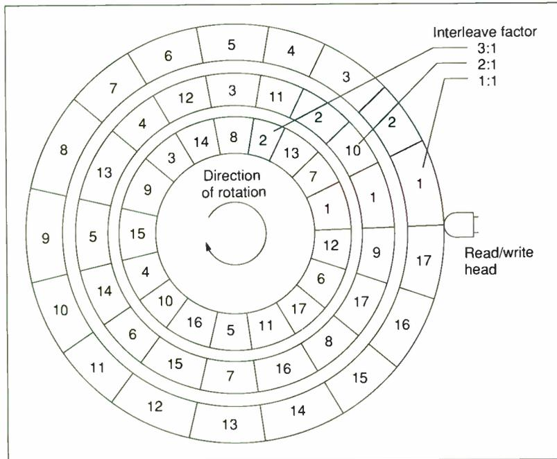
**Figure A:** Arrangements of sectors for different interleave factors. At 1-to-1 interleave, the sectors are numbered in sequence; at 2-to-1, sectors with consecutive numbers are separated by one other sector, and so on.
