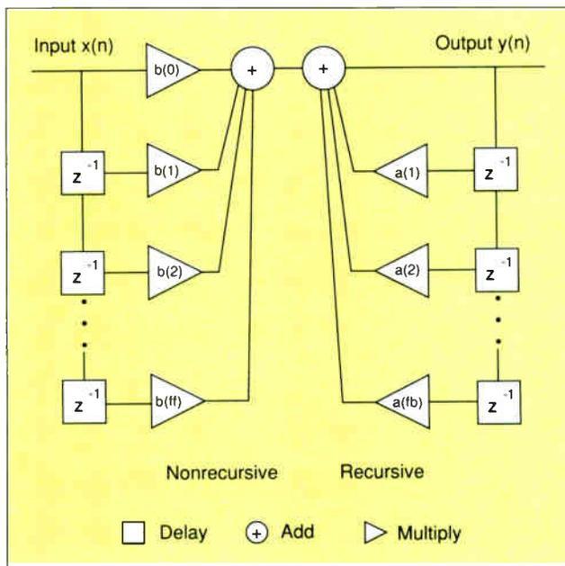
**Figure 4:** This diagram of a general digital filter combines a nonrecursive section on the left (like those in figures 2 and 3) and a recursive section, in which the output  $y(n)$  is multiplied by a series of coefficients  $a(k)$  to  $a(fb)$  and added to the next output. Such filters are useful because their behavior closely models that of analog systems.
