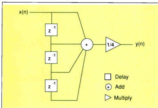
**Figure 2:** In this diagram, a filter (a four-sample averager) adds an input  $x(n)$  to the three preceding inputs (which have been delayed for this purpose) and divides the total by 4 to give the output  $y(n)$ . The effect of this averaging filter is to smooth out rapid deviations in the input signal, while leaving slower deviations, or low frequencies, relatively unaffected.
