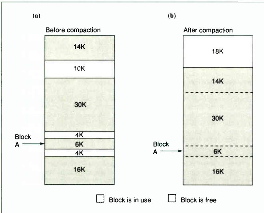
**Figure 2:** (a) If pieces of memory are randomly allocated and freed, the free memory is scattered throughout the heap in unusably small pieces. (b) If all the used blocks are moved to the bottom, the free memory percolates to a single large block.
