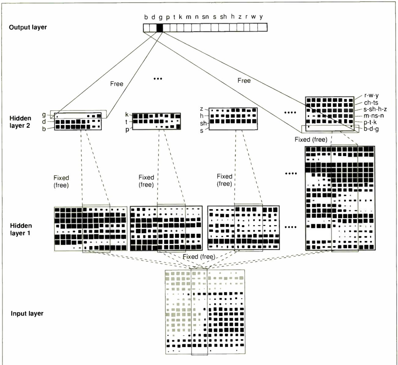
Figure 3: Modular construction of an all-consonant network.
