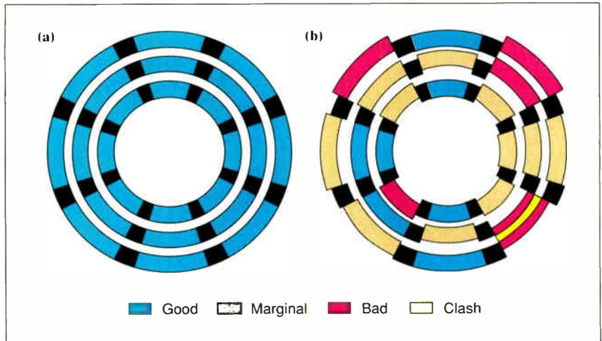
**Figure 1:** This diagram shows what happens when alignment drift causes the data portions of sectors to move out of line with the sector ID headers. (a) Before drift, there is good sector alignment; (b) after alignment drift, some sectors may even clash. (Figure courtesy of Prime Solutions)
