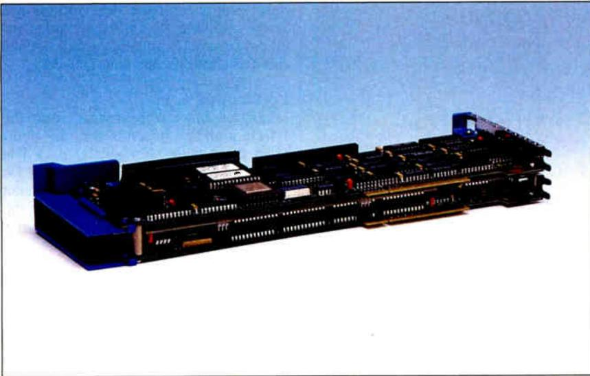
The Ultra Clipper UM1280, Pixelworks' bus-mastering coprocessor, brings enhanced graphics to MCA-compatible computers
