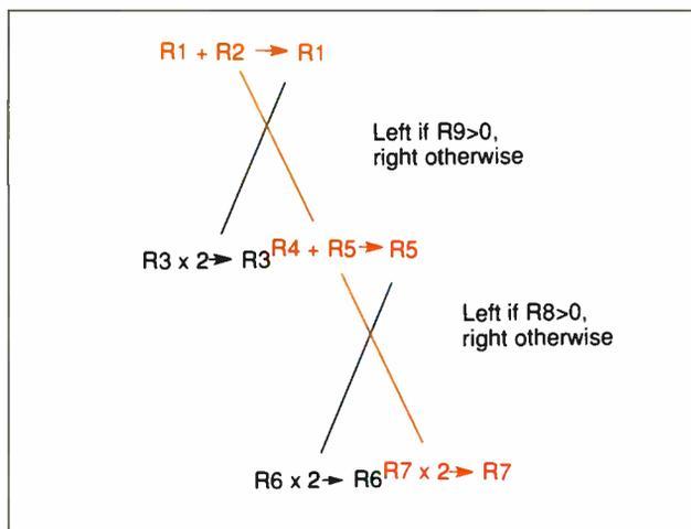
**Figure 1:** A fragment of code with five instructions and two branches. The trace-scheduling compiler chose the three emphasized instructions by predicting the computer's path at each of the branches.
