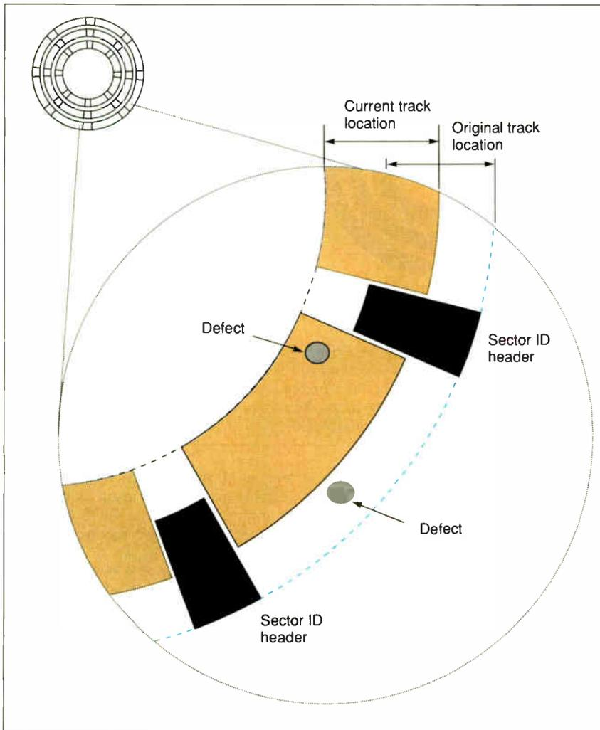
**Figure 2:** Alignment drift can cause "floating defects" not found in the manufacturer's defect map to appear in the data areas of a hard disk. The upper defect, originally harmless because it was between tracks, is now in the middle of the data, while the lower defect is now between tracks. The sector ID headers are now so far from the current track center that the sector may not be locatable. (Figure courtesy of Gibson Research)
