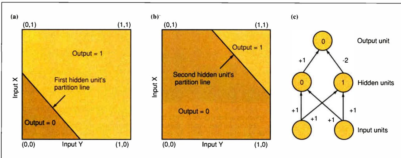
**Figure 1:** A network designed to solve the XOR problem. (a) and (b) The regions of input space for which the two hidden units are active. (c) The number inside each unit is its threshold. A unit turns on when its total input exceeds its threshold. The total input is equal to the sum of its input values (each input multiplied by the weight on the line).
