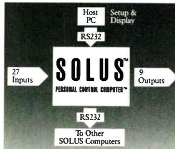
36 digital and analog I/O channels in a compact, intelligent, stand-alone unit that can be located anywhere. 8" wide, 2.25" high, 6.25" deep; 2 lbs; requires just 200 mA.
