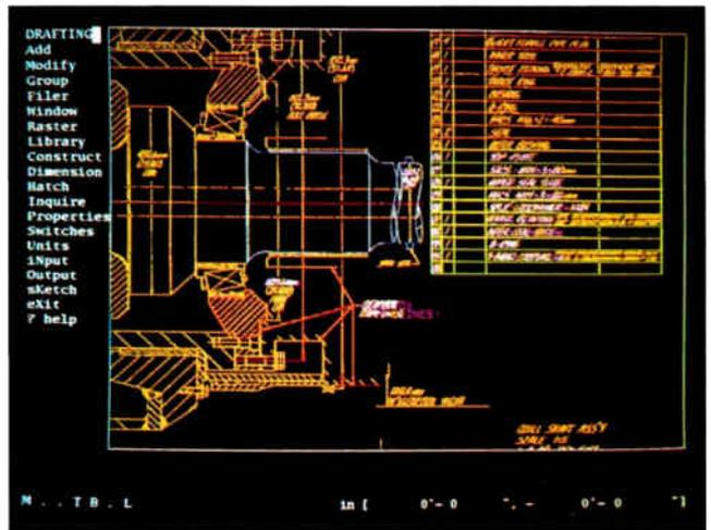
CAD Overlay lets you import scanned images to VersaCAD. The yellow lines are the scanned raster image, and the other colors are VersaCAD entities drawn over the scanned image.
