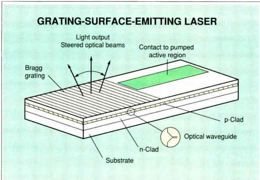
**Figure 3:** Grating-surface-emitting (GSE) laser structure. Light output is in the form of steered, focused, narrow optical beams from the surface of the diffraction grating. Current from the contact to pumped active region stimulates optical emission in the optical waveguide.
