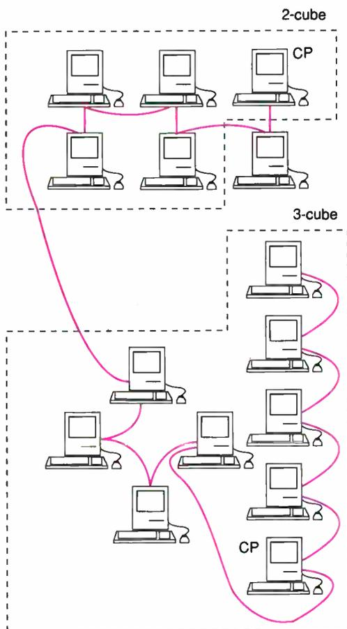
**Figure 2:** Sample Mac-Cube hypercubes on an AppleTalk network. Note that there are 2-cube and 3-cube systems on the same network and that the lone (shaded) user is undisturbed except for the network loading added by the Mac-Cubes. Also, the Macs that make up each cube do not need to be contiguous.
