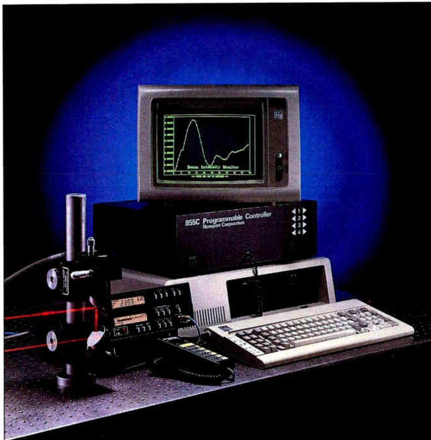
**Photo 3:** National Instruments software, controlling instrumentation for testing lasers. Notice the power meter and stage-positioning system integrated with an IBM PC under the control of LabWindows. The CRT display shows the laser-beam intensity. (Photo courtesy of Newport Corp.)
