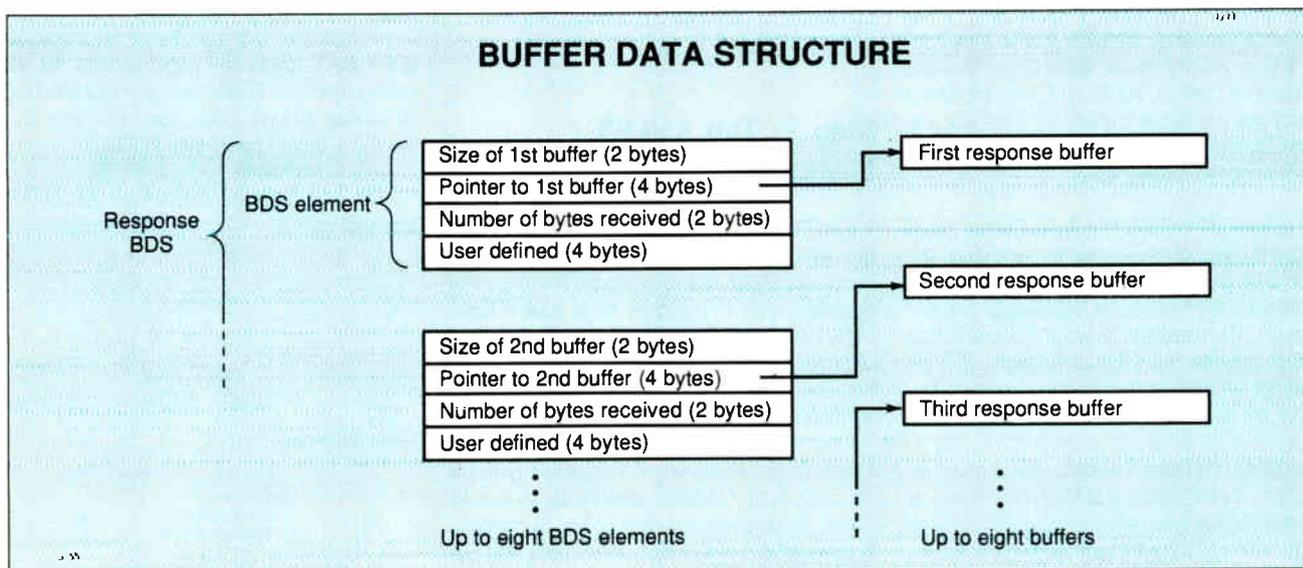
**Figure 2:** The response buffer data structure (BDS) tells the AppleTalk Transaction Protocol where incoming responses can be placed. A single response BDS can consist of up to eight BDS elements of 12 bytes each. A BDS element governs a response buffer, where the actual response data goes.
