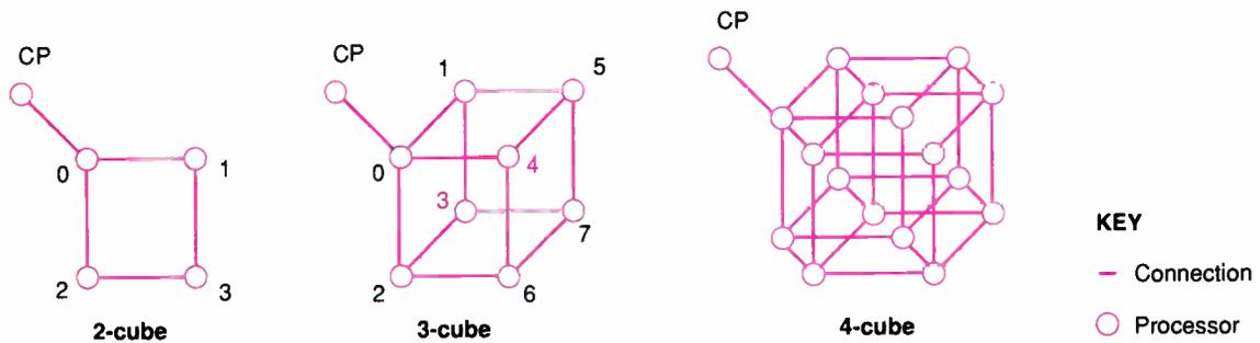
**Figure 1:** Hypercubes of dimensions 2, 3, and 4. Each cube has  $2^p$  processing nodes and a single control processor, and each node is connected to  $p$  other processors. Thus, a 2-cube has four processing nodes and one control processor, and each processing node is connected to two other nodes.
