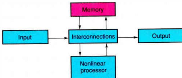
**Figure 1:** Holograms provide memory storage and interconnections, while spatial light modulators are commonly used for input, output, and processing units.
