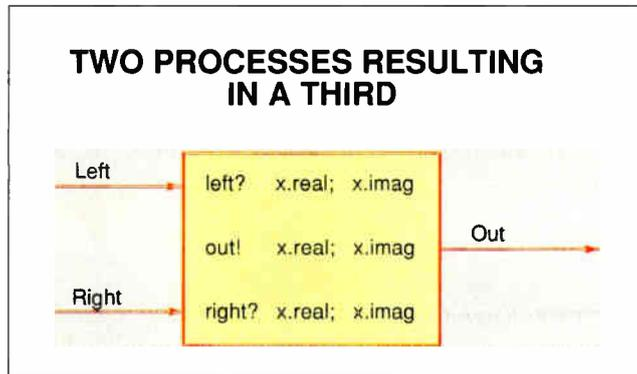
Figure 2: A process diagram of two input streams multiplexed into a single output stream. The Boolean value FALSE on channel shutoff will terminate the program.
