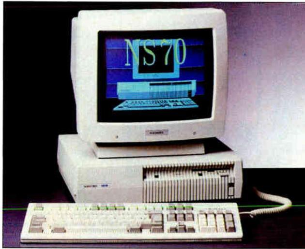
Normerel's 25-MHz NS70-25 has an MCA bus.
