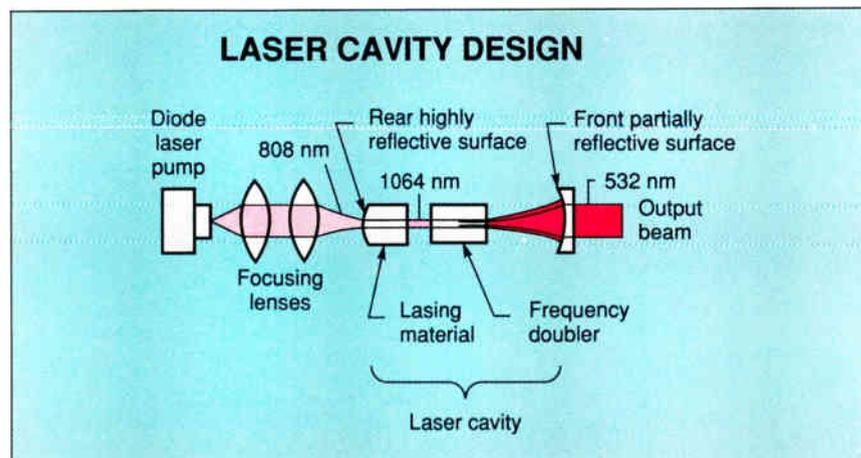
**Figure 3:** A CAD-generated, diode-pumped, frequency-doubled laser cavity. It illustrates the conversion of low-quality infrared diode-laser-pump light to high-quality infrared (1064 nm) and visible (532 nm) light in an all-solid-state design.
