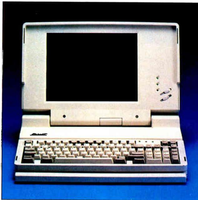
*Copam's 12-pound AT laptops include VGA graphics, nickel-hydride batteries, and a 20-megabyte hard disk drive.*
