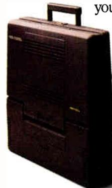
*T5200: 20MHz 386 processor, 2 internal IBM compatible expansion slots, VGA display with external VGA monitor port, 40MB or 100MB hard disk, 2MB RAM standard expandable to 8MB, 1.44 MB 3½ diskette drive.*
