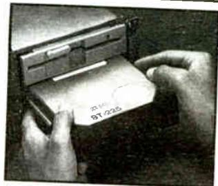
You install the 1.2 meg, 5 1/4" floppy disk drive, learning disk drive operation and adjustment. Later, you improve your data storage capacity dramatically by installing this powerful 20 meg hard drive.
