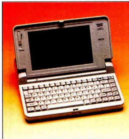
At the heart of the 1100 FD is an 8-MHz NEC V20 (8088-compatible) CPU. There are also 640K bytes of RAM, a single 3½-inch 720K-byte floppy disk drive, and serial and parallel ports. The 9-inch-diagonal screen offers a resolution of 640 by 200 pixels.
