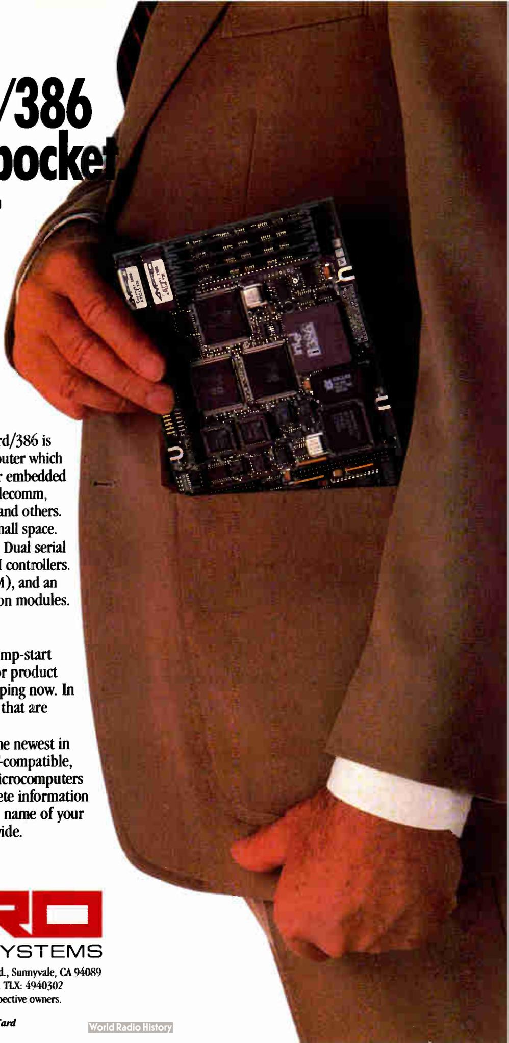
**Big power. Small package.** Little Board/386 is a complete, 32-bit, 20MHz, 80386 computer which occupies just 5.75" X 8". It's perfect for embedded applications such as instrumentation, telecomm, network servers, data acquisition, CAM and others. Anywhere that you need big power in small space.
