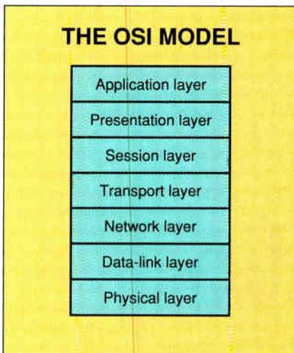
**Figure 1:** The OSI Model consists of seven protocol layers that allow dissimilar computers and applications to communicate and share data. Wireless LANs concern themselves with the Physical and Data-link layers of the model, which describe the physical nature of the connection between two machines and an error-free method of data transmission over that connection.
