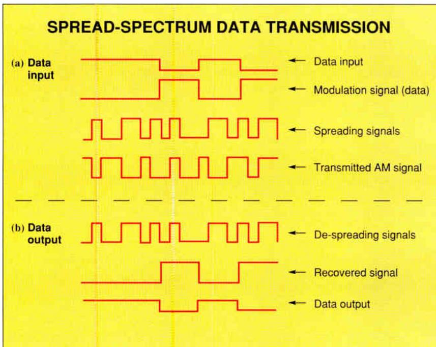
**Figure 3:** (a) To encode data in a direct-sequence spread-spectrum system, you convert the input data to a usable form, multiply this by the spreading code, and send the results to the AM transmitter. (b) To decode the signal, you multiply it by the spreading code and convert the results into binary 0s and 1s.
