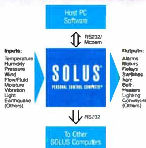
36 digital/analog input/output channels are compatible with standard sensors and output devices. SOLUS can be located on site, or remotely via modem.
