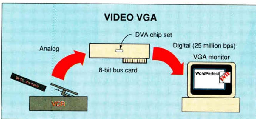
A ribbon cable connects the DVA-4000 to the feature bus of the existing VGA card. "Smart windows" can then display real-time video images and allow you to freeze, resize, and change colors in individual frames.
