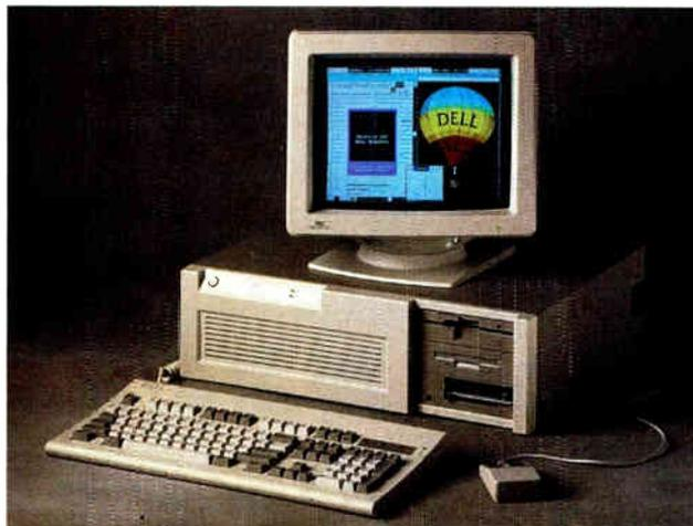
*Dell's 320LX is one of the first 386SX systems with a 20-MHz clock speed.*
