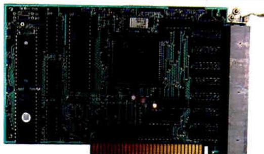
The PCSS-8I is GTEK's most popular intelligent serial I/O card with compact RJ-11 telco jacks. It provides 8 serial channels for PC/XT/AT/PS2-286 and is DOS Compatible. The PCSS-8I has 32K of *Dynamemory*, user upgradeable to 128K bytes. Driver available for SCO™ XENIX®.
