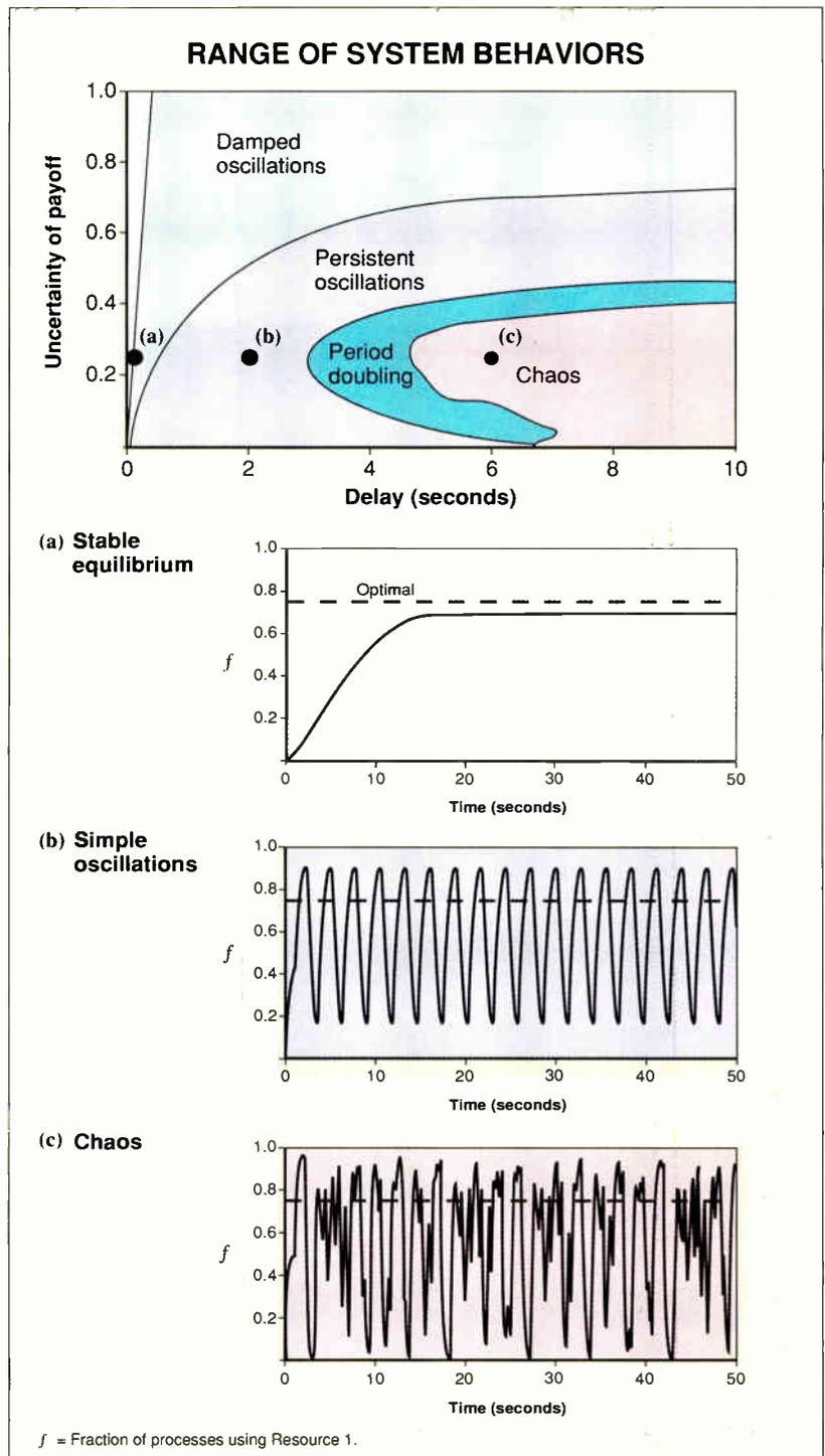
**Figure A:** The range of behaviors for a computational ecosystem in which processes choose between two resources. In the unshaded region, the system does not oscillate, but relaxes to equilibrium. Typical behaviors for the fraction of processes using Resource 1 as a function of time are shown for three particular points: (a) relaxation approaching a stable equilibrium, (b) simple persistent oscillations, and (c) chaotic oscillations. The dashed line represents optimal resource allocation.
