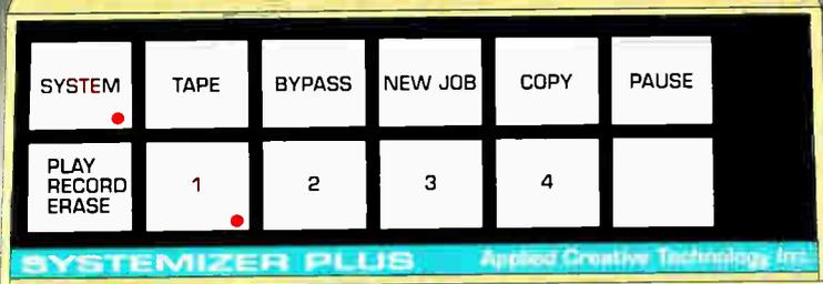
Several models available. The **Systemizer Plus**® shown above is an externally mounted networking module. Because it's self-contained and requires no software in the computer, it can work with practically any computer, operating system and application program.
