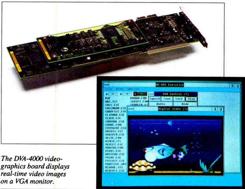
The DVA-4000 video-graphics board displays real-time video images on a VGA monitor.
