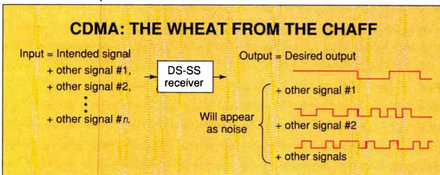
**Figure 4:** The code-division multiple-access method of data recovery separates overlapping signals on the same carrier frequency. Spread-spectrum systems use the spreading code for this purpose. This ensures that only one signal produces valid data. Other signals produce noise when decoded at the receiver.
