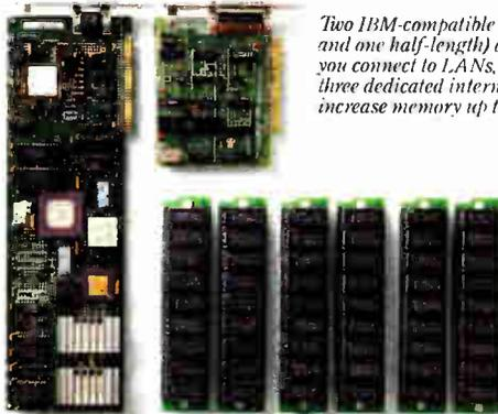
*Two IBM-compatible expansion slots (one full-length and one half-length) and an internal modem slot let you connect to LANs, mainframes and more. Plus, three dedicated internal expansion slots let you increase memory up to 13MB.*
