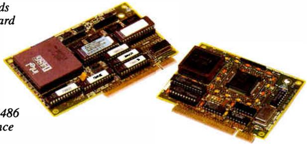
**Photo 2:** *The Premium 386SX/16's proprietary 32-bit memory architecture gives its processor cards a performance edge over ALR's PowerFlex, but at a much greater price. Each card has room for 4 MB of SIMM-mounted RAM; additional memory slots let you expand memory to 16 MB, or to 36 MB with the 486/25 module installed.*
