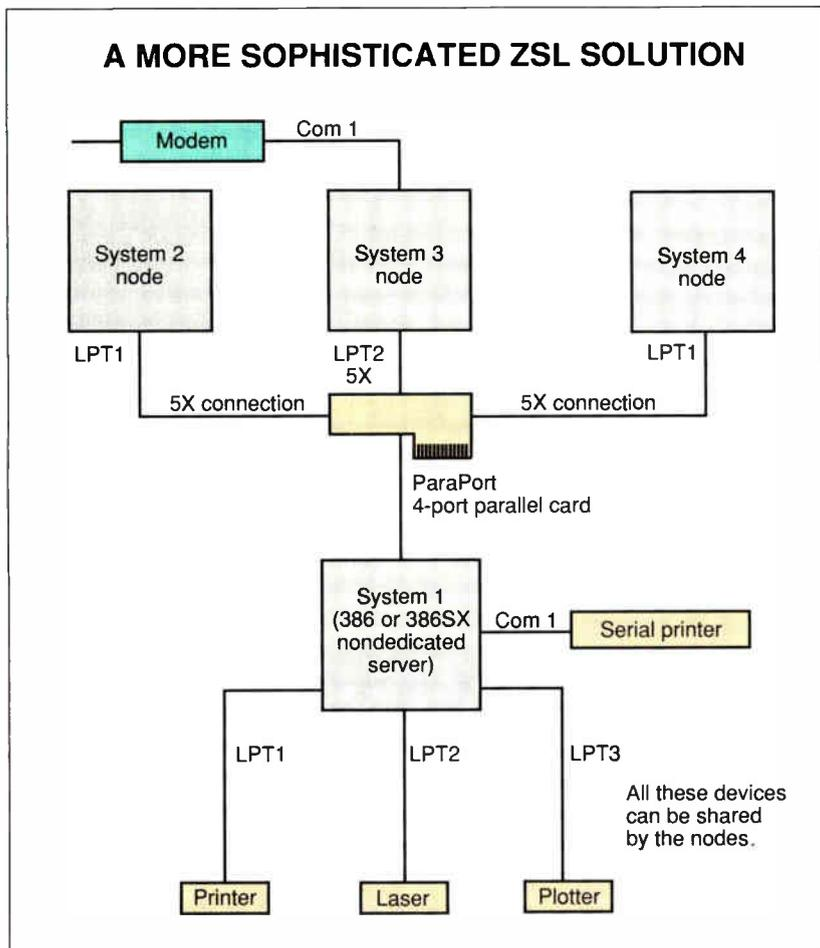
**Figure B:** In this LANLink 5X/PC-MOS hybrid network, System 1 is running single-user PC-MOS. To give the nodes access to the server, Post installed a ParaPort card (four parallel ports) in the server. This system provides full file transfer, file-sharing, and program-execution capabilities.
