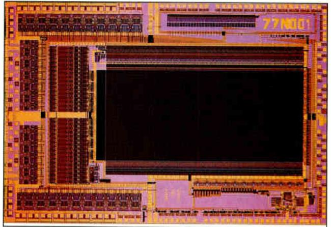
**Photo 3:** Intel's nonvolatile ETANN chip provides permanent true analog weight storage without refresh or battery backup. Its 10,000 multipliers and 20,000 analog EEPROM cells take up the bulk of the dye area.
