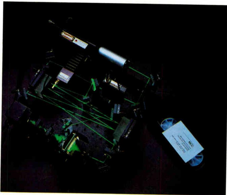
*A prototype holostore device. Since the beam falls within the green range on the visible spectrum, you can trace its progress through the device (see figure 3 for more details).*
