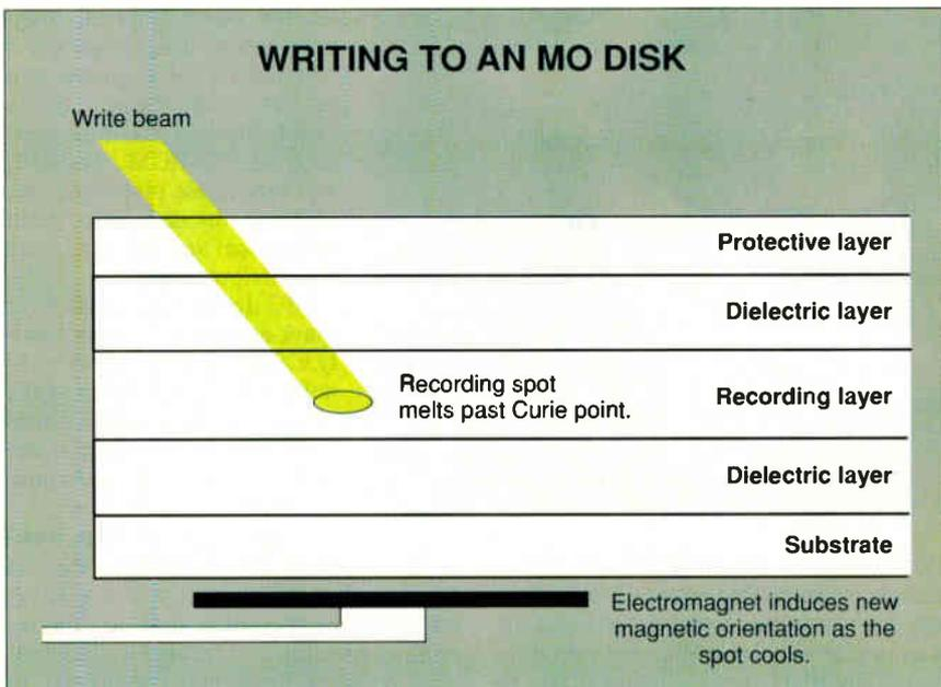
**Figure 2:** Writing a bit to a magneto-optical disk means setting the magnetic orientation of a recording spot. The write laser melts the spot, while the underlying magnet produces a field with the new orientation of the spot. As the spot cools, it assumes this new orientation.
