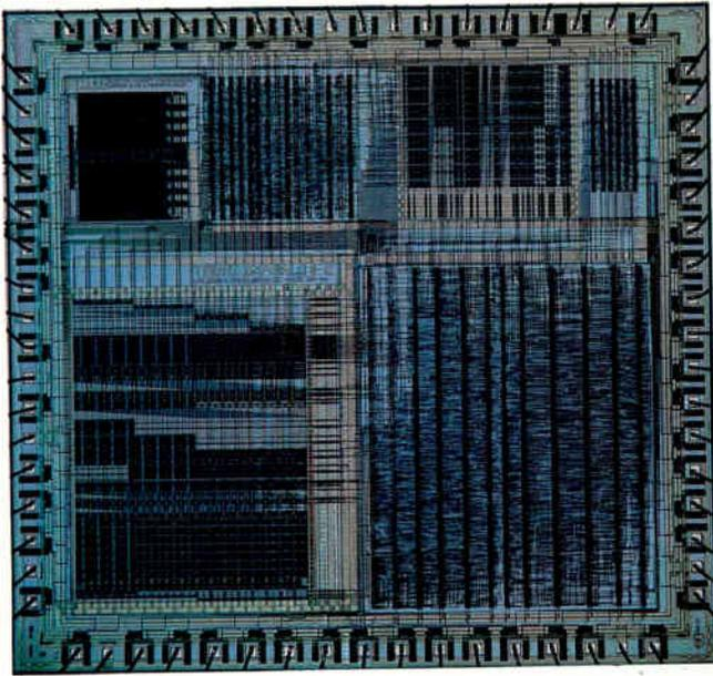
**Photo 1:** The FC110. On the bottom left of the die, the ALU path is set up so it will do 8-, 16-, or 32-bit operations. The large block at the lower right contains the hardware to implement the special instruction set that performs fuzzy-logic operations.
