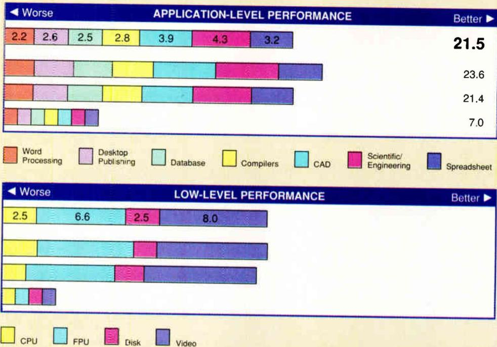
For application and low-level benchmarks, results are indexed and show relative performance; for each individual index, an 8-MHz IBM PC AT running MS-DOS 3.30 = 1. For all benchmarks, higher numbers indicate better performance.
