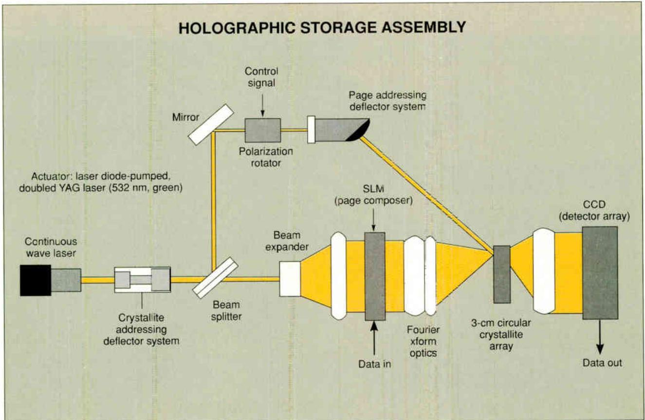
**Figure 3:** The laser source for the holostore prototype is a compact, doubled, diode-pumped YAG laser with 80-milliwatt output at 532 nanometers. The beam splitter splits the laser into separate data and reference beams and steers them onto the surface of a crystallite to store (or retrieve) a page of data.
