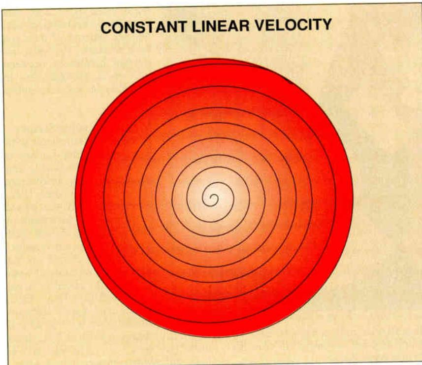
**Figure 1:** In constant linear velocity (CLV) recording, data is arranged in a single spiral track with a uniform density of bits. This lets you pack the most information possible onto the disk. The speed of the disk varies between the outer and inner edges—the closer the read head gets to the outer edge, the faster the disk spins. Data is located by its temporal position, measured in minutes and seconds. Each second consists of 2K bytes of data.
