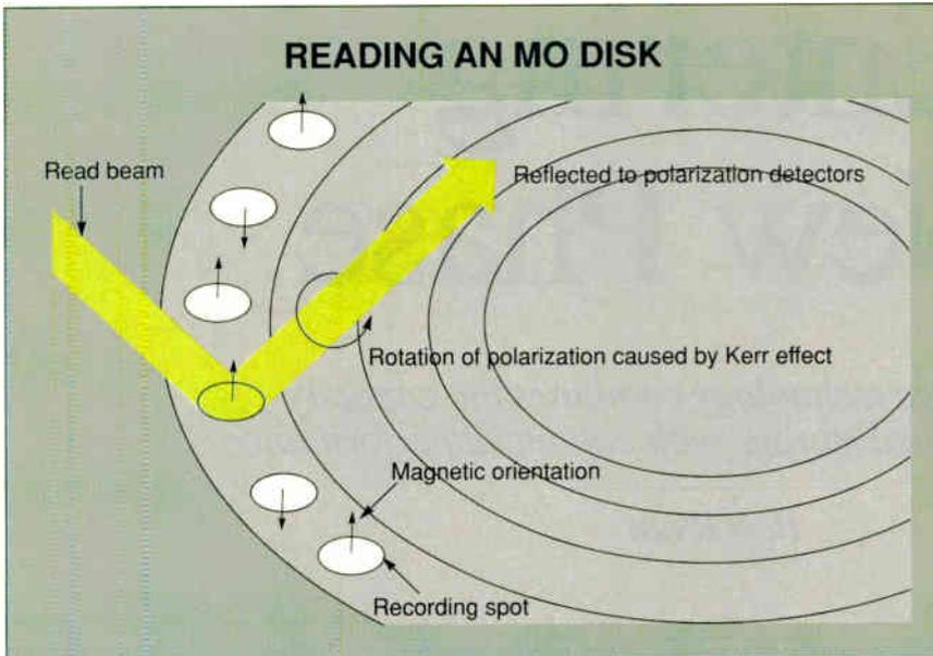
**Figure 1:** Every recording spot on a magneto-optical disk has a magnetic orientation that corresponds to either a 0 or a 1. To determine the orientation of a spot, the read system bounces a low-power laser off the spot. The direction of the polarization rotation put on the reflected beam by the spot's magnetic orientation reveals whether the spot is a 0 or a 1.
