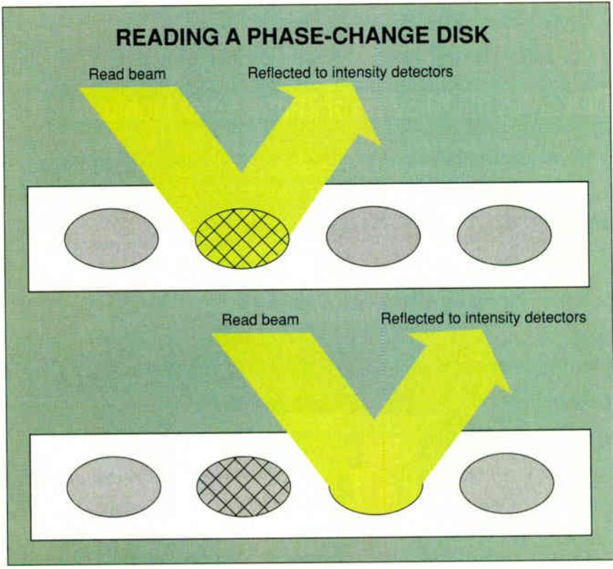
Figure 4: Unlike magneto-optical drives, which must detect small changes in the read beam's polarization, phase-change systems read information by detecting the relatively large differences in the reflectivity of the amorphous and crystalline states.
