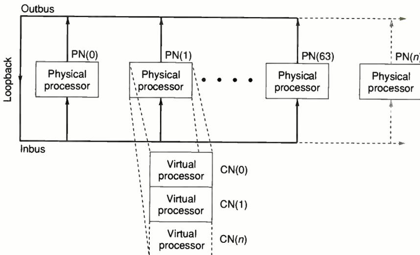
**Figure 1:** Adaptive Solutions' architecture can be extended in two directions. Each chip has 64 processor nodes, and additional chips can be added to provide arrays of hundreds of processors. Virtual processors, called connection nodes, are mapped to each physical processor, creating thousands of neural-network nodes. Loopback techniques and broadcast from any processor allow arbitrary interconnection of all nodes.
