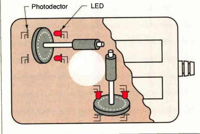
**Figure 2:** As with an electromechanical mouse, a rubber ball inside an optomechanical mouse drives the encoders. In this case, however, LEDs shine through holes in the encoders. The optical encoding scheme eliminates wear on the encoders.
