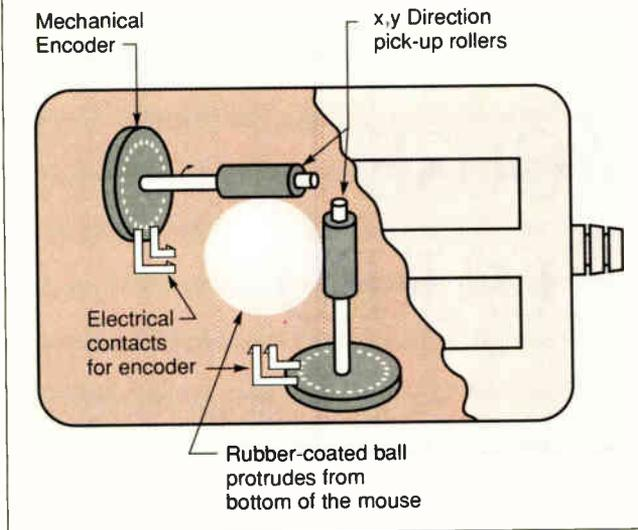
**Figure 1:** In an electromechanical mouse, a rubber ball drives the encoders, which make and break electrical contacts.
