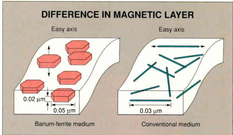
**Figure B:** Since the barium ferrite particles (top) are magnetized vertically, there is a sharp magnetic transition between the particles, even at high densities. This is in contrast to the conventional oxide particles (bottom).
