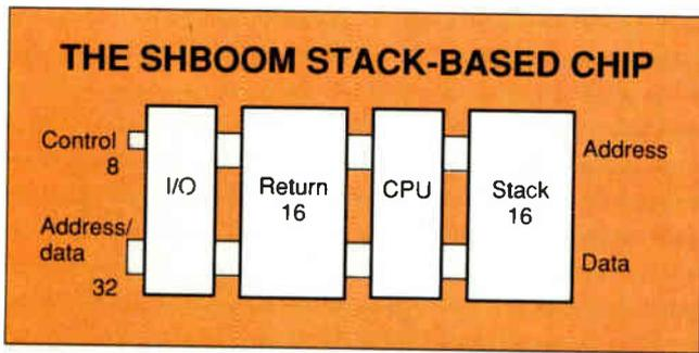
**Figure 2:** *ShBoom* has separate 32-bit internal buses for address and data. Both access the CPU, its two stacks, and the I/O processor. These buses are multiplexed into a single 32-bit external bus with DRAM and I/O control signals.
