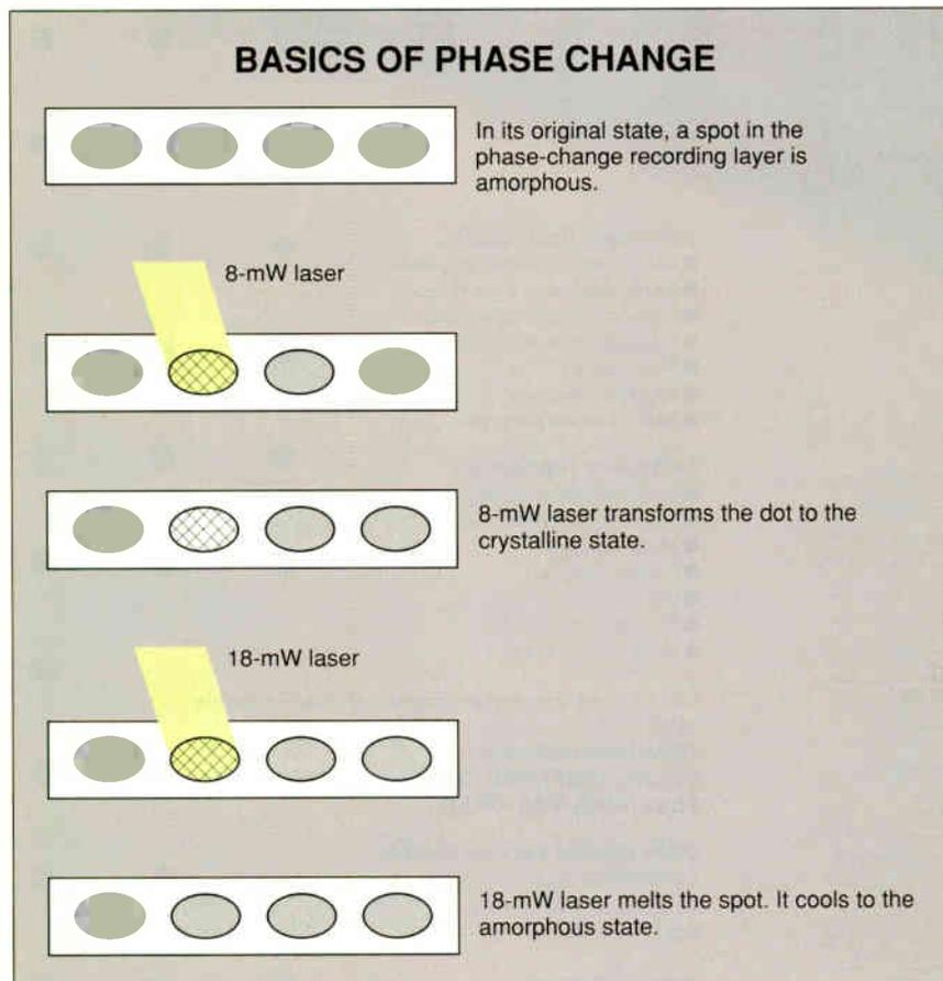
**Figure 3:** The remarkable property of phase-change media to change from amorphous to crystalline at one energy level and from crystalline to amorphous at a higher level enables the realization of direct optical overwrite.
