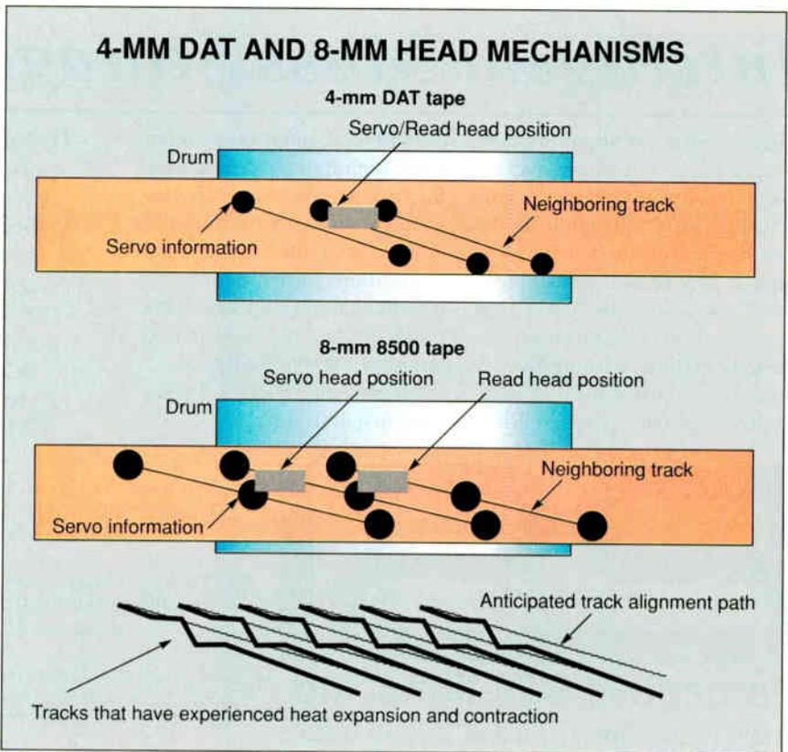
Figure 2: An 8-mm tape drive's separate servo and data heads can have trouble following distorted tracks. The 4-mm DAT drive's integrated servo and data heads track more faithfully.
