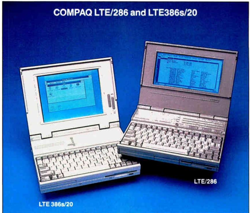
Both of the Compaq notebook machines bear a striking family resemblance, but beneath the exterior, the LTE 386s/20 has a completely new design that incorporates Intel's 20-MHz 386SX. The LTE/286 uses a 12-MHz 80C286 processor. Both accept a math coprocessor and include floppy and hard disk drives. The 386s/20's 2.2-inch-high case—which is slightly thicker than the LTE/286's case—makes that notebook the tallest machine in the group. Both Compaqs are relatively light and easy to carry.
