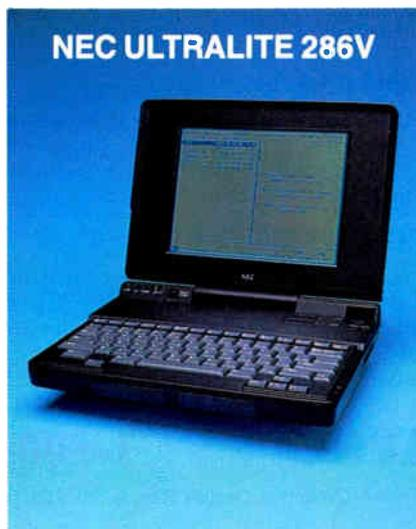
Delete keys double as the F11 and F12 keys. Function key combinations can also change the processor speed, disable the speaker, power down the disk drive, turn off the backlighting, or place the unit in full standby mode. You can also set power-conservation time-outs by invoking the setup program.
