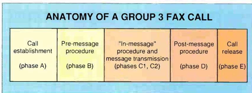
Figure 2: The CCITT T.30 specification divides a fax call into five phases.
