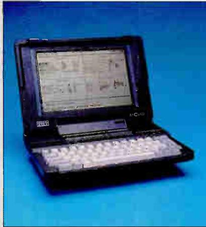
768K bytes of RAM (only 640K bytes is accessible), the 1-MB internal RAM disk, LapLink III, and DOS 3.2.
