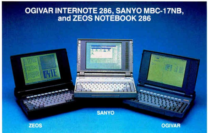
The units fold into a compact 7-pound shell. All three appear to be solidly constructed, durable machines. A row of indicator lights lies on the main unit, just below the screen, remaining visible when the screen is folded down. A handle pops out from the front of the unit for easy carrying.
