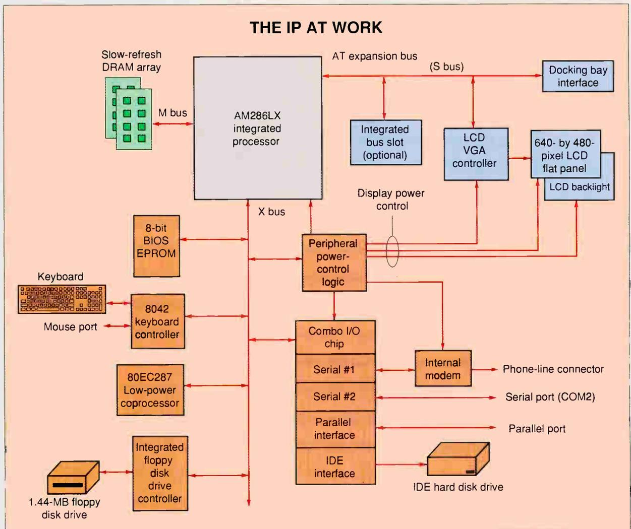
**Figure A:** The Am286LX communicates with the outside world via three buses. The M bus accesses system RAM, the X bus talks to motherboard peripherals, and the S bus communicates with ISA peripherals.
