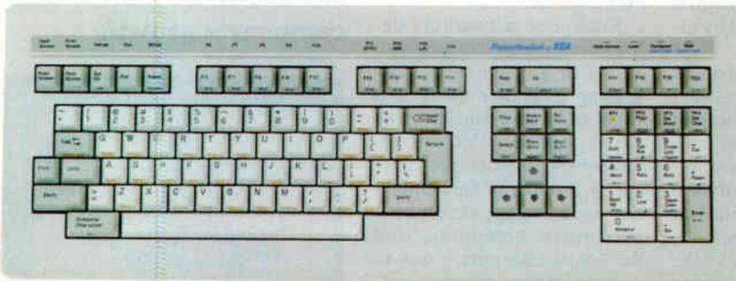
The *PowerStation* keyboard gives you the control you need for key-by-key emulation of a DEC terminal. The *PowerStation* is an exact VT200/VT300 layout keyboard that plugs into your PC. The *PowerStation* brings VAX applications to your PC without having to hunt for re-mapped keys.
