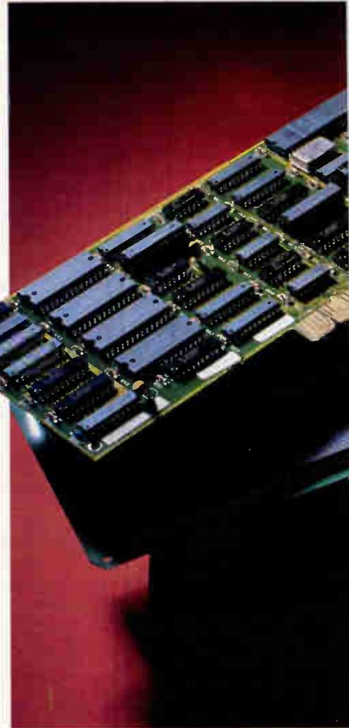
priate physical medium by way of a jumper block. The default configuration is thin Ethernet.
