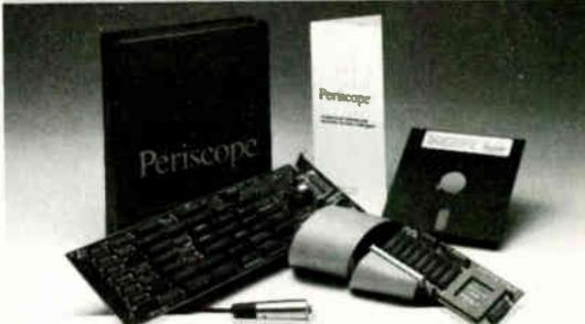
Real-time Periscope Model IV, shown with new 33MHz board and 486 pod.
