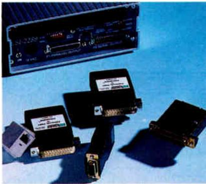
MultiSpool's adapters allow any combination of serial and parallel connections among its input channels.
