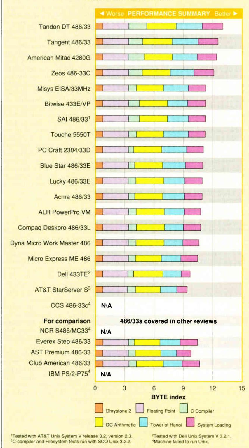
The Unix benchmarks, ranked by cumulative index scores. We tested each system using SCO Unix System V version 3.2.0. For all results, an Everex Step 386/33 running SCO Xenix 2.3.1 = 1.
