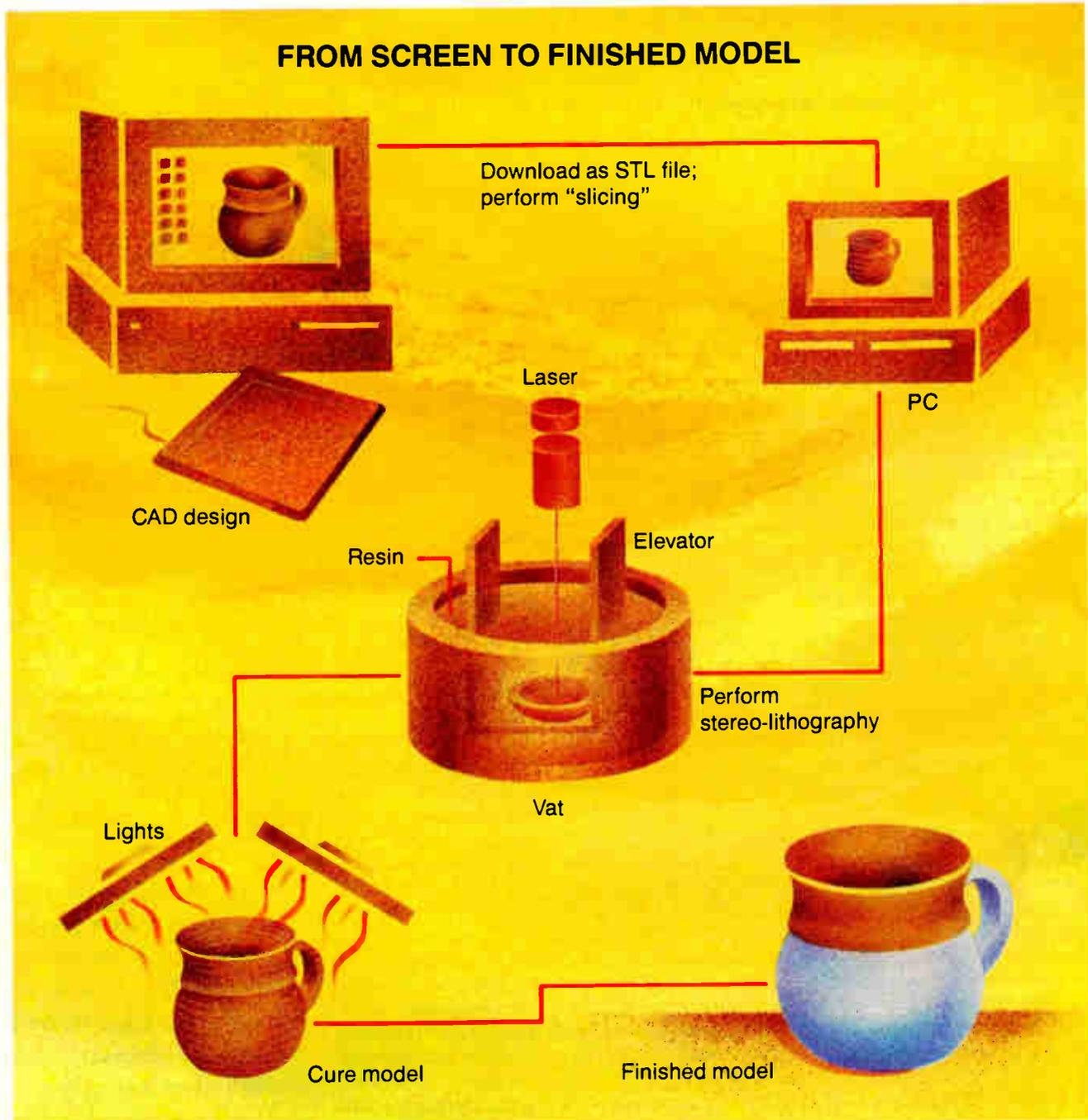
*Rapid automated prototyping, a technology that is now available on microcomputers and workstations, lets you build prototypes from solid-model CAD drawings—just as you use a printer to create 2-D printouts of screen images.*
