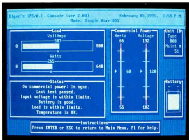
**Screen 2: LanSafe A.I.+ control software for Elgar's IPS/A.I. shows instantaneous values for incoming voltage and line frequency, outgoing power and equivalent volt-amperes, battery level, and other parameters.**
