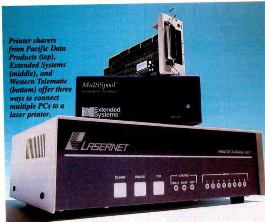
Printer sharers from Pacific Data Products (top), Extended Systems (middle), and Western Telematic (bottom) offer three ways to connect multiple PCs to a laser printer.
