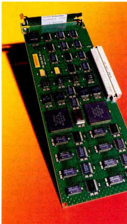
*Storm's PicturePress accelerator card and software compress Macintosh-based image files using three types of compression schemes.*
