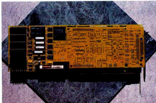
*The CEK101a add-on card for the IBM PC can turn your computer into a satellite communications receiver and is capable of processing any kind of data received by the host.*
