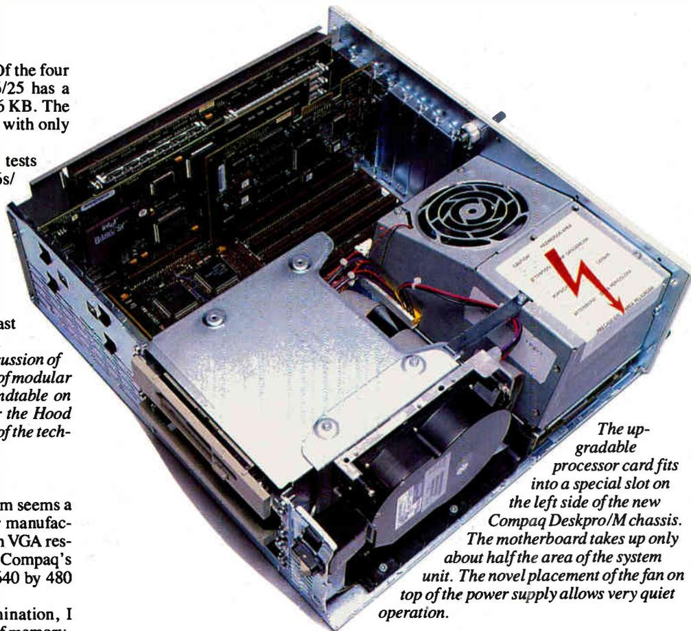
The up-gradable processor card fits into a special slot on the left side of the new Compaq Deskpro/M chassis. The motherboard takes up only about half the area of the system unit. The novel placement of the fan on top of the power supply allows very quiet operation.
