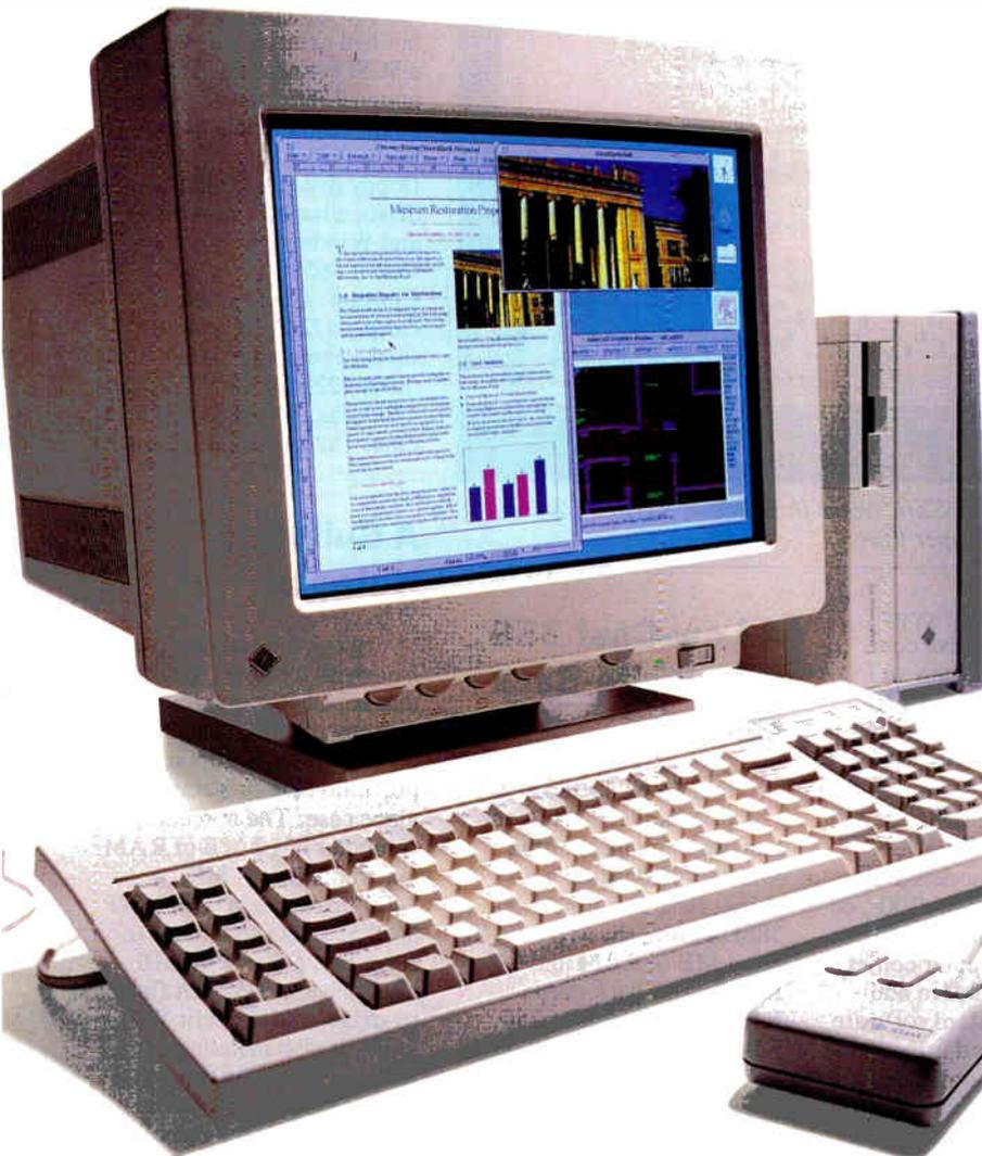
*The new \$11,995 SPARCstation IPX is the lowest-cost accelerated graphics workstation we've ever offered. Its GX accelerator is on the motherboard, freeing up an expansion slot. Its 40-MHz integrated integer/floating point processor performs up to 24.4 SPEC-marks. (Color monitor available at additional cost).*
