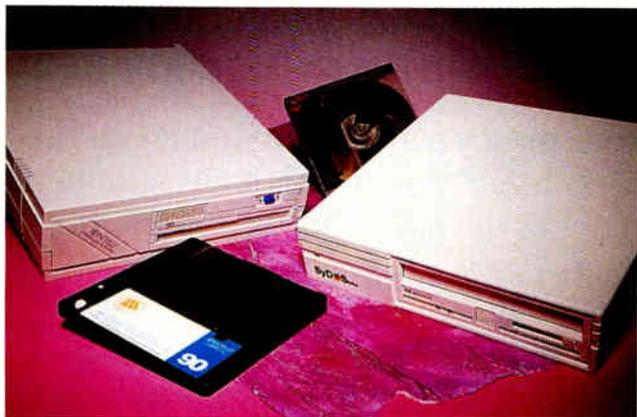
**A** removable-cartridge drive is a cross between a floppy drive and a hard drive, giving you the convenience of a floppy disk with the speed and capacity of a hard disk. The SyDOS 88 and Iomega's **Transportable 90** are the latest offerings from the industry leaders.
