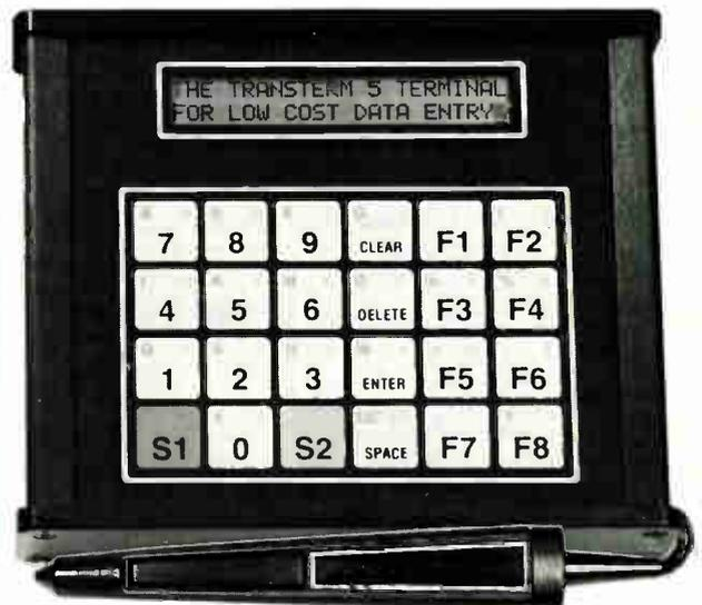
The TransTerm 5 is a work station data entry/display terminal for on-line shop floor data collection into PC/AT based systems. The unit is one of a family of such terminals which feature LC displays for operator prompting and data entry via a membrane keyboard or an optional barcode wand (Code 39). A multi-terminal polling controller (up to 250 stations) and a dBASE III+ compatible software package are also available. System costs below \$300.00 per station. Call for info.
