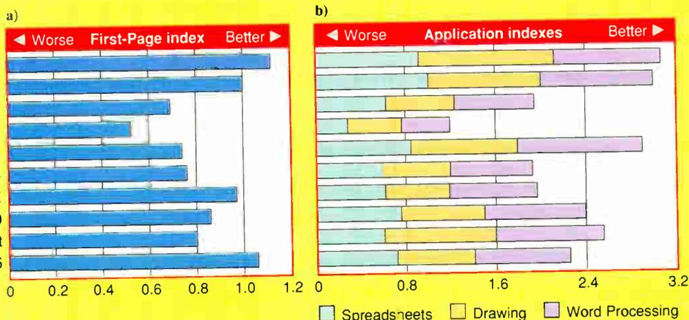
*From click to klunk: (a) The first-page index tracks printer performance on a single text page. We started timing when the printer first received PostScript commands and stopped timing when the page fell into the output tray. Expect this type of performance for memos and simple business correspondence.*
