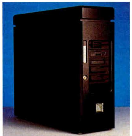
support 512. Its 64 KB of second-level cache (expandable to 256 KB) enhances the 8-KB on-chip cache and FPU. It has a SCSI mirroring hard drive controller with caching and 1 MB of RAM (expandable to 32 MB) and a 300-MB tape backup unit.
