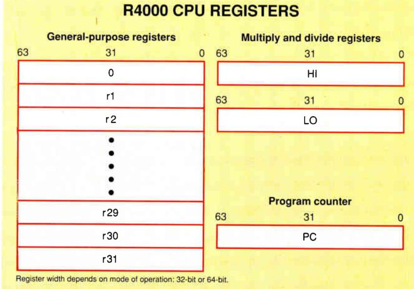
**Figure 1:** Only two of the R4000's registers have special functions: Register 0, following RISC convention, is a bit bucket, and register 31 gets the return address during subroutine calls. The multiply and divide registers store the 64- or 128-bit results of integer multiplication operations or the quotient and remainder of integer division operations.
