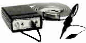
The HANDSCOPE is a unique measuring instrument to be connected to the printer port of the computer, without external power supply.
