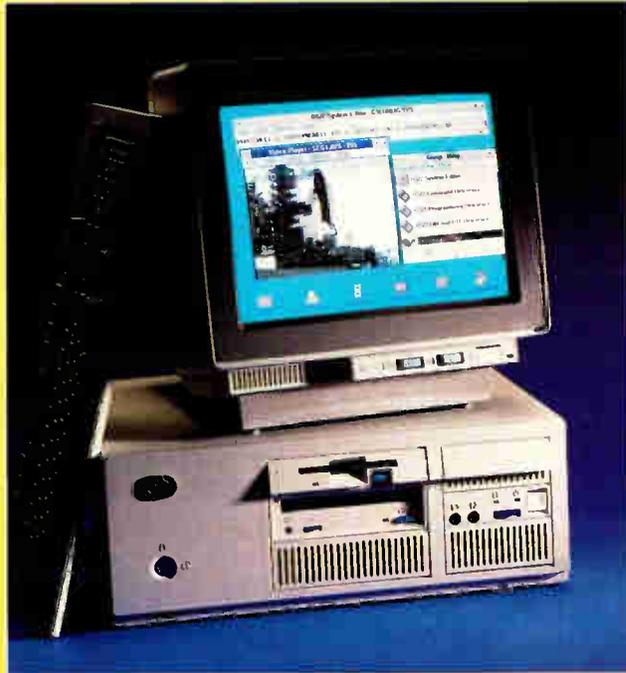
*IBM's first PC designed specifically for multimedia has a CD-ROM drive, an XGA graphics adapter, and an audio capture/playback adapter with a MIDI port.*
