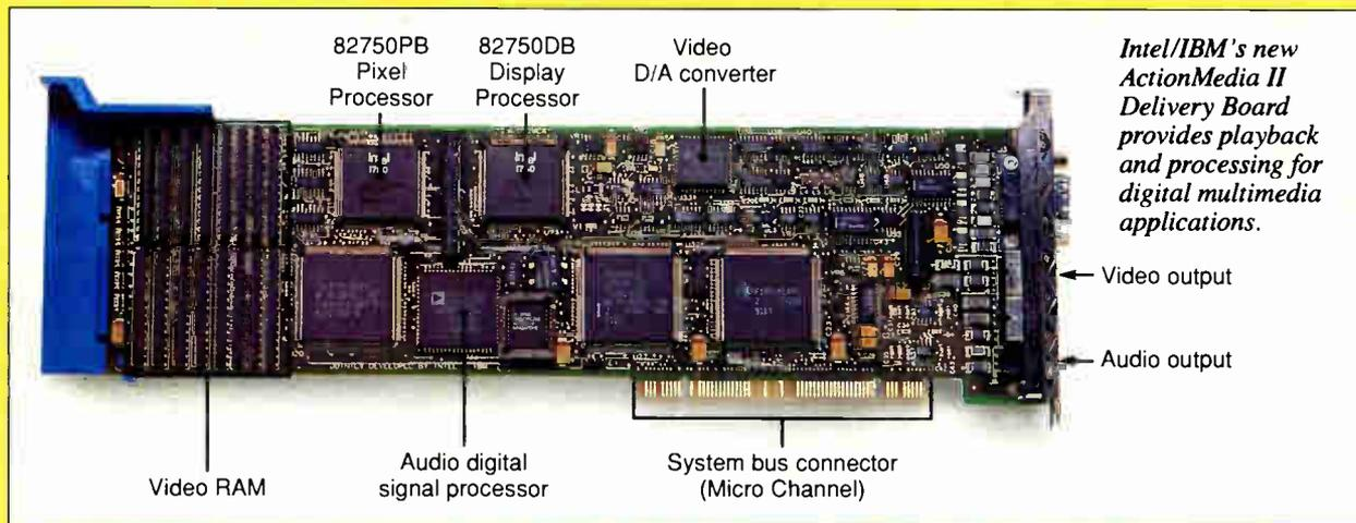
*Intel/IBM's new ActionMedia II Delivery Board provides playback and processing for digital multimedia applications.*
