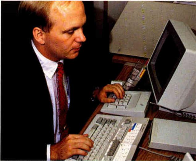
*Screen Reader/PM comes bundled with a small keyboard, about the size of a numeric keypad. This keyboard plugs into the mouse port on any PS/2 computer and lets you control all aspects of the SRD.*
