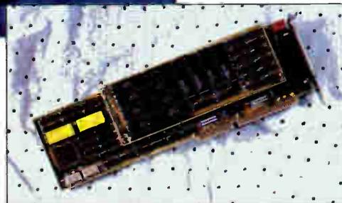
**Datatrans Speedboard™** is a proprietary serial I/O controller, developed by Datatrans to handle heavy data transfer in a multiuser computing environment. With its on-board 16 MHz 80186 processor, up to 512 KB of memory buffer, and statistical supporting software, Speedboard relieves main CPU overhead and effectively accelerates I/O speed.
