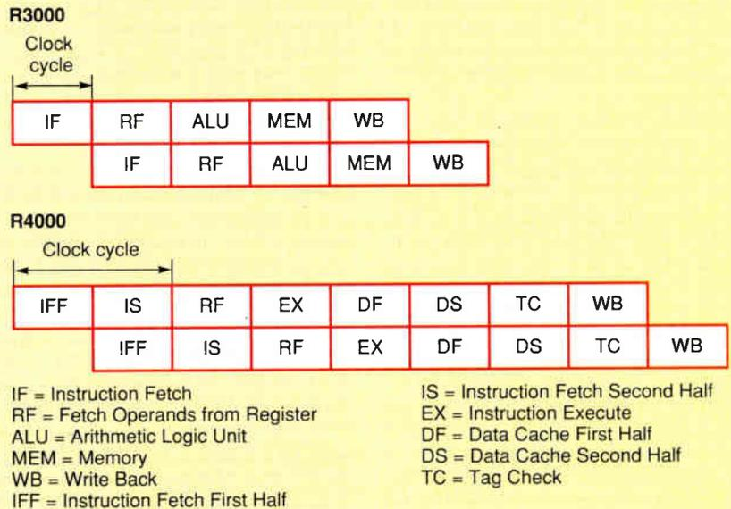
**Figure 3:** The R4000's eight-stage pipeline advances twice per clock cycle; the R3000's five-stage pipeline advances once per cycle. A superpipelined processor requires less silicon and less logic design effort than a superscalar processor. But since superpipelining depends on fast logic, circuit design is tougher. And since the pipeline can be split into only so many stages, the approach eventually runs out of steam—at which point the designers must contemplate a superscalar design.
