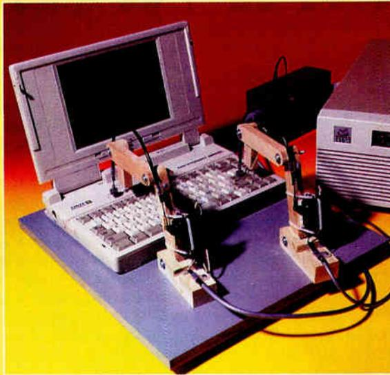
*The battery-life test station uses positional servo motors to actuate a remote rubber finger. To press a key, the motor extends a cable that pushes the finger into the key. Two arms handle most laptops—one for the Return key and one for the standby/power switch. Some laptops may require a third arm to press a Shift or function key.*
