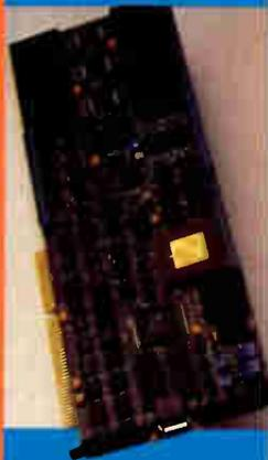
Truevision 1024-32 Graphics Engine provides acceleration for graphics and imaging applications operating under Windows. This single-slot solution features 32 bits per pixel and resolutions up to 1024 x 768.
