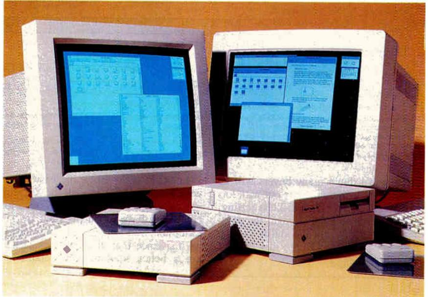
*Sun's entry-level ELC (left) integrates the CPU inside the monitor housing; the performance of the IPX (right) rivals that of Intel-based PCs.*
