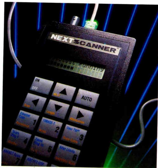
*After testing network wiring, Next Scanner compares the results to a table and indicates if the cable will support the application.*
