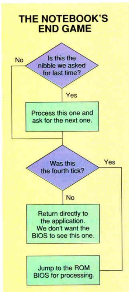
**Figure 3:** After retrieving a nibble of data from the printer status port, see if it's the nibble you asked for (by looking at the returned least-significant bit from the desktop). After processing the data, increment a tick counter. If the counter reached 4, reset it to 0 and branch back to the ROM BIOS. If not, exit back to the foreground application so the clock software sees only 18 ticks per second.
