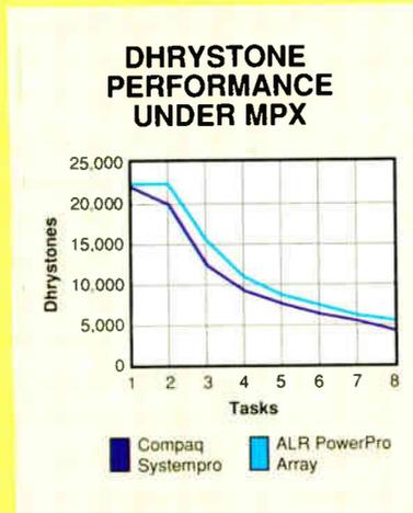
**Figure A:** Dhrystone performance for one through eight tasks. The PowerPro Array shows no performance degradation between one and two tasks running on its dual processors; the Systempro reveals some additional overhead.
