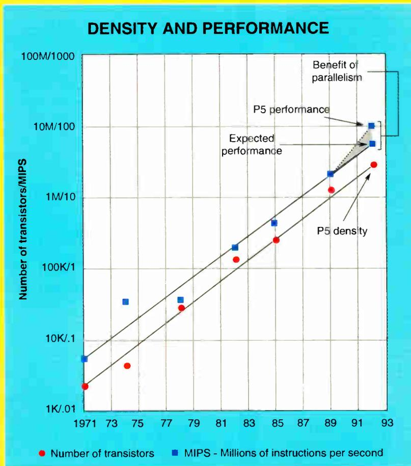
Figure A: When plotted side by side, the number of transistors in Intel 80x86 family of processors and their native MIPS ratings at introduction follow nearly parallel curves. The P5 is expected to sunder the relationship between density and performance by incorporating increased on-chip parallelism.
