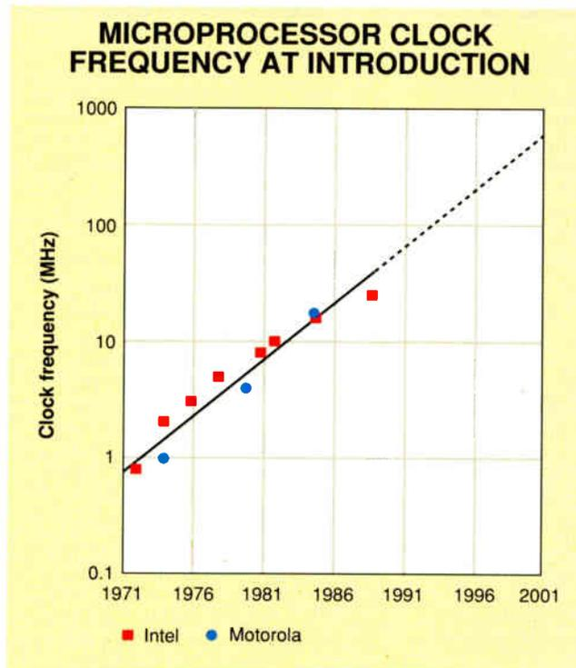
**Figure 2:** *The trend in microprocessor clock frequency is representative of the advances in ICs that will characterize the 1990s.*
