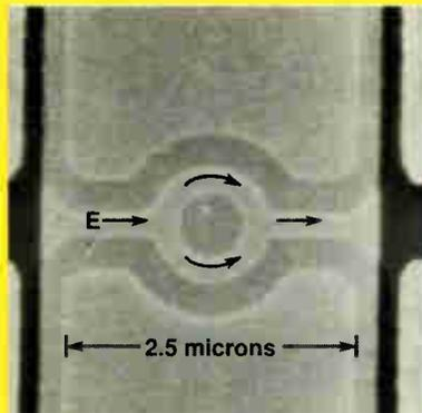
**Photo A:** *The Quantum interference device built by IBM researchers studying gallium arsenide. A magnetic field controls the interference between electron waves passing through the two halves of the ring, turning the device on and off.*
