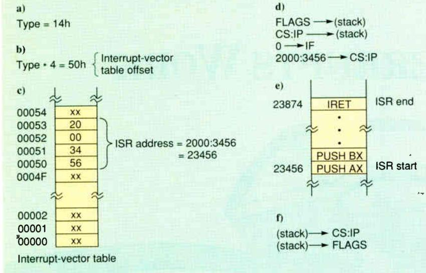
(a) Type byte received: type 14h; (b) multiply type byte by 4 to get interrupt-vector table offset (50h); (c) get ISR address (2000:3456) from interrupt-vector table (location 00050h); (d) push FLAGS register, Code Segment, and Instruction Pointer onto the stack, clear the interrupt-enable flag (IF), and branch to the ISR; (e) execute the ISR (at location 23456h), terminating with an IRET instruction; and (f) restore Instruction Pointer, Code Segment, and FLAGS register from stack.
