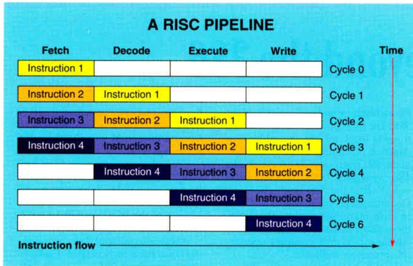
**Figure 2:** In this simplified RISC implementation, four four-cycle instructions are issued in sequence (one every clock cycle) to a four-stage pipeline. The first instruction begins executing at cycle 0, and the fourth begins executing at cycle 3, filling the pipeline. Although each instruction requires four cycles to complete, the overlap in execution steps lets them all finish in seven cycles, as opposed to the 16 required without pipelining.
