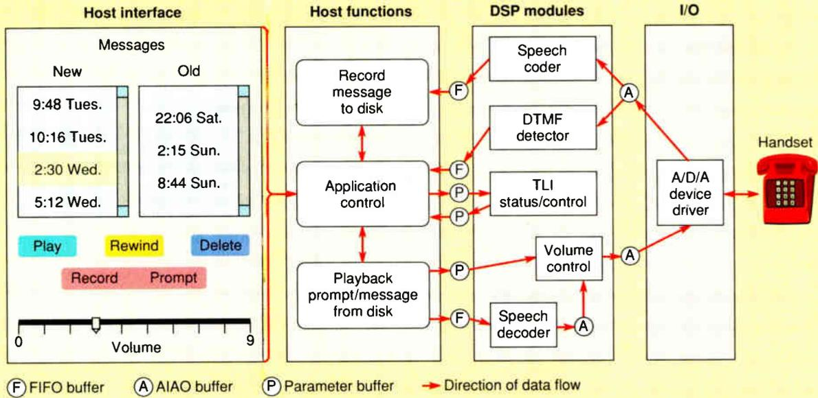
The host application, consisting of a user interface and assorted control functions, accesses the DSP chip by calling various modules from the VCOS Multimedia Module Library. The modules communicate with host functions, with each other, and with the I/O systems through intermediate buffers.
