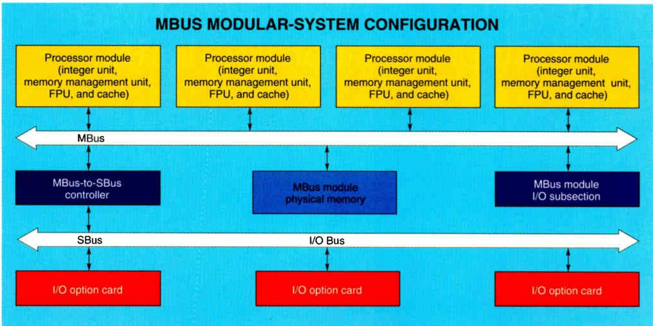
**Figure 4:** *MBus is a SPARC module interconnect bus that supports symmetrical multiprocessing for as many as eight processors and provides data transfers as high as 320 MBps. Systems using MBus as a processor bus also use a separate I/O bus, such as the SBus shown here. The MBus protocol includes the cache-coherency logic necessary for SMP operations.*
