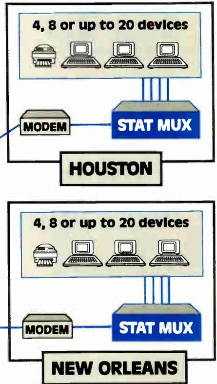
The Telplex® line of asynchronous statistical multiplexers by BayTech are designed to provide user flexibility and to maximize speed by effective utilization of high speed modem technology. Telplex stat muxes support hardwire connectivity for distances to 4000 feet.
