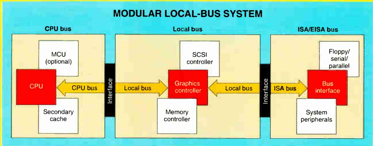
**Figure A:** This three-layered system uses a modular local bus running at 33 MHz to interconnect speed-critical functions. The system now supports 486 CPUs at speeds of up to 100 MHz and provides connections for slower peripherals on a standard 8-MHz ISA bus. The key element of the system's architecture is the separation of the CPU bus from the local bus; other architectures may connect the CPU directly to a local bus.
