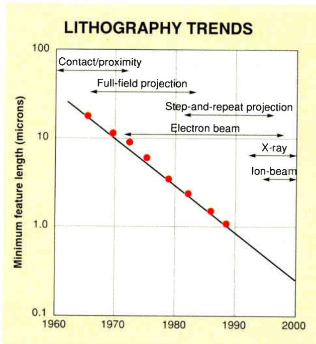
**Figure 1:** *The pursuit of the ever-finer line that has characterized semiconductor technology for the last three decades will come to an end as chips approach atomic dimensions. Depending on the material, the number of atomic spacings at 0.1 micron is in the low hundreds.*
