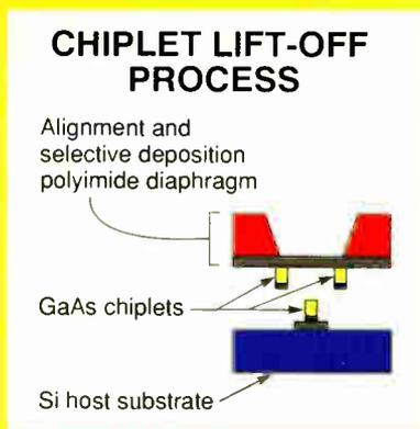
**Figure A:** The GaAs devices on the polyimide diaphragm are aligned with respect to the silicon host substrate, and they are deposited from the diaphragm onto the silicon. Individual devices or an entire array of devices can be aligned and deposited onto this host substrate.
