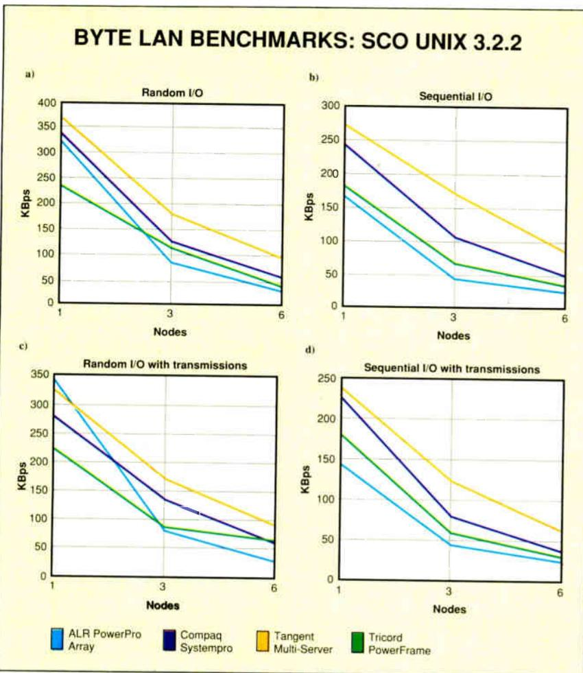
**Figure 2:** Performance under SCO Unix put the Multi-Server consistently out front. Parts (a) and (b) represent file I/O performance without network transmission. In (c) and (d), we measure random and sequential I/O throughput, including network interaction. In each test, the Systempro also performed well, but the PowerFrame's lack of software support for striping placed it a surprisingly low third.
