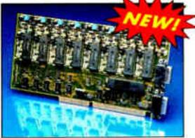
24 Digital I/O lines are built into the **DAC 812** which may be used for TTL-level applications.
