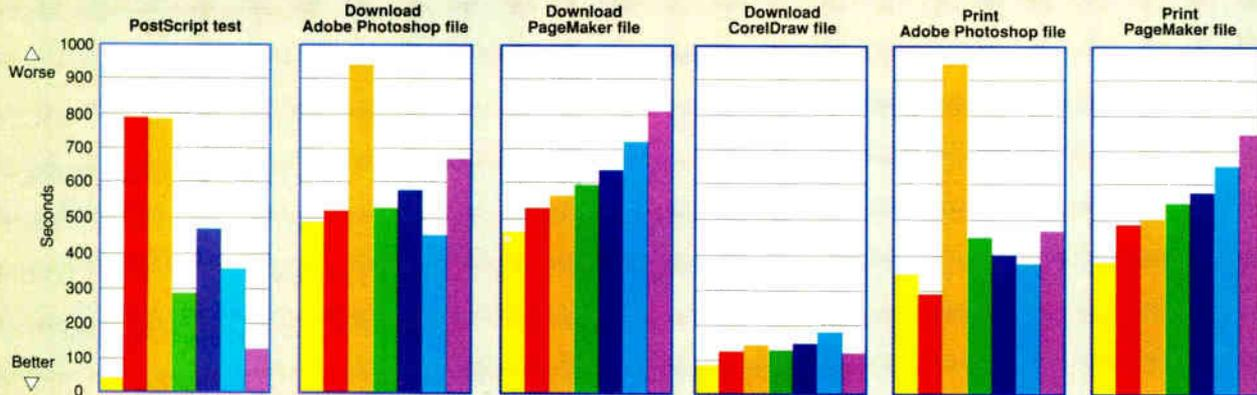
Timing results of the printers at various tasks. With the exception of the Photoshop file downloading and printing, the Tektronix Phaser II PXi was the fastest printer.
