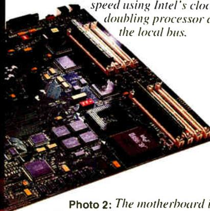
**Photo 2:** The motherboard in the Vectra 486u has a second socket to implement Intel's overdrive scheme.
