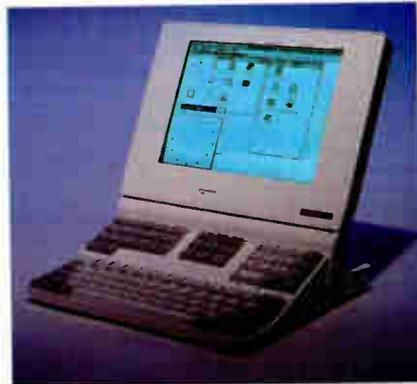
Combines Space-Saver Keyboard, LCD Monitor and 20 Mhz 386sx CPU w/2 Meg RAM (4 Meg optional) in a single very small footprint (27.4 X 26.0cm). Network ready with 10 Base2, 10 BaseT NE-2000 compatible network adapter built-in. Unit does not fold for portability.
