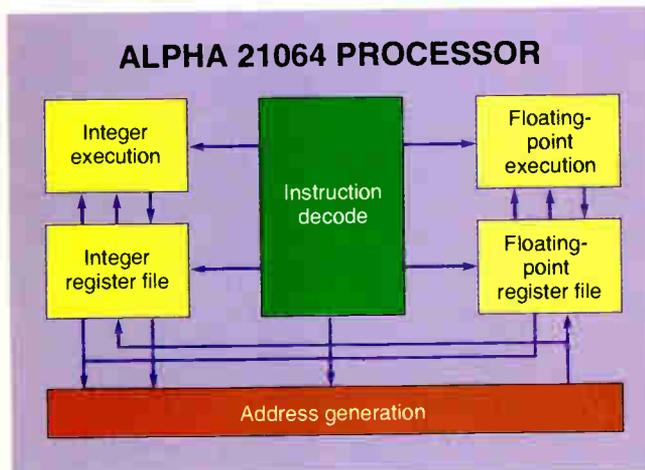
**Figure 2:** Avoiding bottlenecks is the goal of the Alpha core architecture, shown here with distributed floating-point and integer register files and execution logic.
