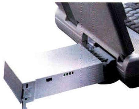
CAD battery sub-system provide up to three hours of portability. A unique design feature allows the EasyStor PDM to "sleep" whenever your notebook transfers to the sleep mode.
