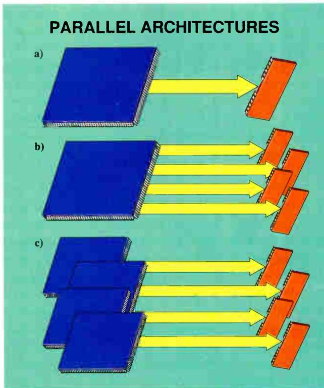
**Figure 1:** (a) In a serial computer system, one instruction works on one data item at a time. (b) In SIMD machines, many data items are manipulated simultaneously by one instruction or by identical instructions on different processors. (c) In MIMD machines, multiple processors act independently on different data items.
