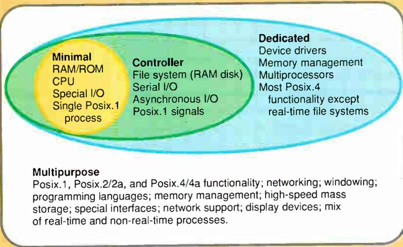
Figure 2: The application environment profile core of Posix.13 is the minimal profile. Successively larger and more robust application environment profiles build on this core.
