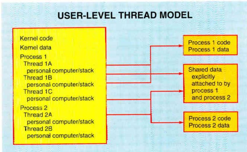
**Figure 2:** A system providing user-level threads is a protected-memory system in that it protects each process and the kernel, but it allows a process to contain multiple threads of execution. The threads executing within a process have immediate shared access to all global data within the process.
