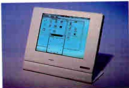
This 10" black on white monitor is easy-to-read, yet compact. Resolution is 640x480 with sharp, flicker-free image. Sharp's high refresh rate, triple supertwist nematic technology with back lighting provides a super bright, low radiation screen with a wide viewing angle. The adjustable monitor base is only 29x14 cm. It lets you mount the LCD monitor on vertical surfaces or fold for transport. Comes with 1.5 m cable and VGA adaptor card. No external power required. IBM AT compatible.
