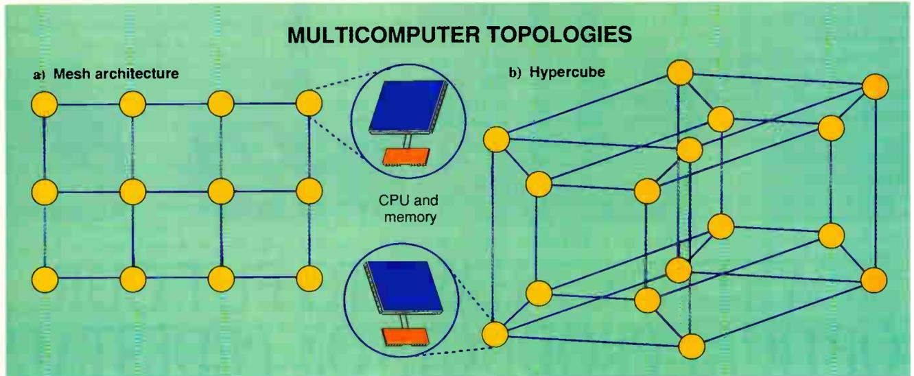
**Figure 3:** The topology you use in a system depends on the nature of the application. (a) If most interprocessor communication is local—within one or two nodes—a mesh architecture is most cost efficient. (b) When communication is more widespread, a hypercube may be necessary to minimize latency.
