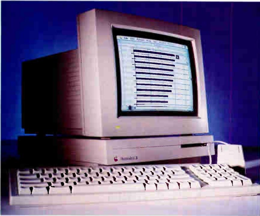
The Mac LC II packs a 68030 CPU, 4 MB of RAM, and 32-Bit QuickDraw capability into a compact box.
