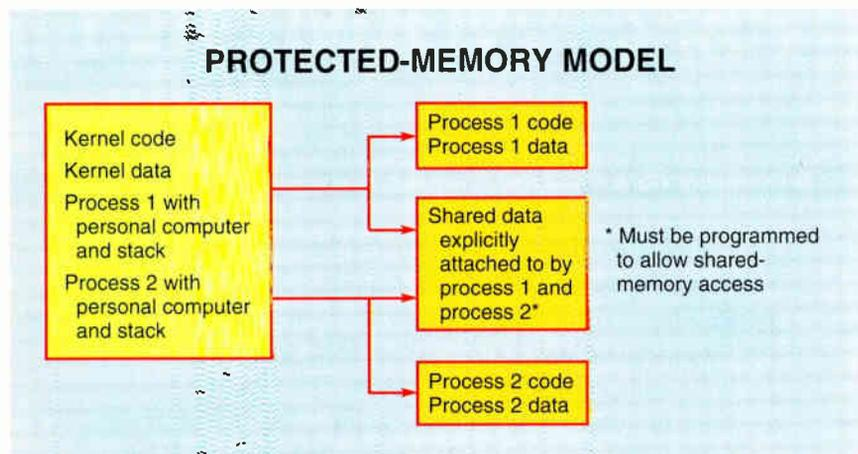
**Figure 1:** The protected-memory model reserves protected data and code areas for each process. Provisions for sharing data between processes must be specially programmed.
