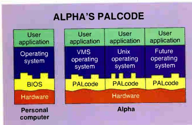
**Figure 1:** Operating-system independence is the goal of Alpha's PALcode. PALcode consists of subroutines that handle context switching, memory management, and other primitives specific to each operating system. PALcode is similar conceptually to the BIOS of a personal computer.
