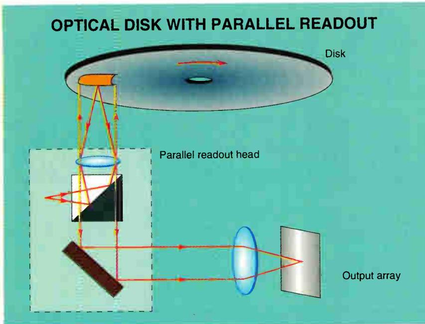
**Figure 1:** A conventional optical memory disk is illuminated with an unfocused beam to address thousands of stored bits in parallel. The illuminated portion of the memory is imaged onto a detector array, and the detected signal becomes part of the computer's RAM space.
