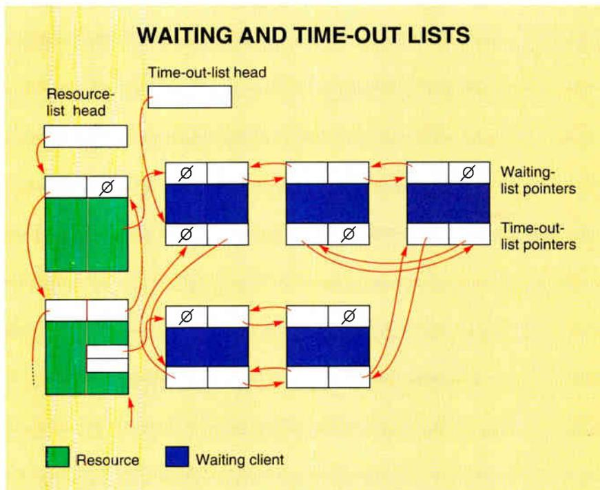
*Attached to each resource is a list of lock definition blocks representing pending lock requests. Lock requests enter the lists in order of arrival; pending requests are also connected to a systemwide time-out list. Requests are attached to the time-out list based on the length of time each associated client will wait for lock request service.*
