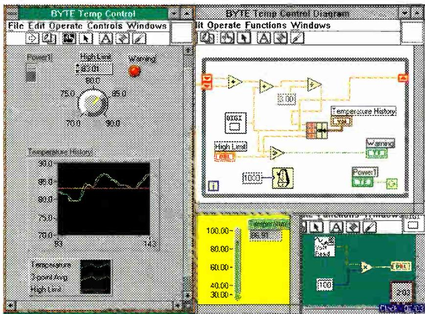
LabView uses a CAD-like technique that lets you draw your data acquisition application. In this example, the instrument panel on the left is driven by the diagram on the right. The Digi icon encapsulates the display and diagram at the bottom right.
