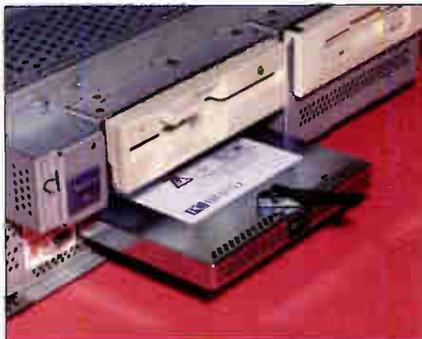
*The PC Brand CPU module makes upgrading microprocessors a snap. Inside the cartridge are the microprocessor, coprocessor, cache, and a few support chips. The 9- by 11-inch system board holds the BIOS and main memory, the IDE controller, floppy disk controller, SVGA display adapter, and one parallel and two serial ports.*
