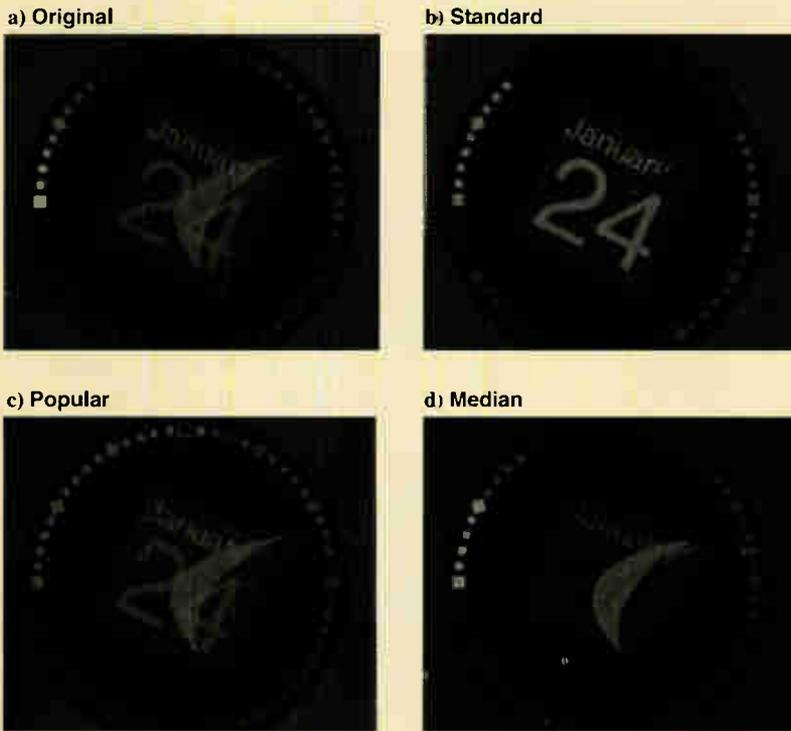
Figure 6: An example of the image results you can expect when using several color-selection mechanisms. (a) is the original image, (b) uses the colors in the standard 4-bit system palette, (c) uses the 16 most popular colors, and (d) uses 16 colors as calculated by the median-cut algorithm.
