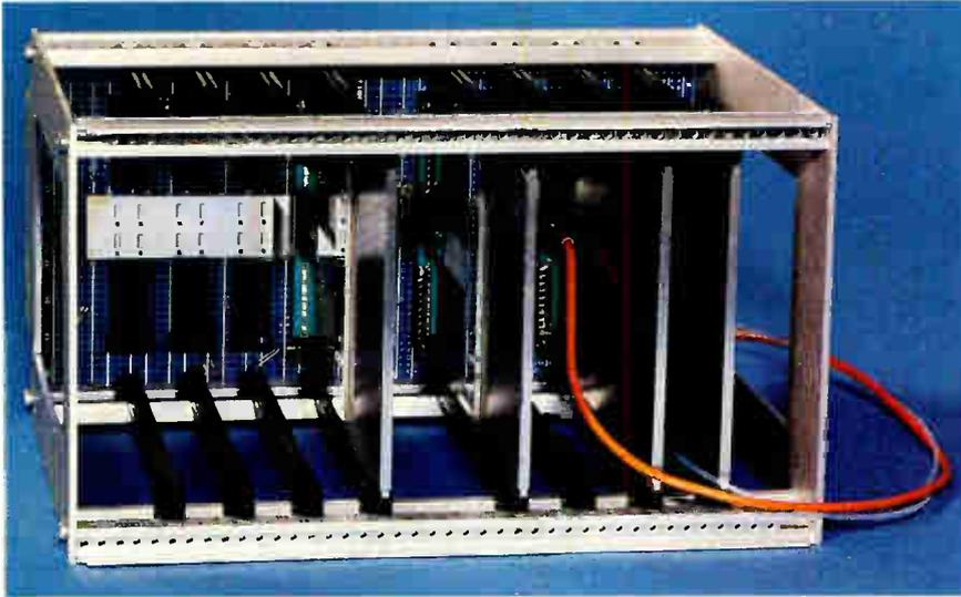
**Photo 3:** Optical backplane hardware assembled in a VME card cage. Its function is to implement 32 fanouts distributed over four double-sided daughterboards inserted in the four card slots on the left side of the card cage. The prototype device was produced by Charles T. Sullivan, Bruce L. Booth, and Anis Husain. (Photo courtesy of Honeywell Systems and Research Center, Bloomington, MN)
