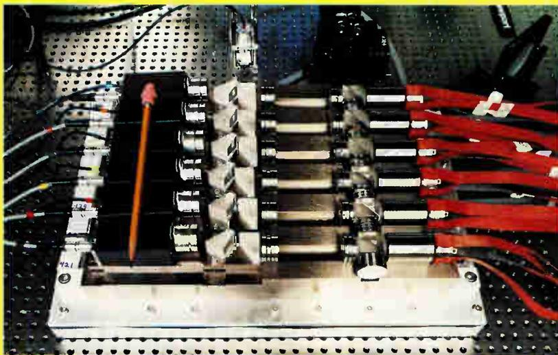
**Photo A:** A 16-by-32-bit-wide multistate-interconnection-network prototype developed by AT&T Bell Laboratories (Naperville, IL). This switching fabric is based on free-space digital optical interconnections and S-SEED devices. (Photo courtesy of AT&T Bell Laboratories)
