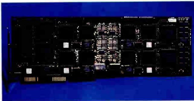
Dialogic's \$1150 Dialog/41D, which includes a DOS development kit. This board supports up to four channels for dial-up or—for heavy-demand services using an additional adapter like Dialogic's \$2300 DTI/124—a digital T1 line. (Heavy fax broadcasting applications without voice synthesis require a direct connection from the MLCP-4 to the T1 board.) Dialogic
