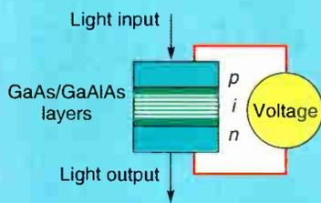
An S-SEED is a p-i-n photodiode built around multiple layers of GaAs and GaAlAs (gallium aluminum arsenide). These layers act as quantum wells, trapping electrons and holes close by. The resulting energies determine the optical transmission of the device.
