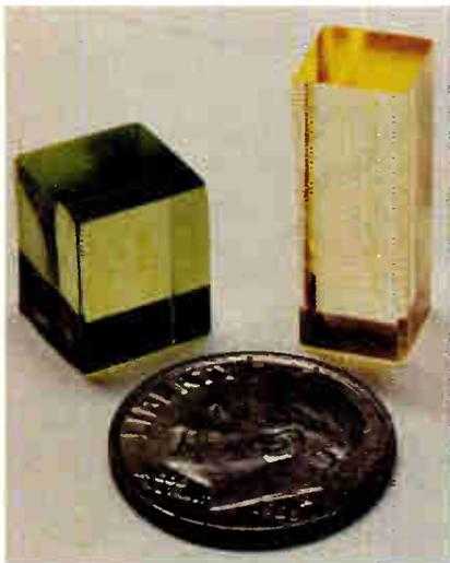
**Photo 1:** Polymer memory cubes such as these prototypes developed by UCI's Peter Rentzepis are capable of storing information in three dimensions. Data can be written and read in thousandths of a second by two laser beams. (Photo courtesy of University of California—Irvine)
