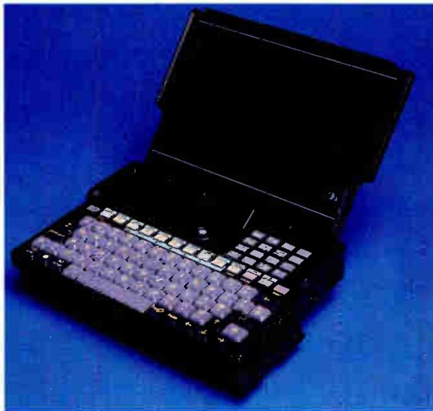
around the 16-MHz NEC V30HL 8086-compatible processor. It has 1 MB of RAM, of which 384 KB is configured as expanded memory. The DSP is provided by Analog Devices, and future Olivetti machines may well provide additional functionality through the DSP. Currently, only a speech module is provided, which creates speech files compatible with a number of other vendors who use the Analog Devices DSP. The files are not compatible with Sound Blaster files, and no conversion utility is available yet.
