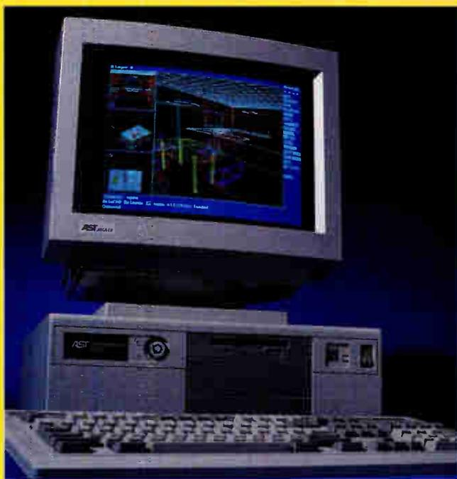
Adding 4 MB of memory to each of two SIMMs was simple. The 4/50d's cover, secured by three hand-tightened screws, popped off easily. Once I got inside, I could easily pull out the processor board, which can be populated with up to 16 MB of memory, from the motherboard to quickly snap in the SIMMs. The whole process took about 15 minutes.
