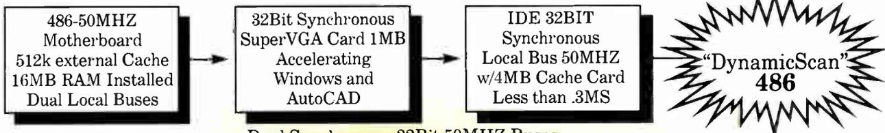
Dual Synchronous 32Bit 50MHZ Buses
