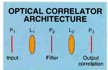
**Figure 2:** You can use this optical system to compute a wide variety of features. The input image is placed at  $P_1$ , a filter is placed at  $P_2$ , and the correlation of the input and filter function appears at  $P_3$ . By using various  $P_2$  filters, you will find that this architecture can achieve all major low-, medium-, and high-level computer-vision operations and all functions needed in figure 1.
