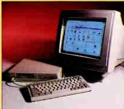
*The Addtech SlimPro, a transportable computer similar to the Ergo Brick and the Flytech Carry1, lets you carry your computer from site to site and be able to plug in a full-size keyboard and monitor.*
