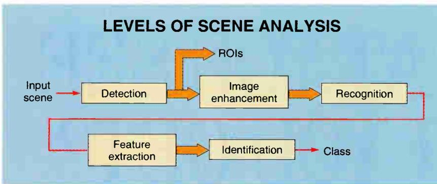
**Figure 1:** The first two operations let you locate and enhance a candidate ROI (region of interest) in a scene. Then, typically, you calculate features that describe the contents of each ROI and input them to a classifier that determines the identity of the object in each ROI.
