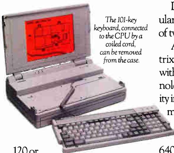
*The 101-key keyboard, connected to the CPU by a coiled cord, can be removed from the case.*
