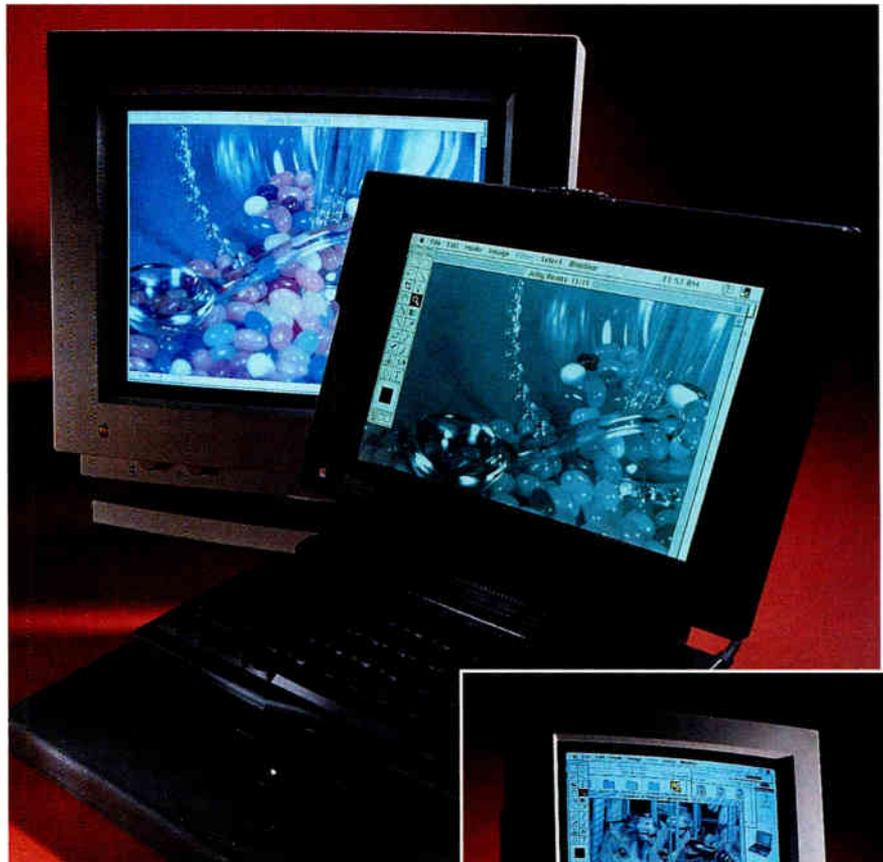
**Photo 1:** *The PowerBook 180, shown here with an external color monitor, bundles more performance than a Mac IIfx into a 9.3- by 11.25- by 2.25-inch package.*
