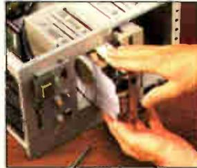
You install the 1.2 meg, 5-1/4" floppy disk drive, learning disk drive operation and adjustment. Later, you dramatically improve your computer's data storage capacity by installing a powerful 80 meg IDE hard drive.
