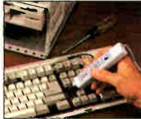
After you build this digital logic probe, you explore the operation of your computer's 101-key, detached "intelligent" keyboard and its dedicated microprocessor.
