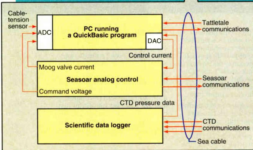
**A personal computer on-board the research ship** takes the ASCII data coming into the serial port and plots it as five separate curves representing the five elements of data. In addition, the program sends pressure data out through an A/D converter to the shipside Seasoar controller, thereby eliminating the need for the Seasoar depth sensor.
