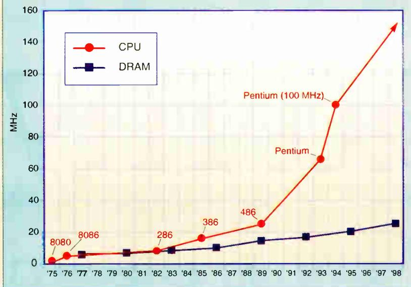
Comparing the relative speeds of microprocessors and memory chips necessarily requires some apples-and-oranges compromises, but no matter how these curves are plotted, the results are similar: CPU performance is rapidly outstripping DRAM performance. While the CPU curve climbs steeply, the DRAM curve remains almost flat.
