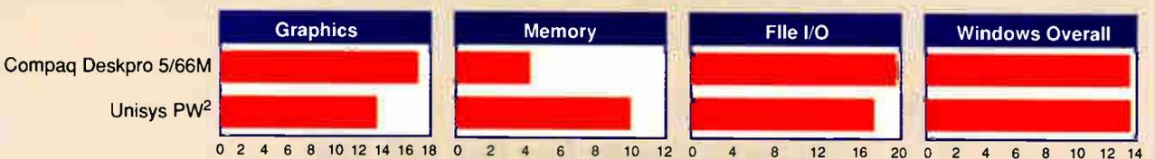
All results are indexed, and higher numbers indicate better performance. For each index in the Windows tests, a Compaq Deskpro 386/33L running Compaq DOS 5.0 and Windows 3.1 = 1. The overall index is the average index of the individual tests.
