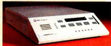
Its menus make configuration easy, but you will probably do fine with the defaults. The Comsphere is designed to be easy to upgrade; we upgraded it from a V.32bis modem to a V.32terbo modem by downloading software over the phone. Its impaired-line performance was a perfect 100 percent, and its best-case throughput was near the top.
