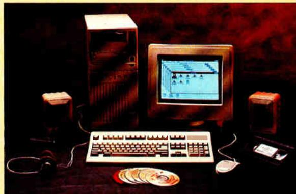
The Mega M46D2LM (\$3895) local-bus multimedia system has 8 MB of RAM, 256 KB of cache RAM, 2 MB of VRAM, and 1 MB of DRAM. The MPC-compliant system includes a Pro Audio Spectrum 16 sound card, speakers, a microphone, and headphones. The medium-tower system can read multisession Photo CDs and includes Windows NT driver support.
