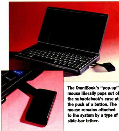
The OmniBook's "pop-up" mouse literally pops out of the subnotebook's case at the push of a button. The mouse remains attached to the system by a type of slide-bar tether.
