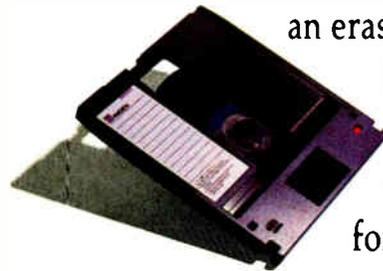
The multifunction capability allows use as an erasable, rewritable work-horse drive. And as a WORM (write once read many) archiver for mass storage.
