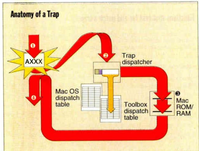
When an exception occurs ①, program flow jumps to the Trap Dispatcher ②, which uses the Toolbox bit in the trap word to select a dispatch table address. This address is used to locate and execute a routine in ROM or RAM ③. The thread of execution then returns to the next instruction in the Mac program ④.
