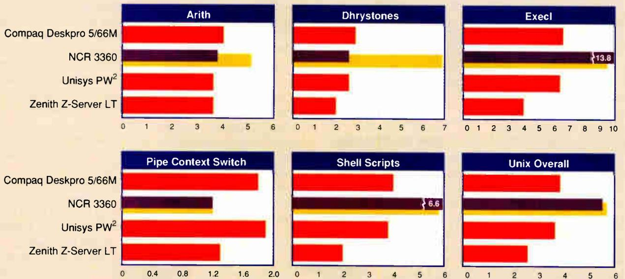
All results are indexed, and higher numbers indicate better performance. For each index in the Unix tests, a Sun Sparcstation IPC = 1. The overall index is the average index of the individual tests.
