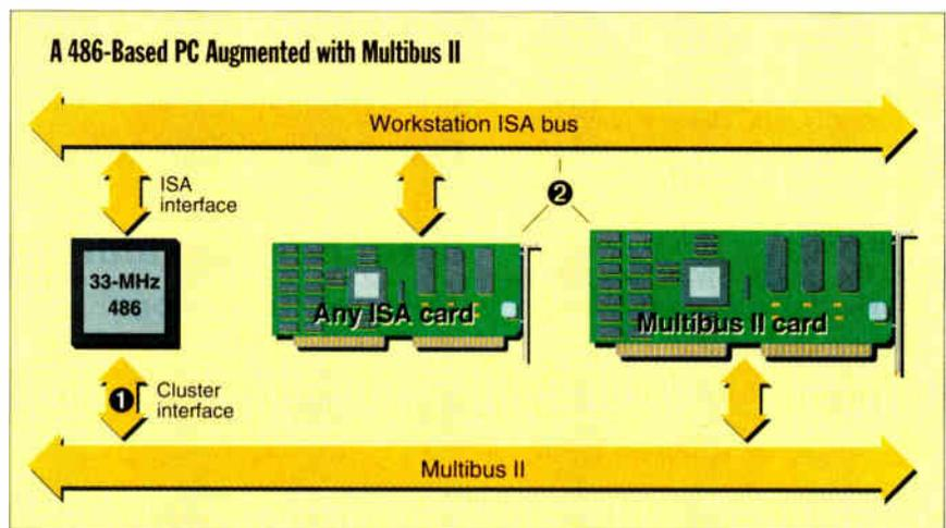
**PC-cluster interface software** ① decouples the CPU from transfer overhead and uses a backplane message-passing protocol, enabling concurrent I/O data transfers at maximum bandwidths. ② A workstation's ISA bus doesn't have sufficient bandwidth to push data fast enough for I/O-intensive operations. But under applications-software control, a 320-Mbps Multibus II bus can assume I/O-intensive operations. Routine system tasks are left to the ISA bus.
