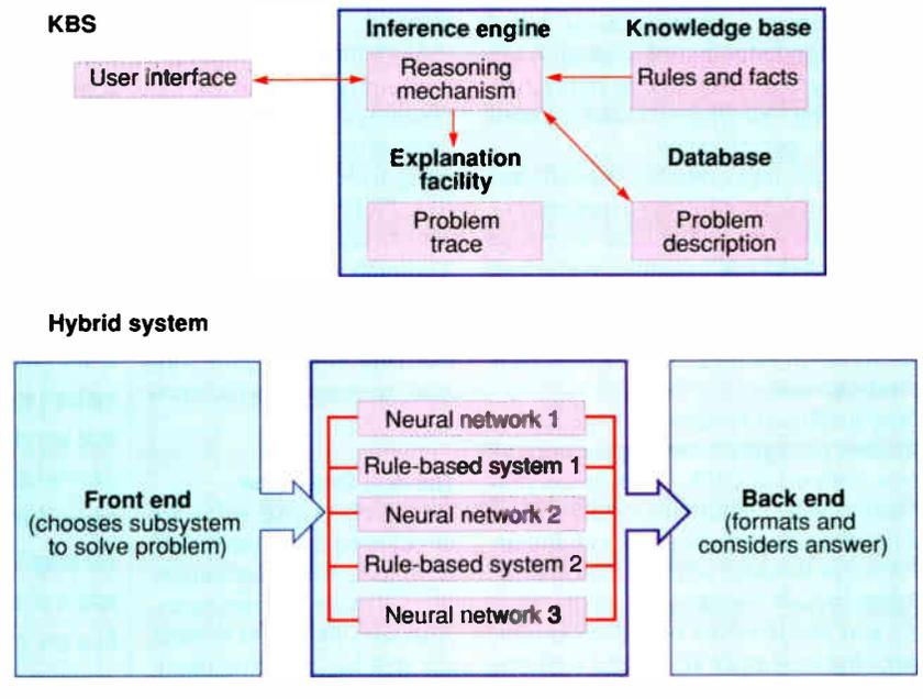
**A generic KBS (knowledge-based system)** relies on its own database, knowledge base, explanation facility, and inference engine, but a hybrid system can select a subsystem to handle each problem through the front end while the back end formats and consolidates partial answers from each subsystem. (Data courtesy of Silverman, Barry. *Expert Systems*, Addison-Wesley, 1987; Eberhart, Russell C., and Roy W. Dobbins. *Neural Network PC Tools: A Practical Guide*, Academy Press, 1990)
