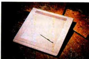
and manipulate them faster and more naturally than previously possible. The Wacom Technology (Vancouver, WA) device has a customizing menu strip with two pressure buttons that let you set the pressure-sensitive UltraPen for a firm or soft touch.
