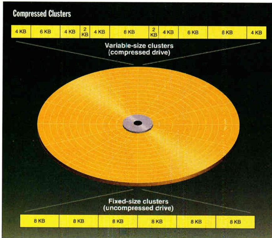
**Uncompressed DOS drives** normally store data in fixed-size clusters of 8 KB. (Macintosh clusters are also fixed size, but the size varies depending on the drive capacity.) Compressed drives store data in clusters that vary in size according to the compression ratio. A cluster may be as small as 512 bytes (assuming a 16-to-1 compression ratio) or as large as 8 KB (if the data is uncompressed). The average is about 4 KB (2-to-1 compression).
