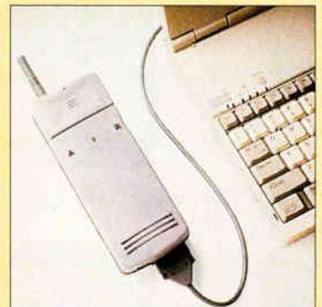
The AirCommunicator connects to the serial port of your portable PC and transmits over standard cellular phone networks; an RJ-11 jack lets you connect to standard phone lines. You can send data at a transfer rate of up to 57.6 Kbps and send and receive faxes at up to 14.4 Kbps. The device automatically switches between different standard protocols for maximum efficiency. Cost is \$1495.
