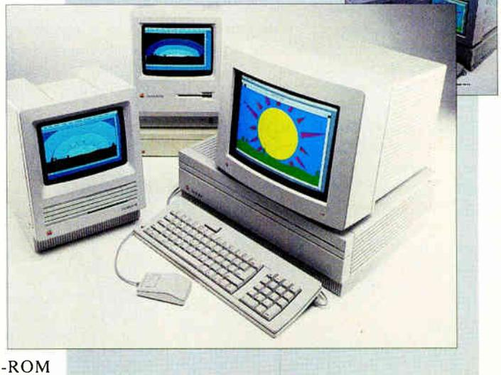
**1988:** Apple migrated the Mac to the 68030 processor, by introducing first the Mac IIx (\$7769) and then, in January 1989, the Mac SE/30 (\$4369). These computers featured the SuperDrive, a high-density (1.44-MB) floppy drive that could read and write DOS or OS/2 floppy disks, and a 68882 FPU. Owners of Mac IIs and SEs could upgrade to the new machines with a floppy drive and main logic board swap.
