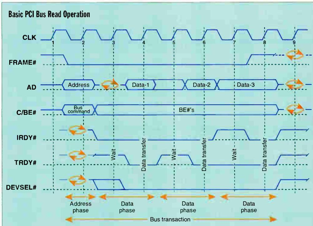
**A read transaction starts with the address phase**, with FRAME# asserted, AD[31::0] driving the address onto the bus, and C/BE# containing a valid PCI bus command. The data phase follows, which can have any number of data transfer and wait cycles. During the data phase, C/BE# indicates what byte lanes are used.
