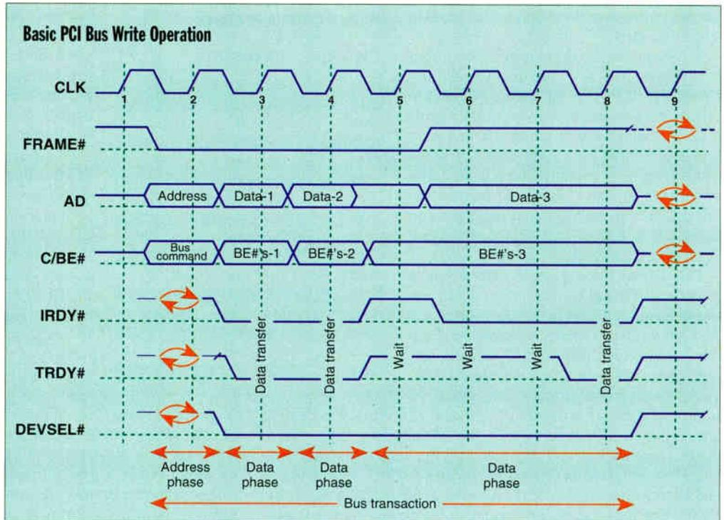
**A PCI write transaction is similar** to a read transaction. The data phase of read and write transactions ends when both IRDY# and TRDY# are asserted. The wait states shown here are inserted only when a slow device is accessed.
