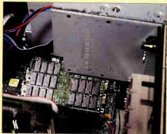
**The Acma 486 Tower includes** both a 3½-inch and 5¼-inch floppy drive. Unfortunately, the manufacturer doesn't follow the convention of designating the 3½-inch drive as the A drive. We couldn't reverse drive designations from within the BIOS setup since both drives are on the same ribbon cable connector, and the documentation did not provide any information on changing jumpers.
