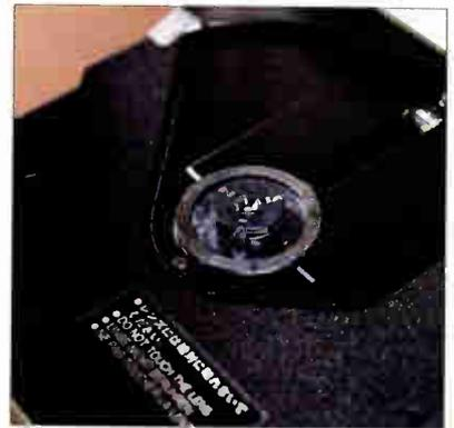
as do the Pentiums and 486s we received from DEC. This unique drive design uses three spring-backed ball bearings to hold a CD in place.
