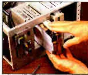
You install the 1.44 meg, 3-1/2" floppy disk drive, learning disk drive operation and adjustment. Later, you dramatically improve your computer's data storage capacity by installing a powerful 200 meg IDE hard drive.
