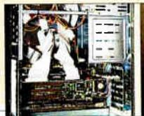
This EISA/VL-Bus tower provides the fastest performance in this category in the BYTE Unix tests, along with plenty of room to grow. It can hold up to eight drives, and it offers 16 SIMM sockets for up to 256 MB of RAM. The internal cabling is well placed, so you can access all internal components without a fight. Cornell's ISA-based cousin was the second-fastest most expandable system in BYTE's Unix tests.
