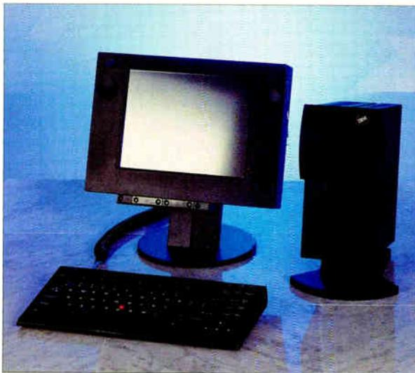
The 603-based desktop can drive flat-panel displays, as well as standard CRTs.
