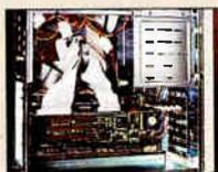
In addition to its superior performance, this huge tower also supplies growing room: It offers two 3½-inch drive bays and four 5¼-inch drive bays, along with three available EISA slots and one VL-Bus slot. CompuAdd's C466De Mini Tower posted the second-highest speed scores. Its sturdy tower chassis supports four 3½-inch and three 5¼-inch drives. Five 32-bit EISA and one VL-Bus expansion slot were available for additional cards.
