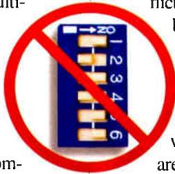
opening the computer and physically setting the jumpers and DIP switches. And since no standard has been set to determine which cards can use which resources, numerous conflicts can arise between cards. Often, it's a process of trial and error to determine which resources aren't already being used by other cards.
