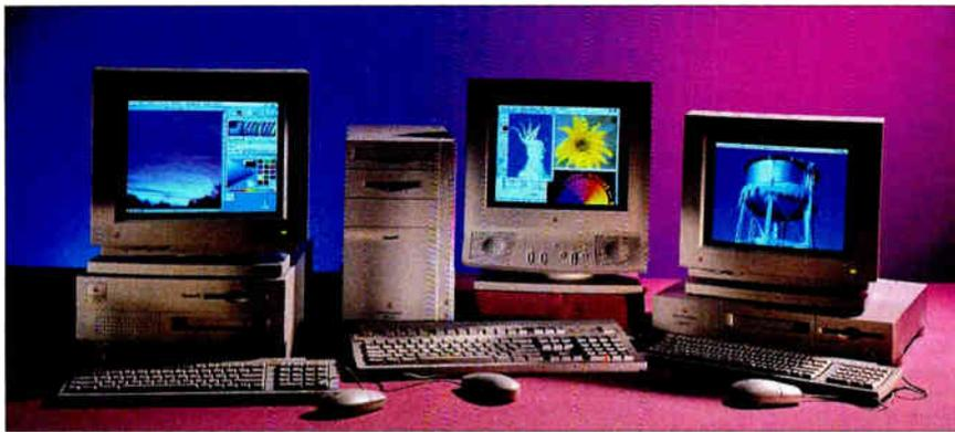
Left to right: the Power Mac 7100/66, the Power Mac 8100/80, and the Power Mac 6100/60. The systems are shown with an optional CD-ROM drive. A plug-in board provides AV capabilities.
