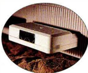
**A "paper out" flag** on the HP LaserJet 4MP tells you at a glance when the input tray is low on paper. The bright-orange flag, which is easily seen whether the printer is at your desk or connected remotely to a network, drops automatically. The printer need not be on for this feature to work.
