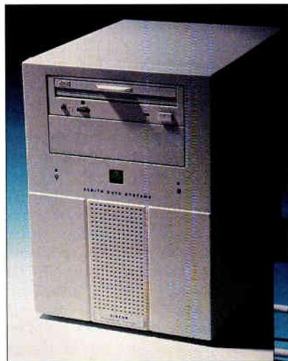
The 8- by 11- by 12-inch Z-Stor Personal Server provides dedicated file and printer sharing for peer-to-peer Ethernet LANs. The optional internal CD-ROM adds \$499 to the \$999 base-unit price of the Model 400. Hooking to coaxial cable requires an optional FriendlyNet connector (inset).
