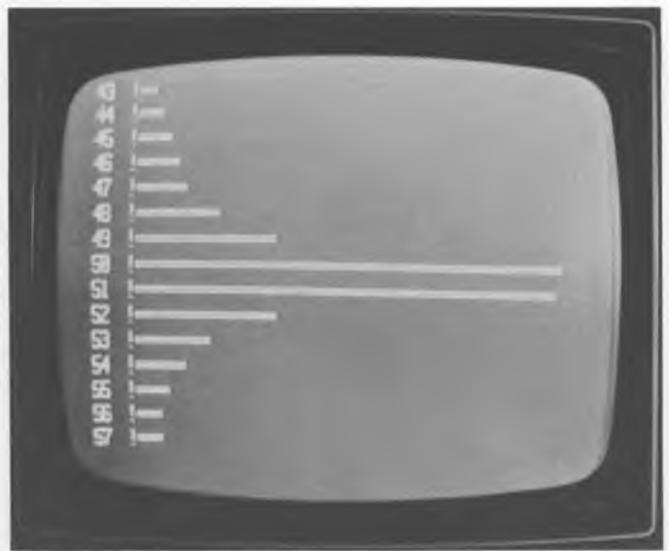
Photo 5: Video graphics display of the magnitude spectrum corresponding to a sine wave whose assumed frequency is 1010 Hz with a sampling interval  $T = 0.1953$  ms. This frequency corresponds to the midpoint between the 50th and 51st harmonics, and the imperfections of the DFT in representing a continuous time signal now can be seen.
