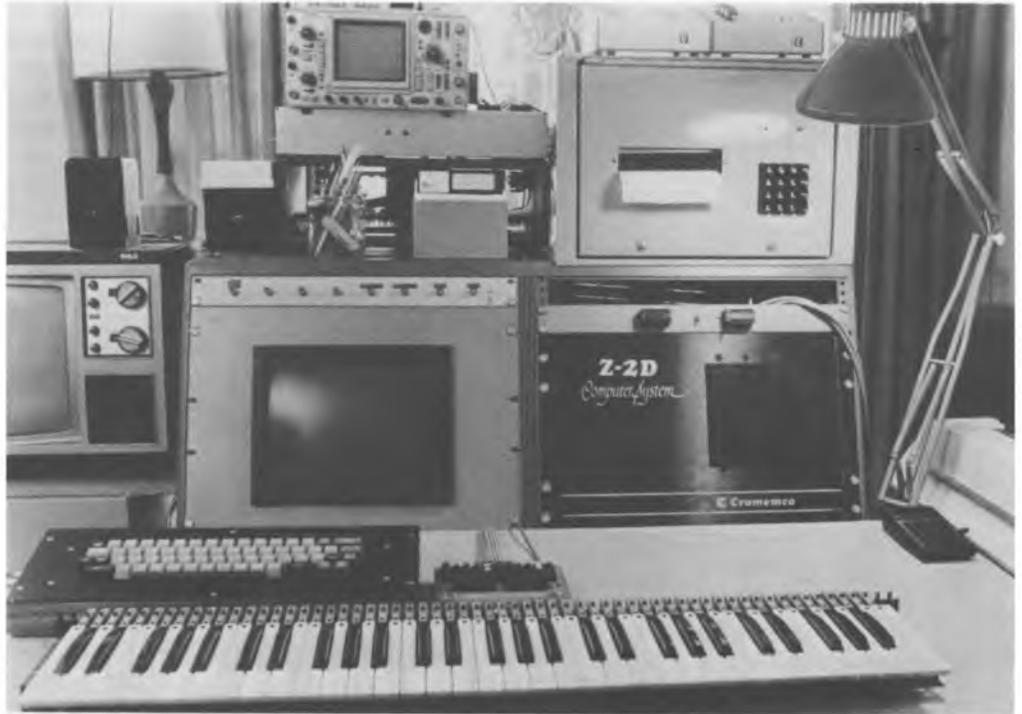
*Photo 1: The author's polyphonic music keyboard system, which allows more than one note to be played simultaneously. The scanning keyboard interface is just behind the 61 note manual in the foreground. The stand alone ASCII keyboard in front is dedicated to music related tasks, and allows two easily distinguished levels of system control.*
