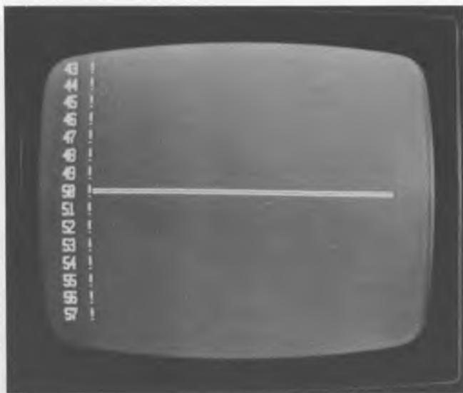
Photo 4: Video graphics display of the magnitude spectrum corresponding to a sine wave whose assumed frequency is 1000 Hz with a sampling interval  $T = 0.1953$  ms. This assumption results in an integer number of cycles (50) in the record duration  $t_p$ , which corresponds to 50 ms. The frequency then corresponds exactly to the 50th harmonic and the spectrum appears as a single line.
