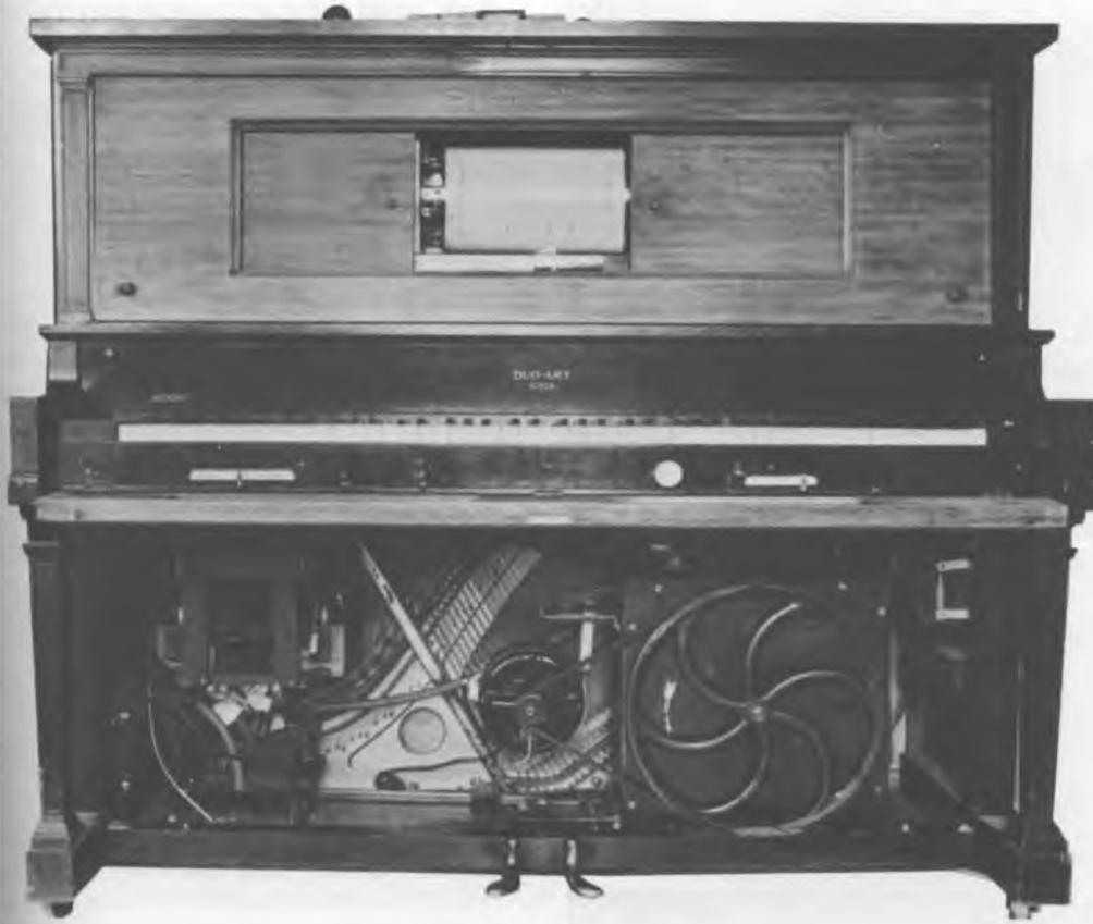
*Photo 1: The Duo-Art reproducing player piano as it is currently displayed in my home. Notice the electric motor at bottom center. It is original equipment. The vacuum pump is at the right; it is connected to the motor by a 1968 V8 Buick fan belt, which just happens to be a perfect fit. The piano was built in 1925 and required extensive renovations. The binary dynamics control system is located at bottom left (see photos 3a and 3b).*
