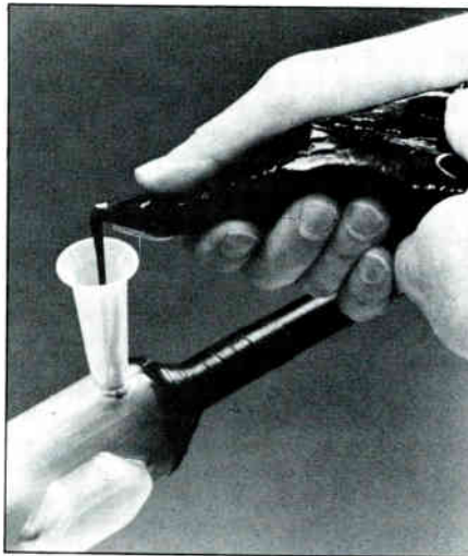
3M's CX-8990 closures come with a moisture-proof hard encapsulant.
