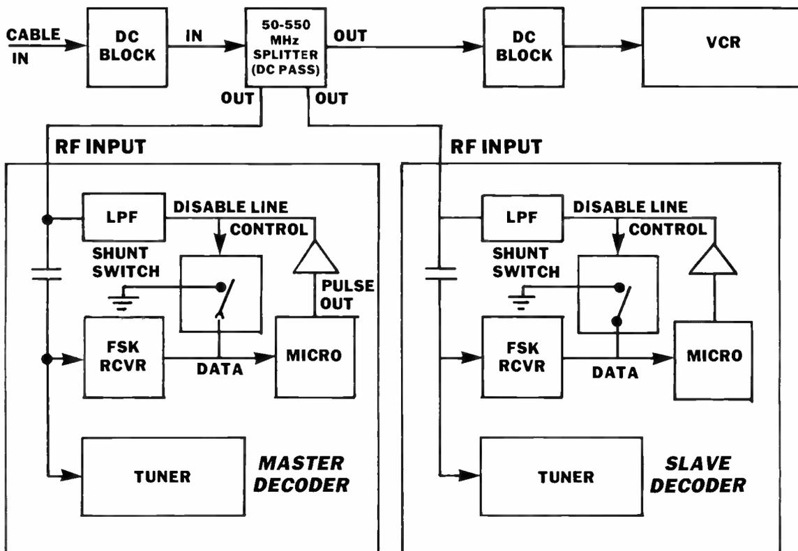
Figure 1 illustrates a functional block diagram of a master/slave configuration, the FSK inhibit approach. The master is designed to transmit a DC pulse of a certain duration to the slave that will disable the slave decoder's control data line during a deauthorize message that follows an inhibit message. (See Figure 2.) The DC pulse is put on the RF input cable of the master decoder whenever an inhibit command is received from the headend via the out-of-band standard FSK control channel.
