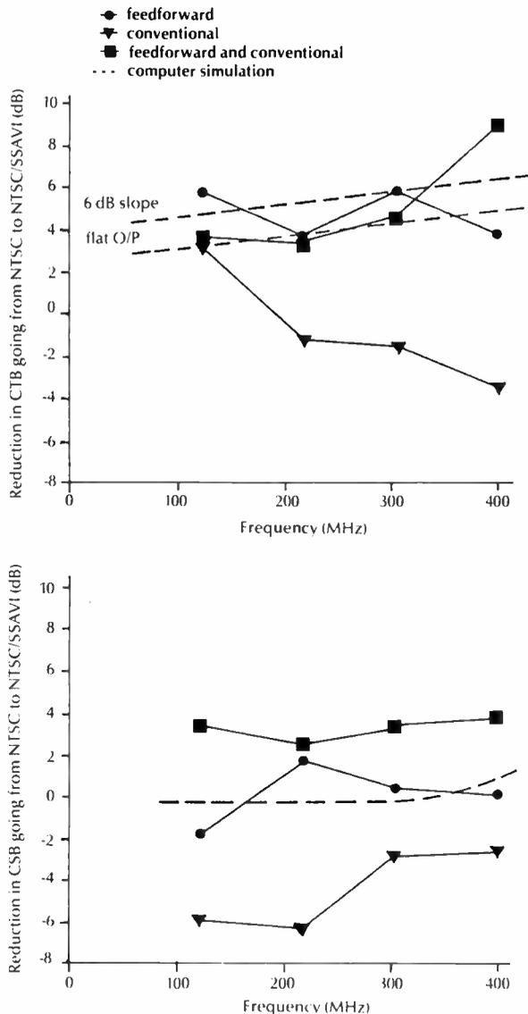
forward post-amplifier is shown in Figure 5, where it can be noted that for any signal format, significantly less feedforward improvement is obtained for CSB than for CTB.
