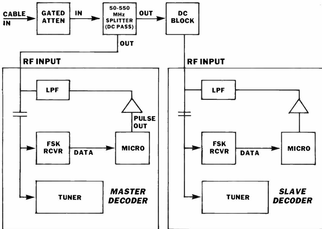
slaves or masters. The DC block units are required to block any DC signal from entering the system, as well as to prevent possible DC signal attenuation caused by customer equipment hook-up (such as VCRs). Most commonly available splitters can pass DC signals without significant degradation from output to output.
