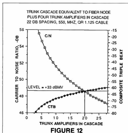
mitted the direct replacement of the amplifier locations, one can see that the "reach" is inadequate to replace the original 28 in cascade, and some sort of hub network will be required to complete the upgrade from 270 to 550 MHz. ■
