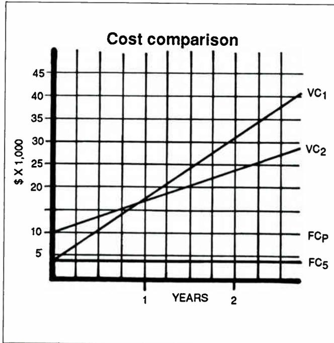
the extra cost of the new connector is covered and a net savings is realized in the 20,000 subscriber model system.
