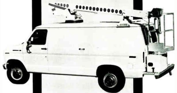
A-28 van mounted lift with APU. Utility-body mounted lift also available.
