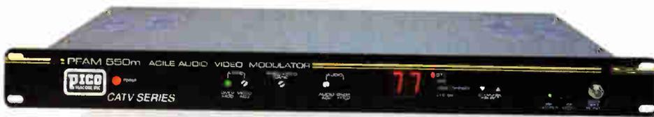
The PFAM 550m is a microprocessor controlled rebroadcast quality, phase locked loop synthesized, frequency agile CATV television modulator. The double conversion and superior SAW filtering provide adjacent channel compatibility and spurious free output.
