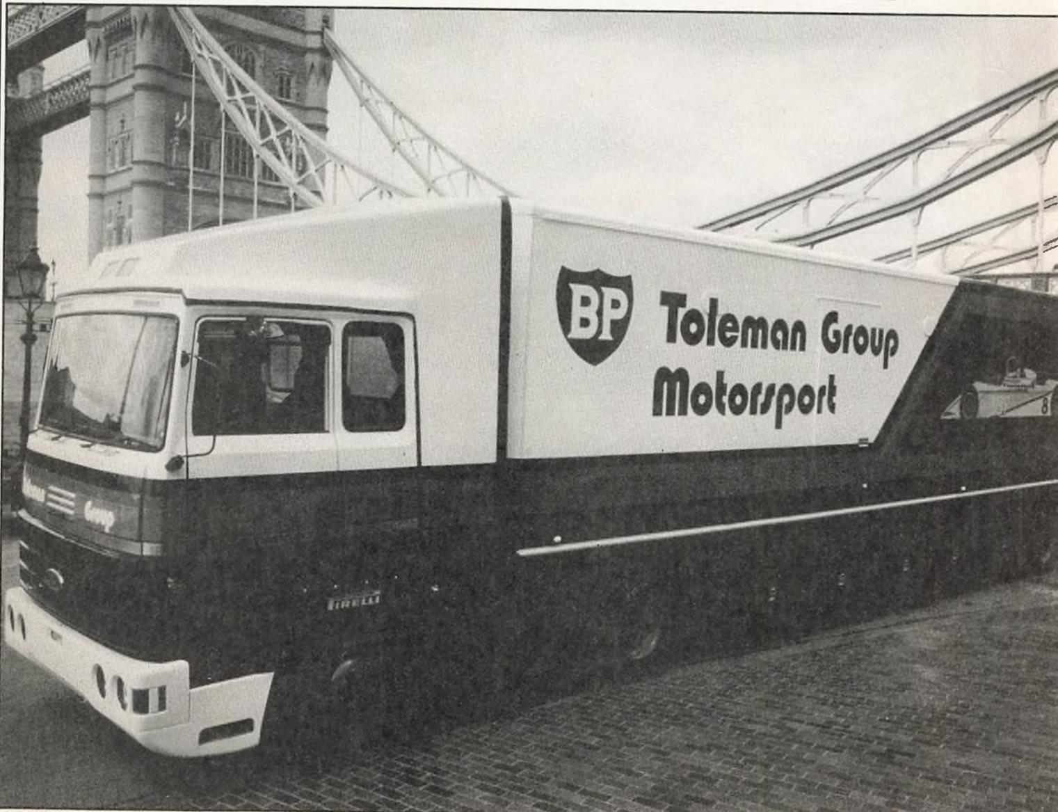
This is still more aerodynamics applied to a tractor unit. It begins with the simple things — flush wipers, flush step (lowering in response to the insertion of the key-card), wraparound screen with internal pillars, low profile tyres, airscoops for front and rear brakes and engine and a roof-mounted intake for factory air. Also, perhaps the major step, is the British Rail-type concertina between tractor and trailer. Boy Scouts will also observe the flush-mounted CB antenna. Ho hum.
