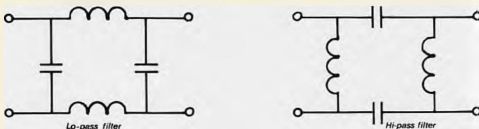
Fig. 4. Showing two basic types of filters. Note from the text that the capacitors will offer less and less reactance as the frequency is increased, while the coils act just the opposite.
