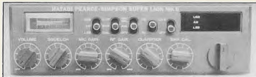
crophone gain, RF gain, Clarifier, SWR calibrate knob and finally the channel selector. Not much to be said about the volume control — however the squelch is a different story. The squelch action is smooth to open and has a long hysteresis (once open it takes a while to close after the signal is removed) and we found it a bit tricky to adjust the threshold.
