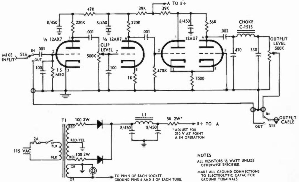
Now mount all controls and wire in all remaining components, following the schematic diagram and photographs. Use shielded wire for all audio leads (to grid or plate of any tube, as well as input and output) and try to keep these leads well away from the filament wiring.
