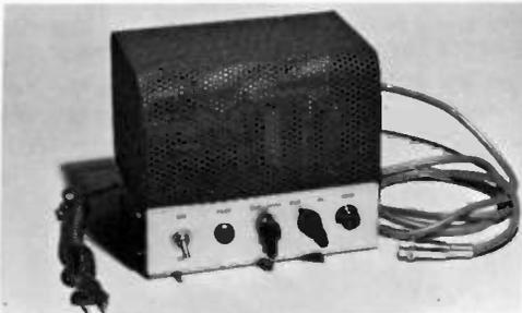
When the wiring is finished, the unit should be checked out before hooking it to your transmitter. One way of doing this is to connect a pair of head-
