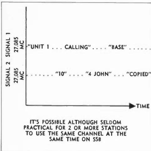
In other words, on sideband it is conceivable (although seldom practical) for two or more conversations to be going on at once on a channel. It is the beat note of two or more AM carriers trying to be at the same spot at once that covers up the audio intelligence on an AM signal . . . not the audio intelligence of one covering up the audio intelligence of the other.
