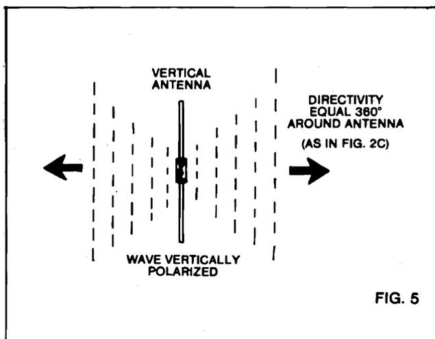
Fig. 5: A vertical antenna radiates waves that are vertically polarised.
