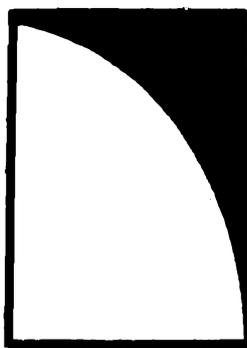
Power wave of full length non-loaded antenna
