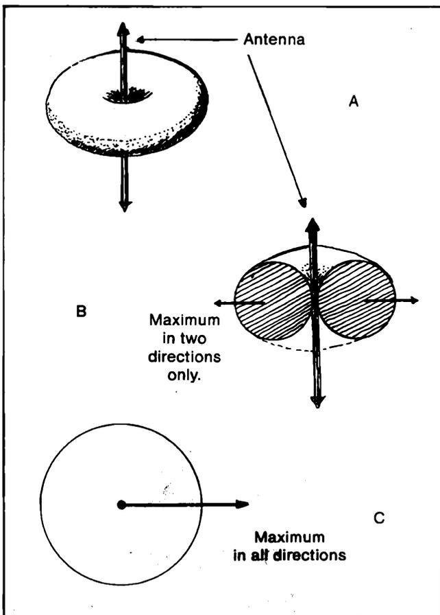
Fig. 2: (a) Solid configuration of radiation from a half-wave (dipole) antenna. (b) Radiation pattern when antenna is horizontal (see also fig. 3). (c) Radiation pattern (omnidirectional) when antenna is vertical.
