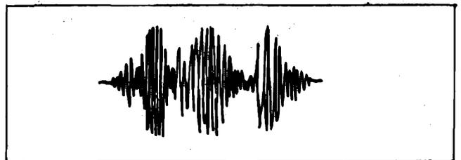
FIG 1. Typical Speech Waveform. Note the high amplitude of the peaks relative to the 'average' level.
