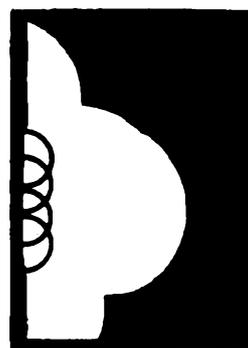
Power wave of center loaded or lump wound antenna
