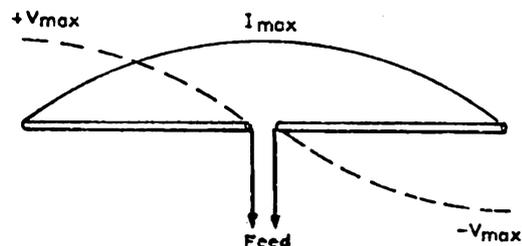
Fig. 1: Current and voltage distribution on a half-wave dipole antenna.
