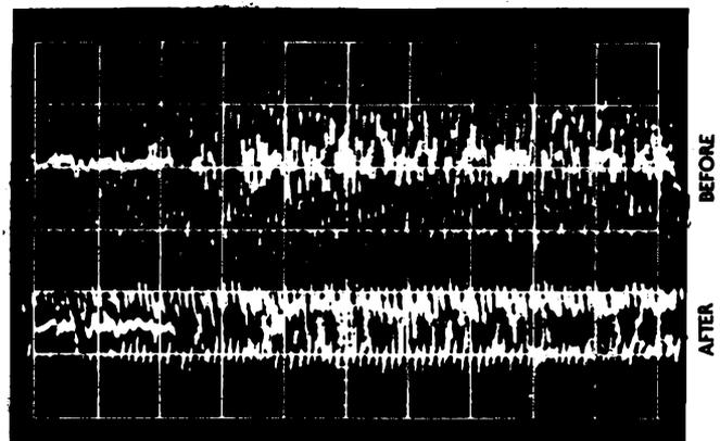
FIG 2. The word 'Hello' before and after passing through a speech processor. Note the peaks have been removed even though the average level has been increased.
