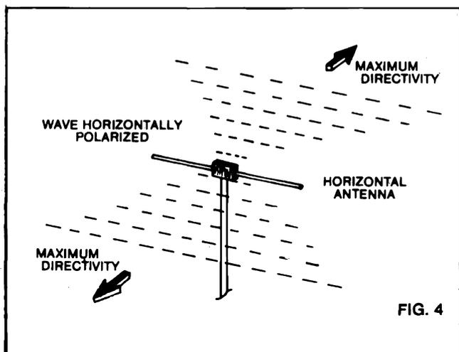
Fig. 4: A horizontal antenna radiates waves which are polarised in the same plane as the antenna itself i.e. the wave is horizontally polarised.
