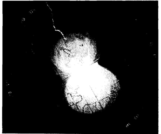
Fig. 3: Actual radiation pattern from a half-wave antenna in horizontal mode. Taken from a polar pattern display unit and shows how intensity of radiation diminishes with distance.
