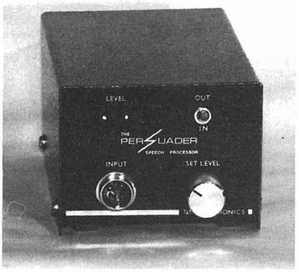
By removing power wasting peaks from the speech waveform and unwanted frequencies the average 'talk power' can be increased by up to THIRTY TWO times, i.e. a ten watt transmitter using the 'PERSUADER' will provide average 'talk power' equal to a 320 Watt transmitter with normal modulation.
