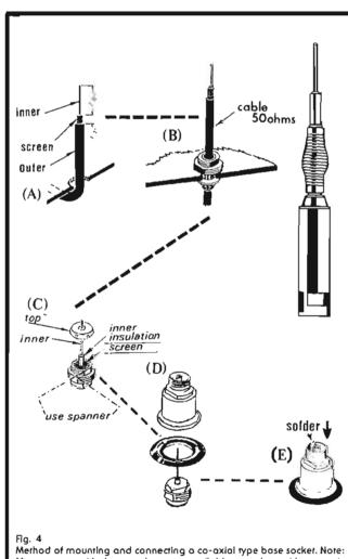
Mag mounts with these sockets are available complete with approximotely 5 metres of 50 ohm co-axial cable.
