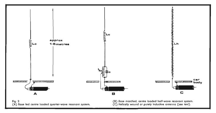
high resistive loss unless a very high 'Q' coil is used. Most of the mobile antennas at present on the market employ one or the other of these designs and all that can be done to keep the efficiency as high as possible is the use of high 'Q' loading coils and good quality insulating materials.
